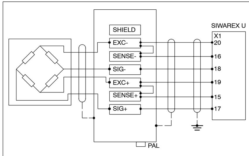
Figure 2-5 Connection of load cells using the 4-wire technique (example: connection to channel 2)
