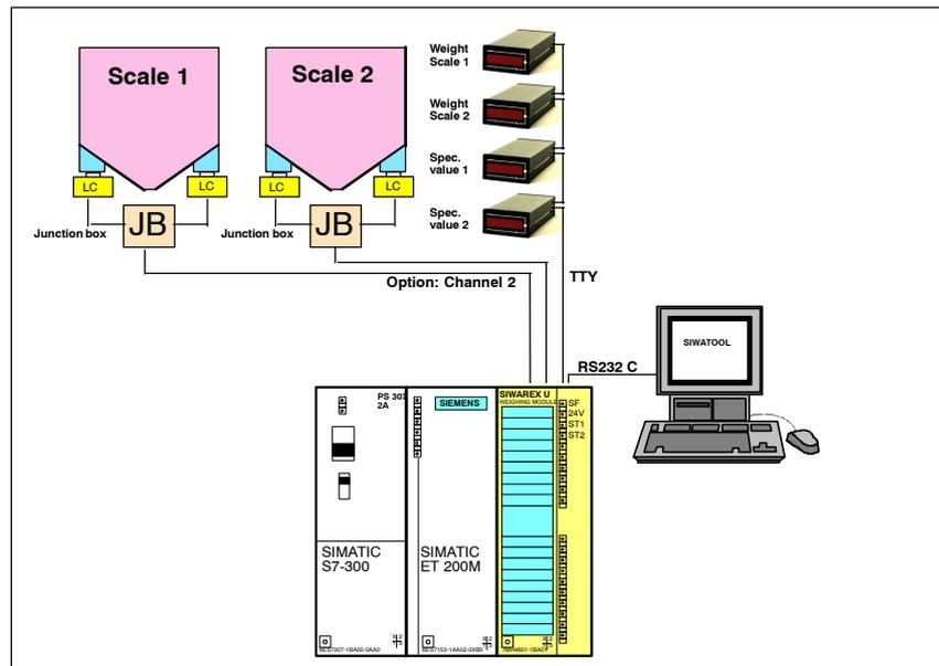
Figure 1-5 The SIWAREX U as a controller-independent field device
