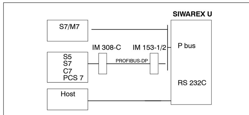
Figure 4-1 Possible links to a host system
