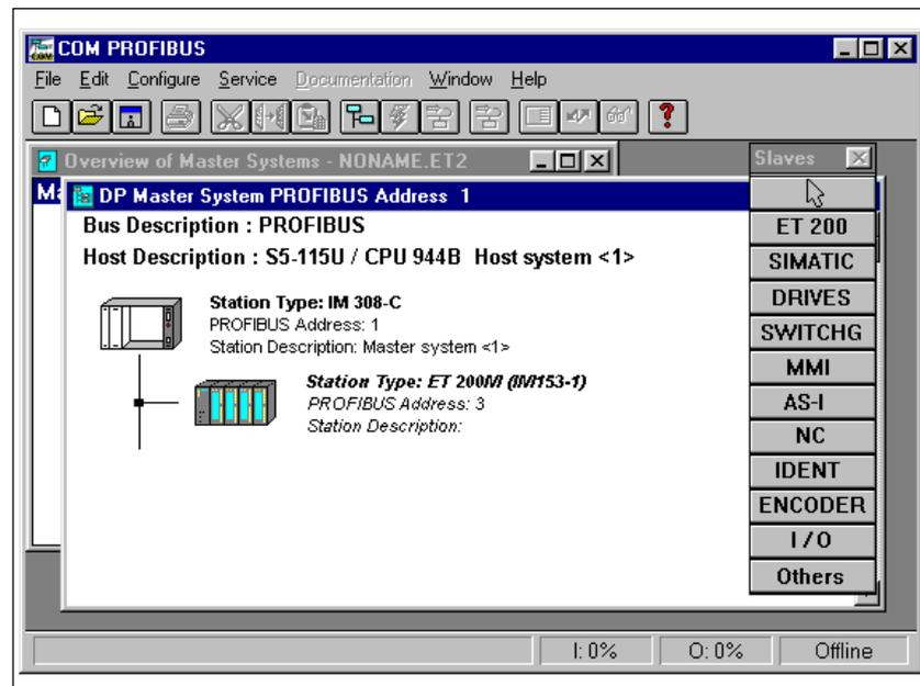
Figure 6-2 Parameter assignment with COM PROFIBUS
