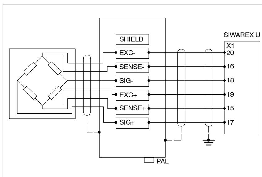
Figure 2-4 Connection of load cells using the 6-wire technique (example: connection to channel 1)
