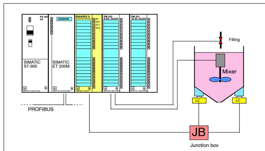
Figure 1-8 SIWAREX U fill level scales
