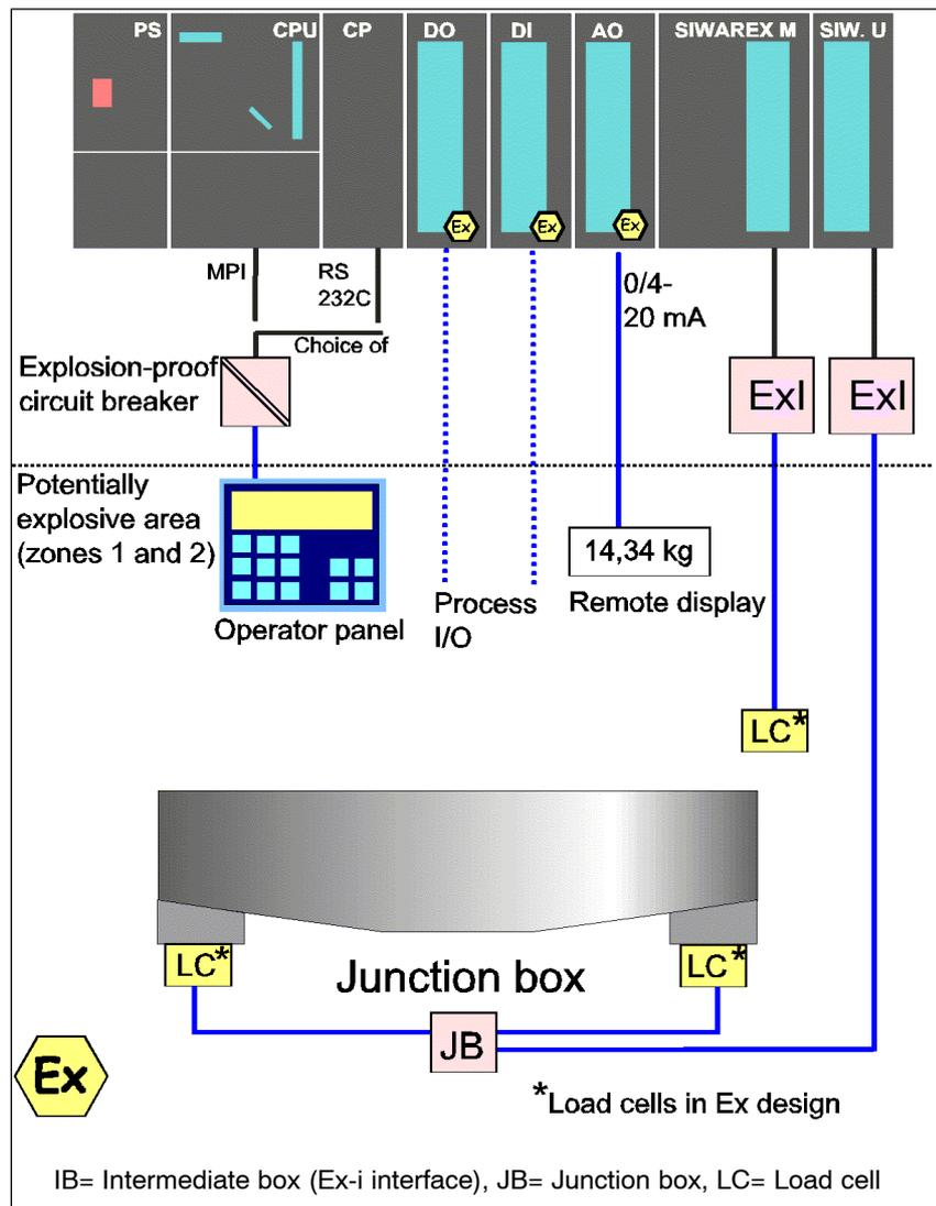
Figure 1-9 Scales for potentially explosive area
