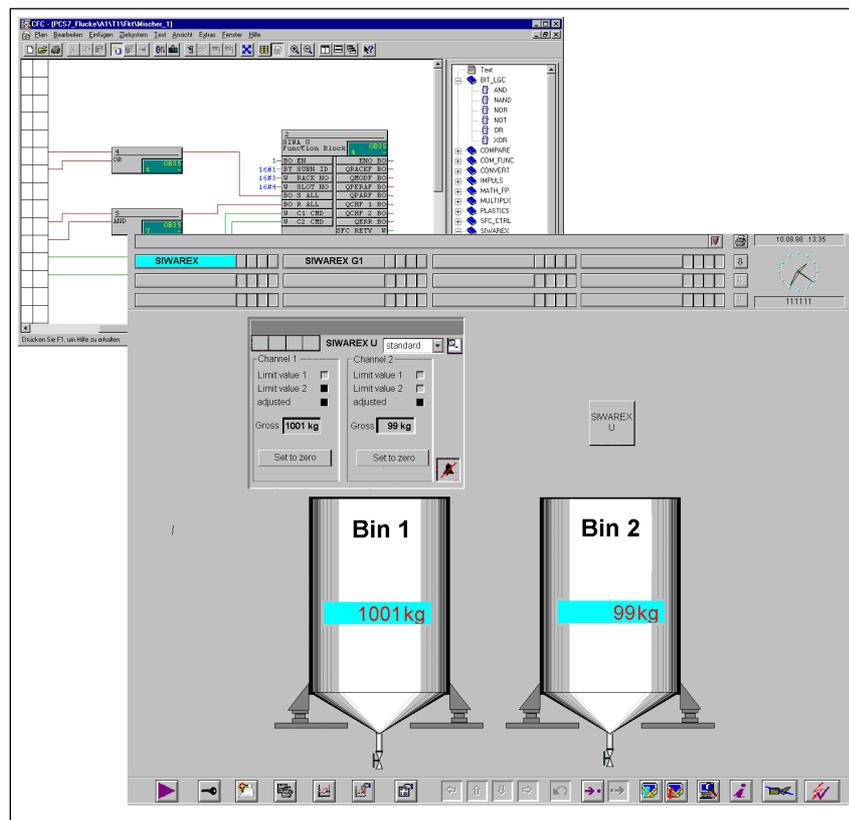
Figure 1-4 Representation of the SIWAREX U in the ES engineering system (left) and on the OS operator station (right)
