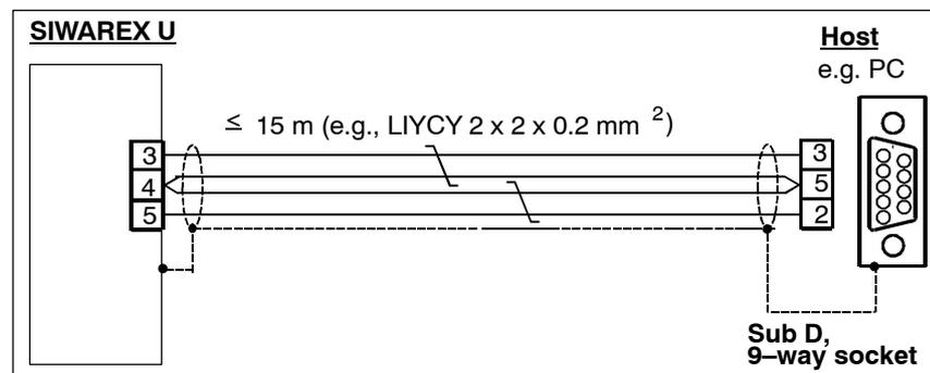
Figure 2-6 Connection of a PC to the RS 232 interface
