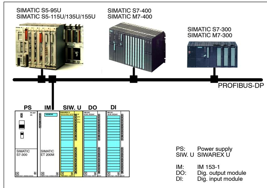
Figure 1-3 The SIWAREX U as distributed periphery in the SIMATIC S5/S7/M7
