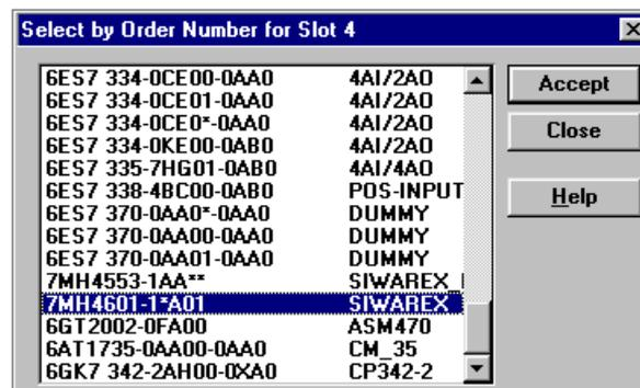
Figure 6-1 Selection of SIWAREX U module during configuration of the ET 200M
