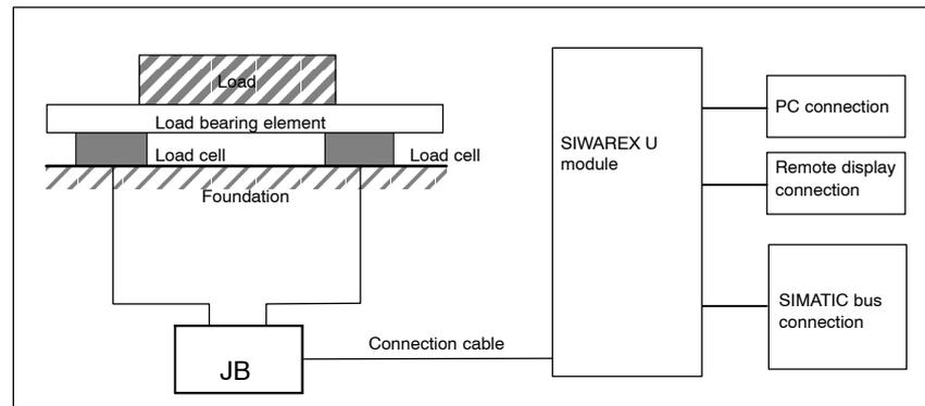
Figure 1-7 Setup of the weighing system with a SIWAREX U
