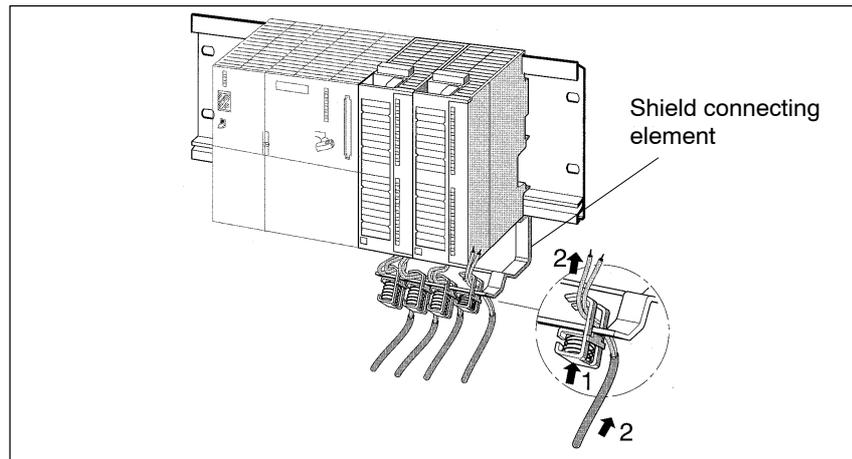
Figure 2-1 Shield connecting element
