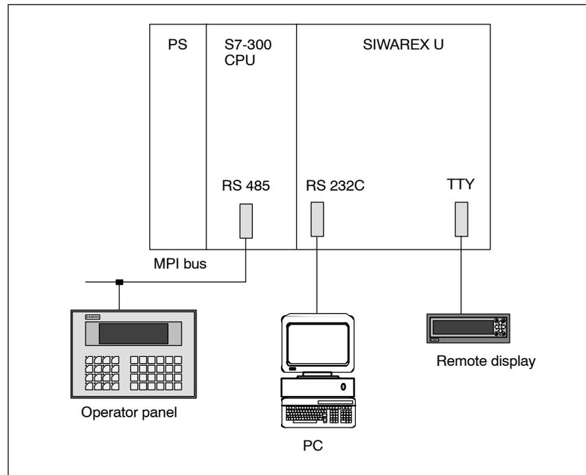
Figure 10-1 Connection of optional components
