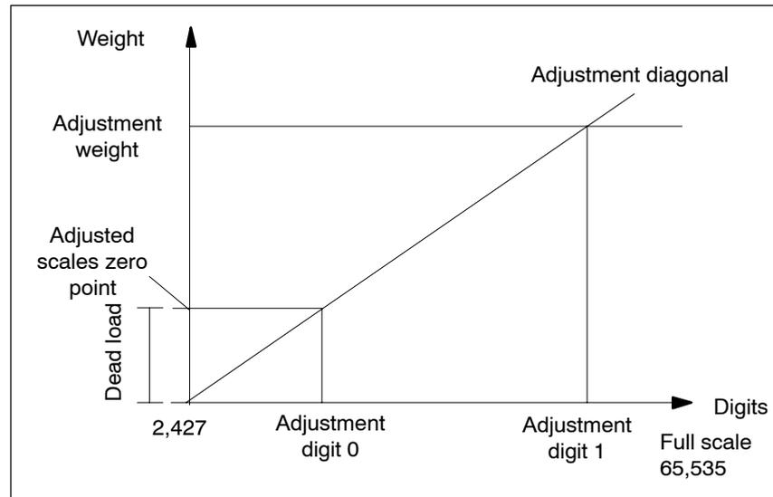
Figure 3-2 Adjustment procedure
