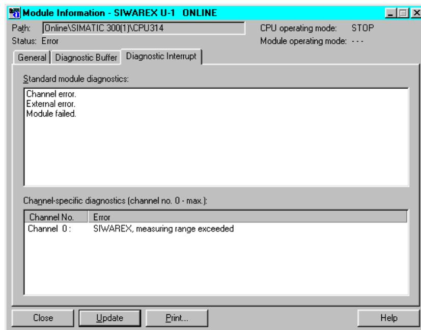
Figure 5-2 Module status in STEP 7
