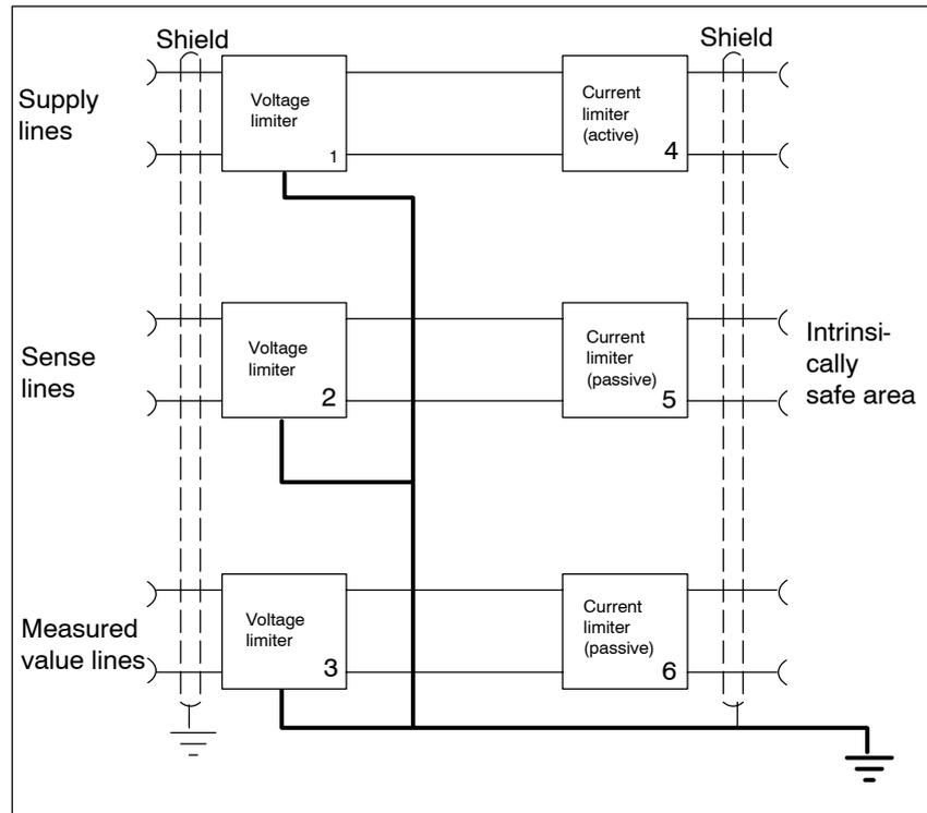
Figure 10-4 Diagram of the Ex-i interface
