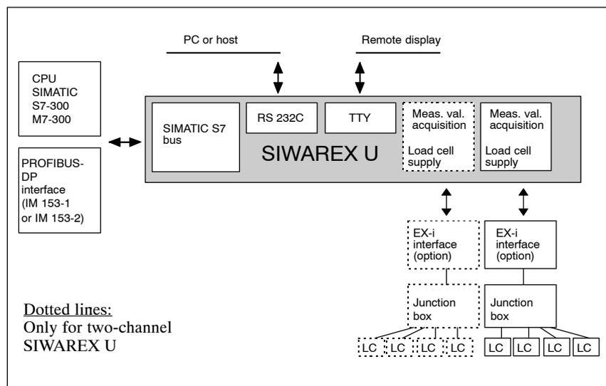
Figure 1-6 Diagram of the SIWAREX U setup
