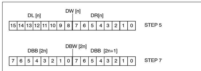
Figure 9-1 Comparison of data addressing with STEP 5 and STEP 7
