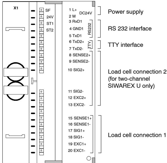
Figure 2-3 Connection elements on the front of the SIWAREX U
