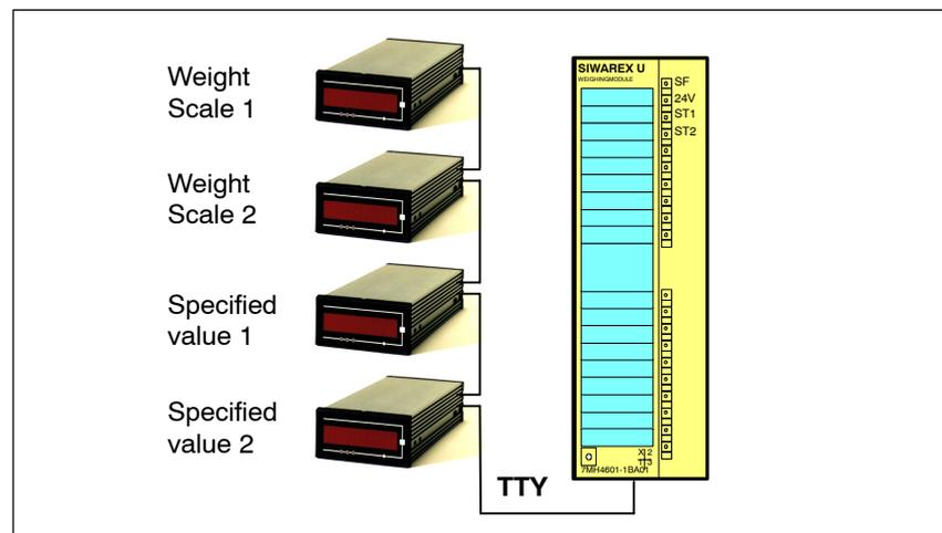
Figure 10-2 Example: Connection of 4 digital remote displays to the SIWAREX U
