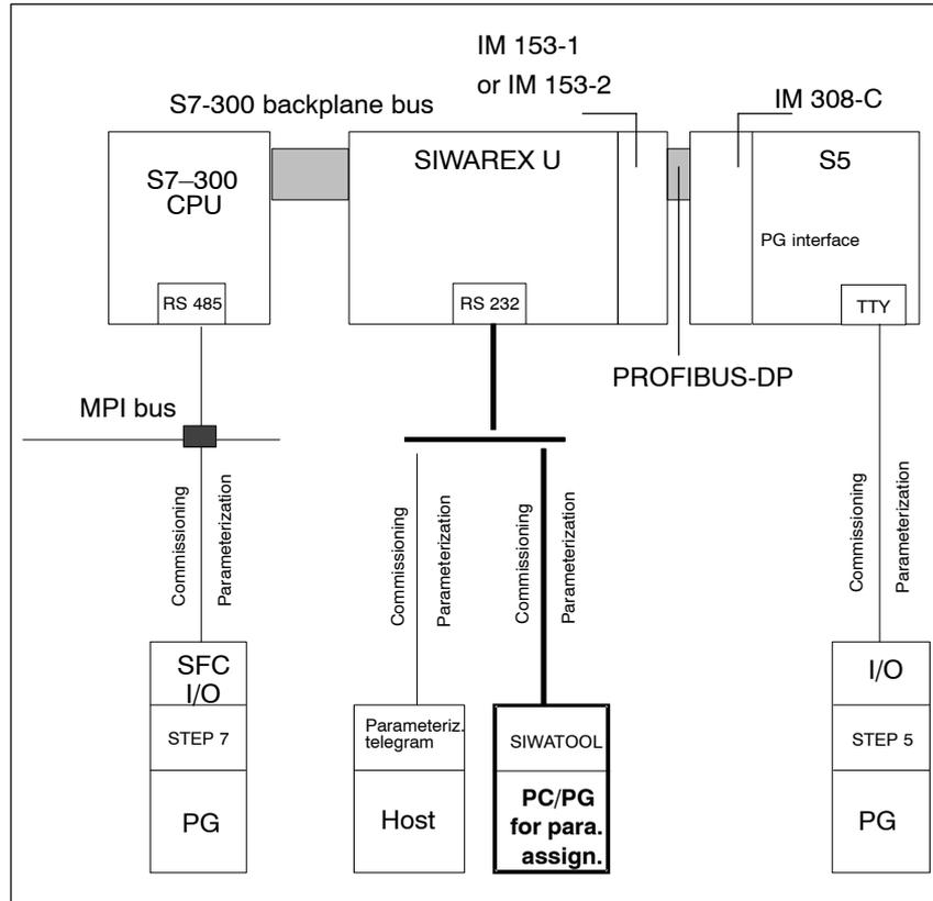
Figure 2-9 Methods of parameter assignment for various system configurations
