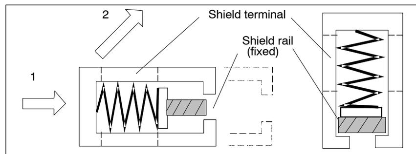
Figure 2-2 Mounting the shield terminals
