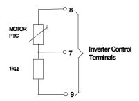
Figure 2.2.5: Motor Overload PTC Connection
