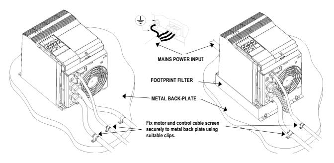
Figure 1.2.3: Wiring guidelines to minimise effects of EMI - MICROMASTER FSC
