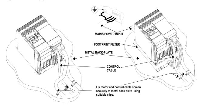
Figure 1.2.2: Wiring guidelines to minimise effects of EMI - MICROMASTER FSB
