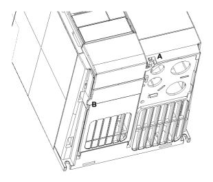
Insert the blade of a small screwdriver into slot A in the front of the inverter and press in the direction of the arrow. At the same time, press down on tab B at the side of the access panel.
