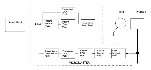
MICROMASTER Closed loop PI control - Block Diagram
