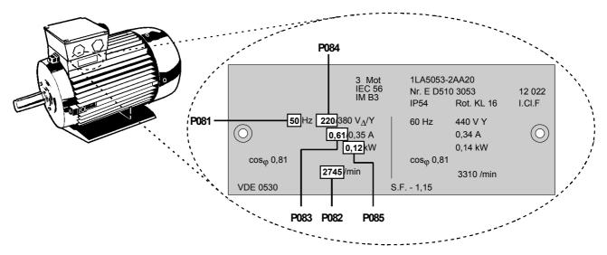
Figure 3.2.1: Typical Motor Rating Plate Example
