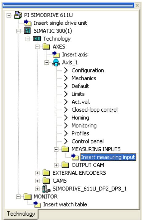
Figure 4-35 Inserting a measuring input
