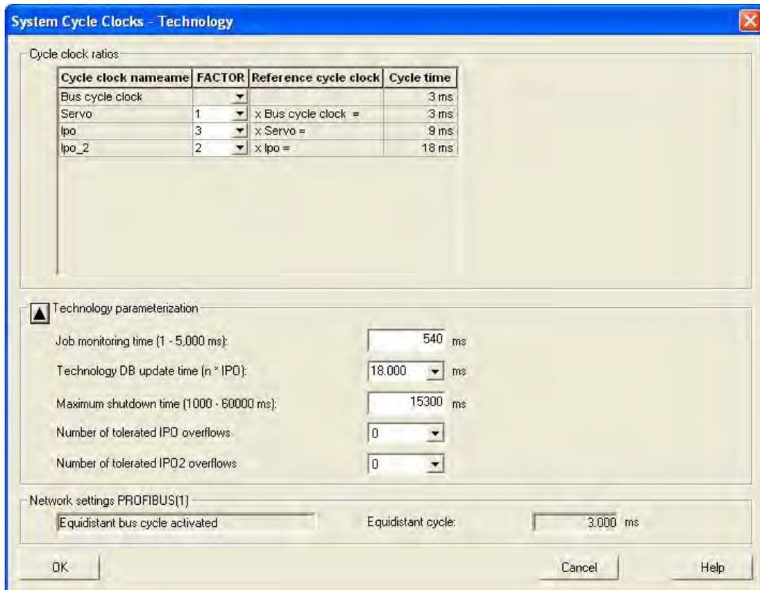
Figure 4-27 Set system clock cycles
