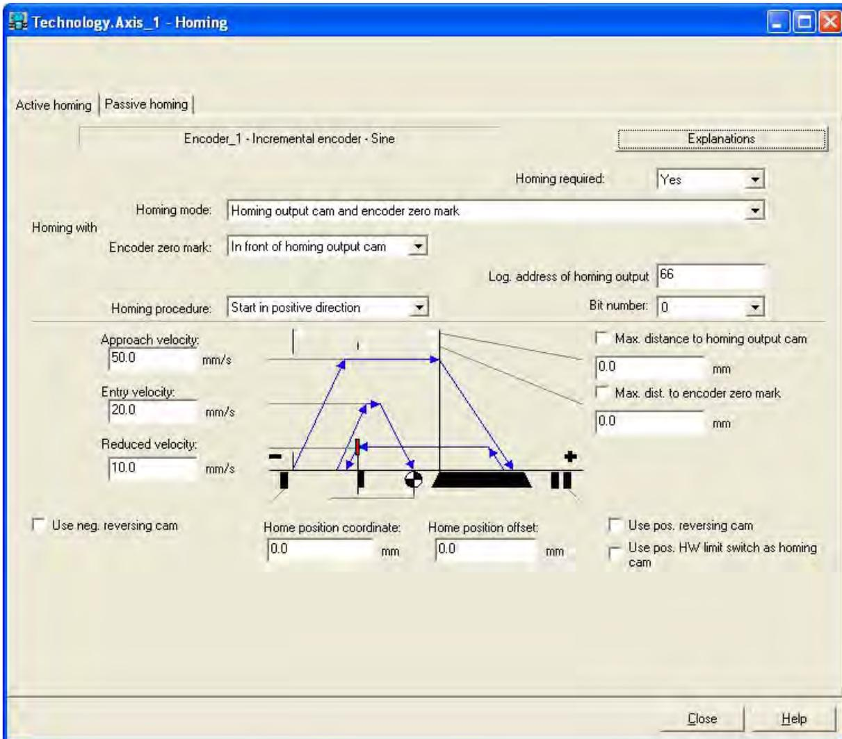
Figure 4-32 Axis homing in STEP 7 (homing cam homing mode and encoder zero mark)
