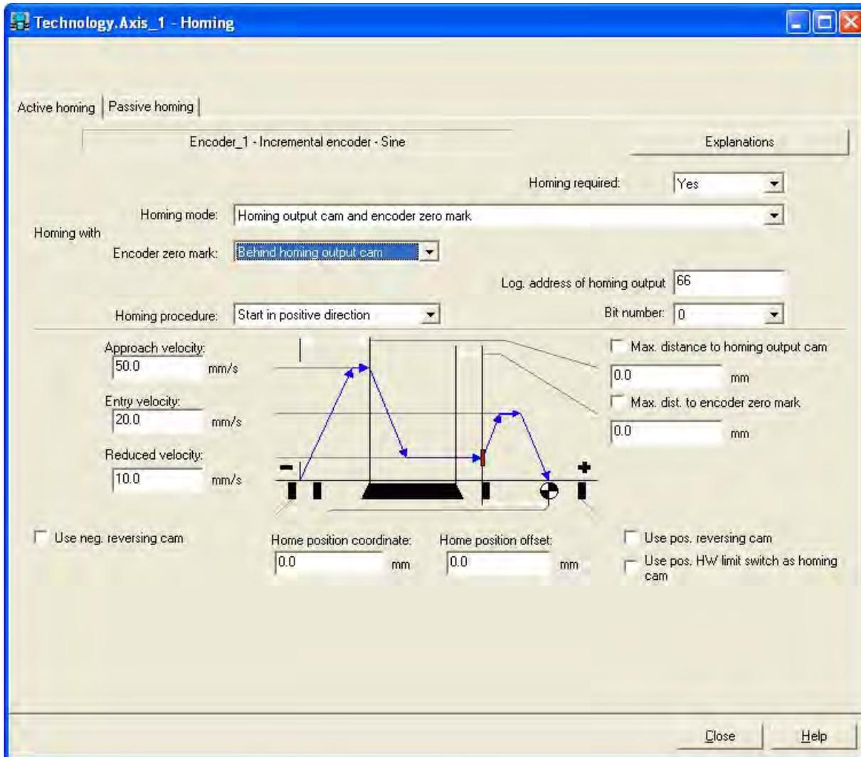
Figure 4-33 Axis homing in STEP 7 (homing cam homing mode and encoder zero mark)
