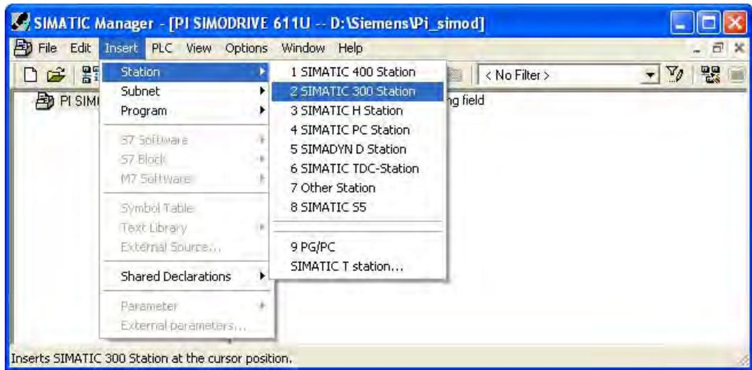
Figure 4-2 Inserting a SIMATIC station 300
