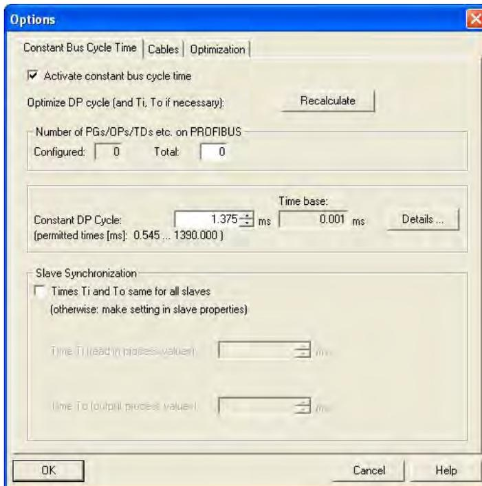
Figure 4-7 Activate isochronous bus cycle
