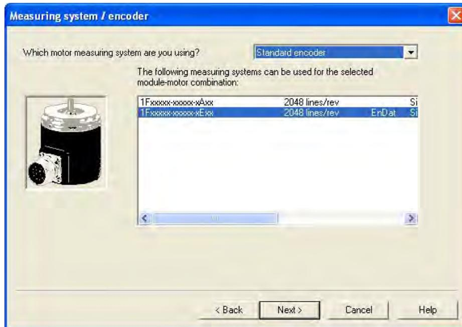
Figure 4-47 Measuring system/encoder window
