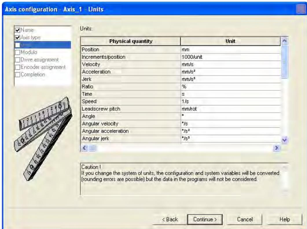
Figure 4-17 3rd window of the axis configuration
