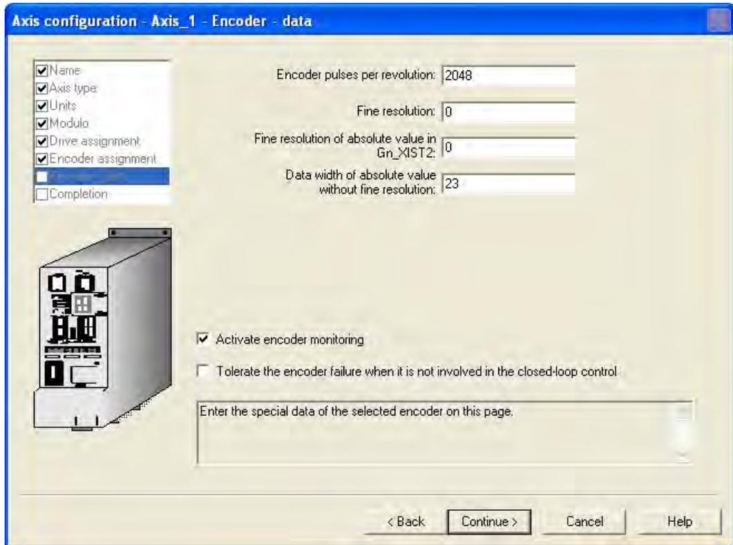
Figure 4-21 Axis configuration in S7T Config (enters the resolution of the absolute encoder)
