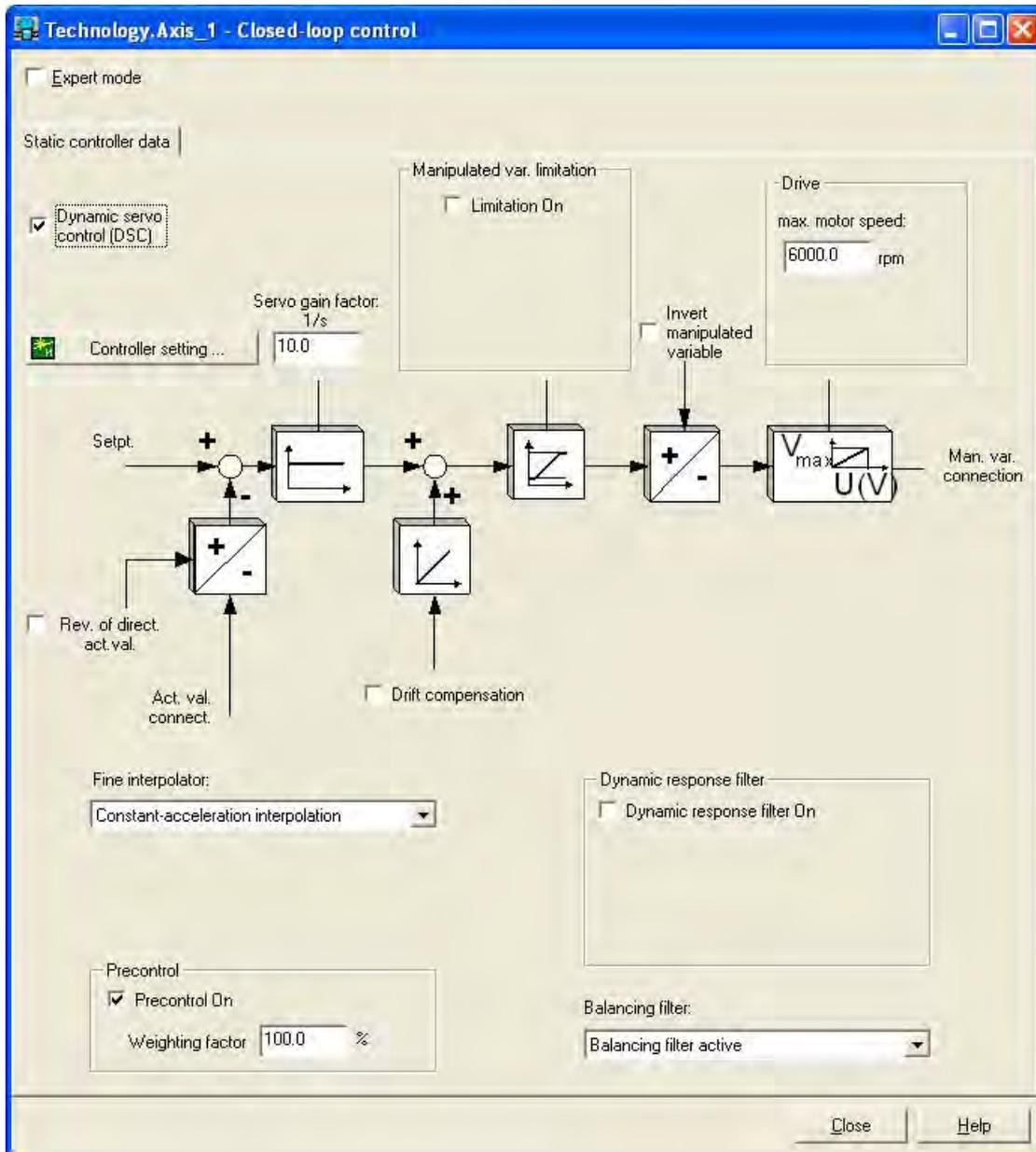
Figure 4-26 Position controller configuration
