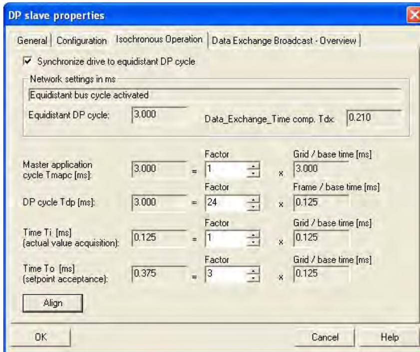
Figure 4-11 Activate clock-synchronized operation
