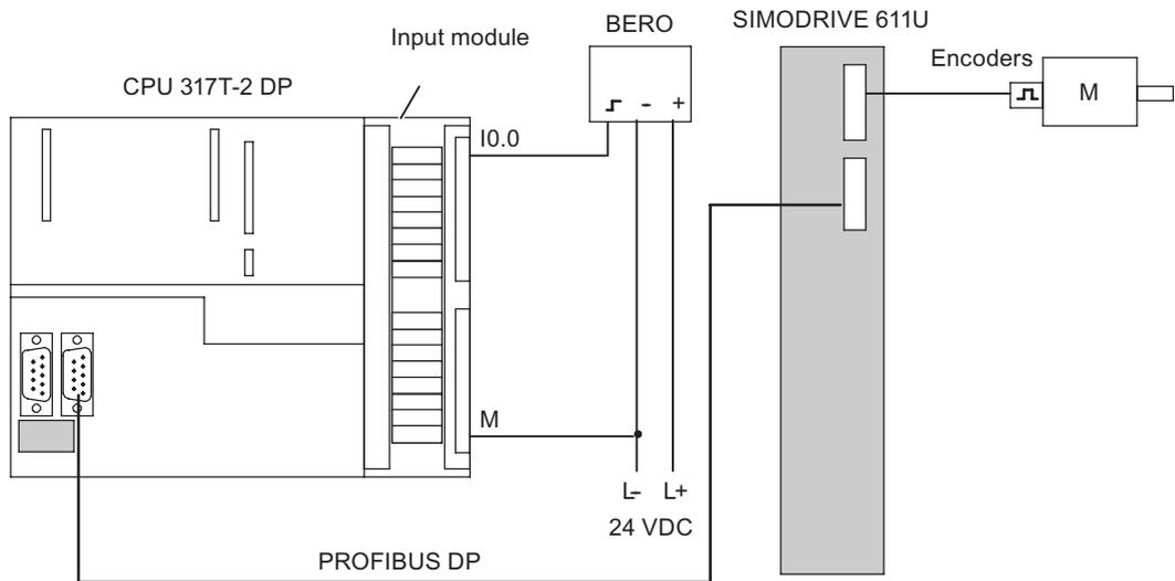
Figure 4-31 Homing (Homing output cam and encoder zero mark)
