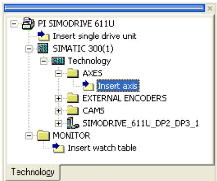
Figure 4-14 Inserting an axis
