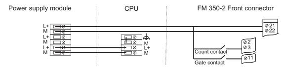
Plug the front connector into the FM 350-2 and screw-tighten it.
