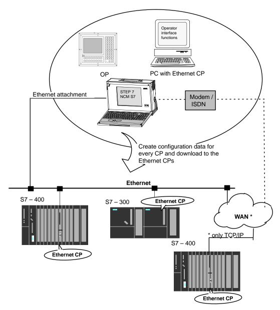
Figure 1-2 Configuration for PG/OP Operation
