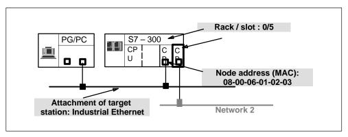
Figure 7-2 The CP requiring diagnostics is accessible indirectly over another CP
