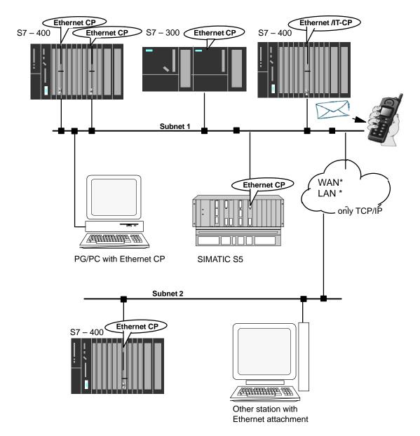
Figure 4-1 Possible Connections
