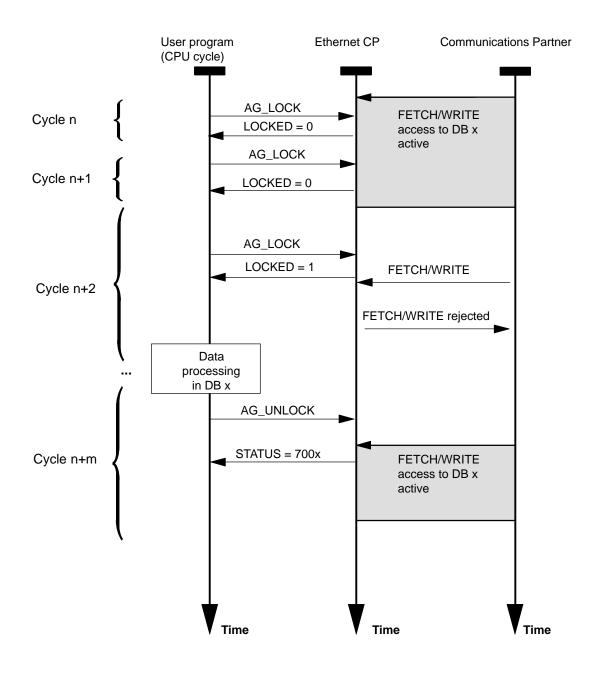
The lock job must first be monitored in the user program using the code in the return parameter LOCKED. As long as LOCKED=0 is indicated, it must be assumed that there is still a FETCH/WRITE access active.
