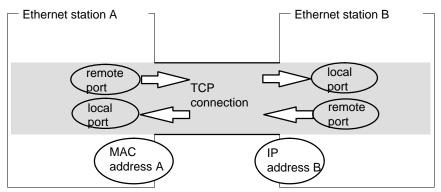
Figure 4-15 Sending and Receiving on One TCP Connection
