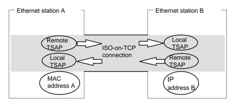
Figure 4-11 Sending and Receiving on One ISO-on-TCP Connection
