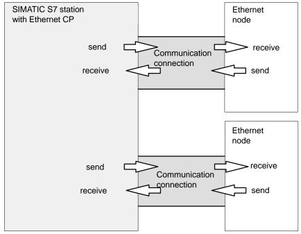
Figure 4-2 Sending and Receiving via one Communication Connection
