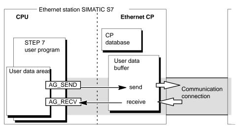
Figure 3-1 Interaction of the CPU and Ethernet CP on Connections
