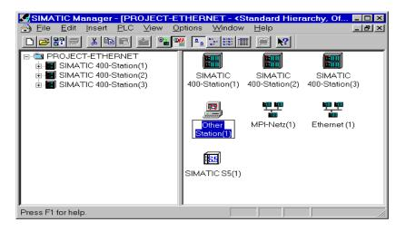
Figure 2-5 Project With Substitute Objects Configured
