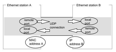
Figure 4-19 Sending and Receiving on One UDP Connection
