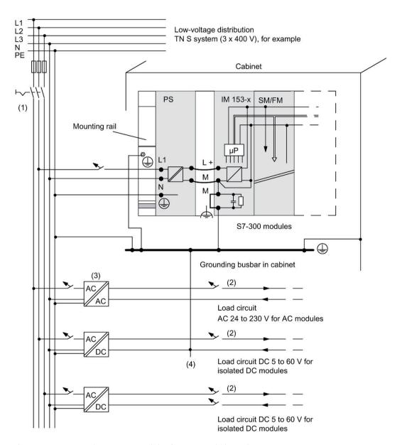
Figure 3-10 Operating S7-300 modules from grounded supply
