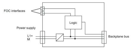
Figure 10-3 Block diagram of the IM 153-2 FO
