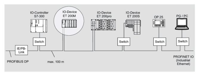
Figure 1-2 Typical structure of a PROFINET IO network
