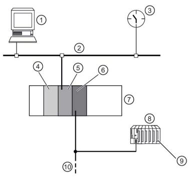
Figure 8-11 Sample configuration: Communication processor as DP master and DP clock master
