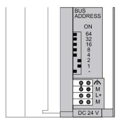
Figure 2-2 Setting PROFIBUS address 3
