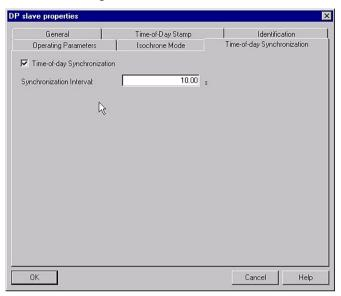
Figure 8-19 Dialog box DP slave properties > Time-of-day Synchronization
