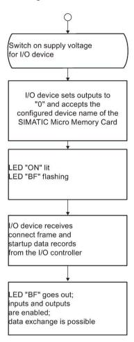
Figure 6-5 Startup of ET 200M on PROFINET IO
