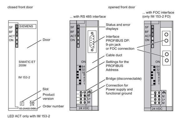
Figure 1-4 Front view of the interface modules IM 153-1 and IM 153-2AA02 / -2AB01
