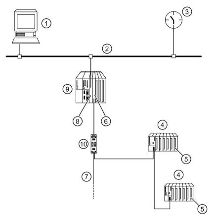
Figure 8-1 Example structure for time stamping signal changes with IM 153-2
