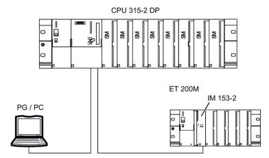
Figure 7-5 Update via PROFIBUS DP (PD / PC via CPU to the IM 153-2)
