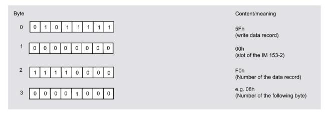
Figure 8-14 Head data of the telegram with the data record 240 for the configuration
