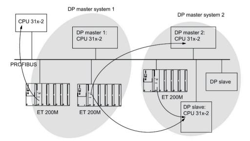
Figure 8-24 Direct data exchange with the IM 153-x
