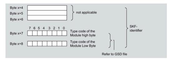
Figure 9-18 Structure as of byte x+4 for removing / inserting interrupt
