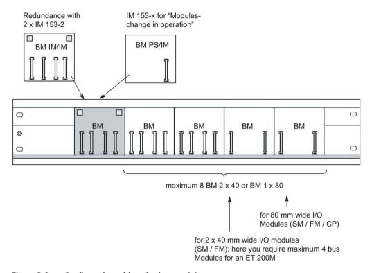
Figure 3-9 Configuration with active bus modules
