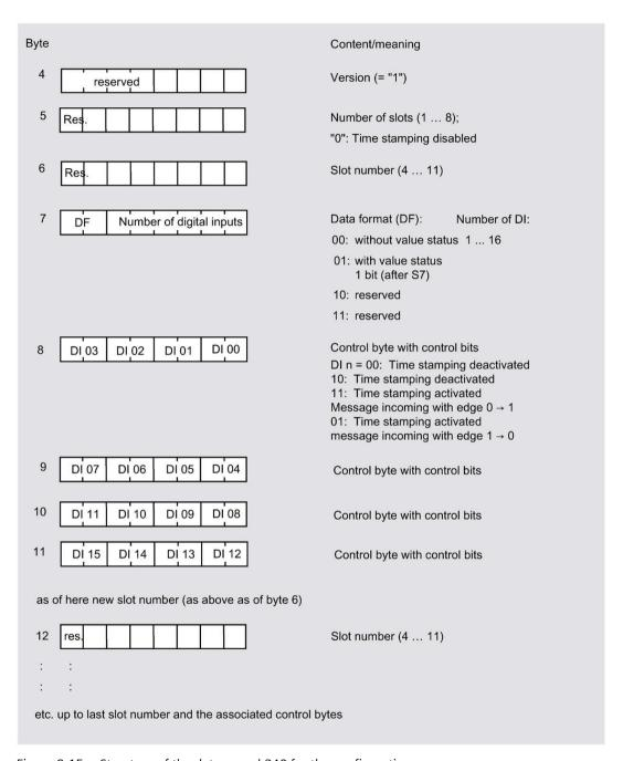
Figure 8-15 Structure of the data record 240 for the configuration
