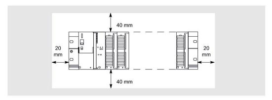
Figure 3-6 Clearance measurements for an ET 200M installation on a mounting rack
