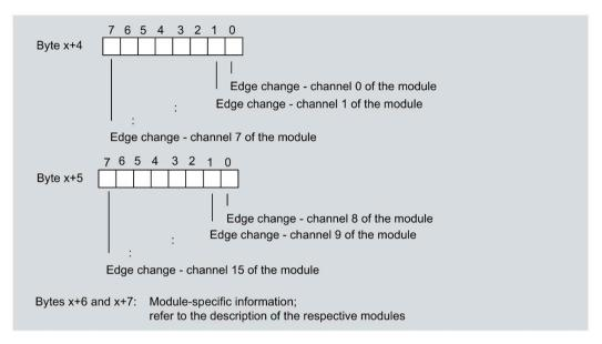
Figure 9-17 Structure as of byte x+4 for hardware interrupt (digital inputs)
