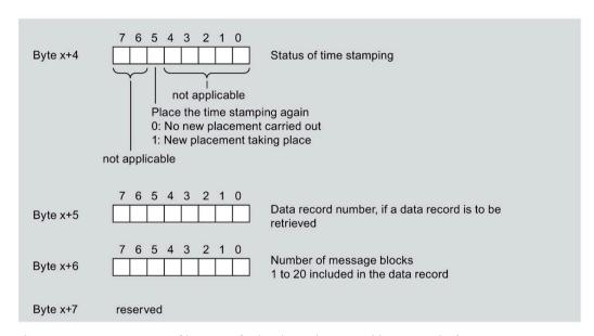
Figure 9-15 Structure as of byte x+4 for hardware interrupt (time stamping)
