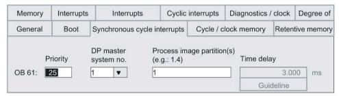
Figure 8-21 Synchronous cycle interrupts dialog box
