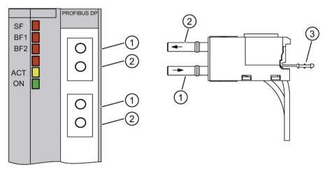
Figure 5-1 Connect the FOC to the IM 153-2 FO
