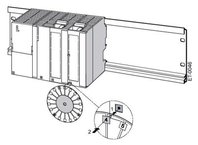
Figure 4-3 Attach the slot numbers to the modules.
