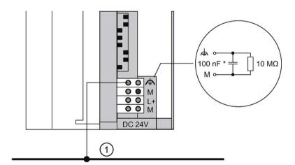
Figure 3-12 Configuration of an ET 200M with ungrounded reference potential
