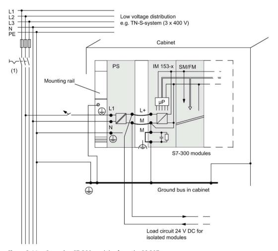
Figure 3-11 Operating S7-300 modules from the PS 307
