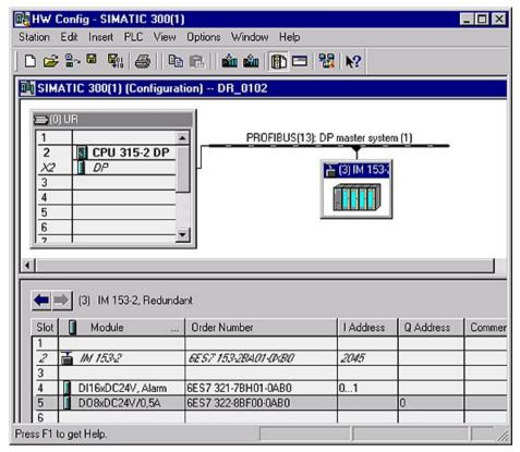
Figure 2-4 Configuration table for ET 200M
