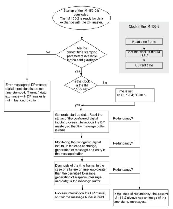
Figure 6-4 Start-up for time synchronization / time stamping
