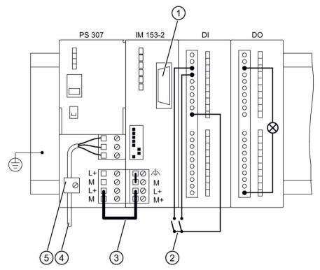
Figure 2-3 Wiring of the ET 200M
