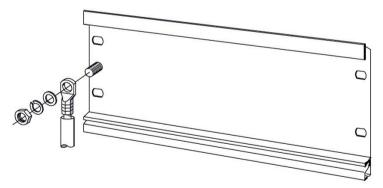
Figure 4-2 Connecting the protective conductor to the rail
