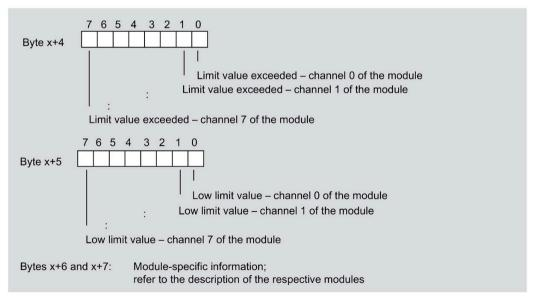
Figure 9-16 Structure as of byte x+4 for hardware interrupt (analog inputs)
