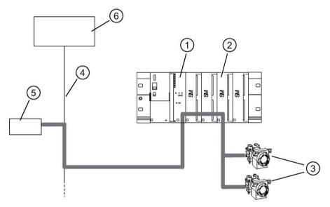
Figure 3-2 Passing on parameter assignment data with an IM 153-2 and HART modules
