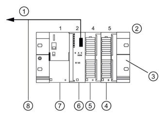
Figure 2-1 ET 200M components for the example configuration
