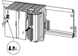
Figure 5-3 Bringing the front connector into the wiring position
