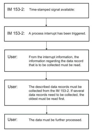
Figure 8-13 Processing time-stamped signals
