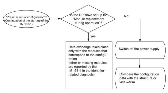
Figure 6-2 Startup behavior in the case of module change during operation
