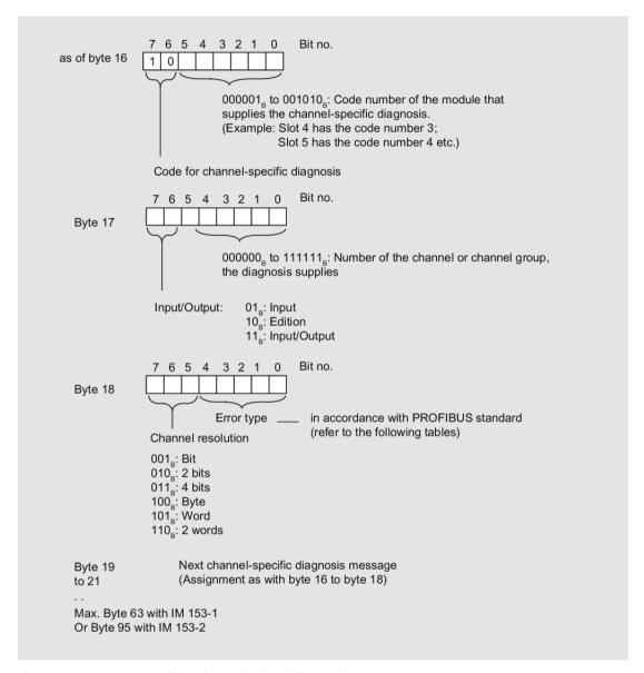
Figure 9-6 Structure of the channel-related diagnostics
