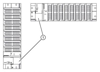
Figure 3-5 Horizontal and vertical installation of an ET 200M
