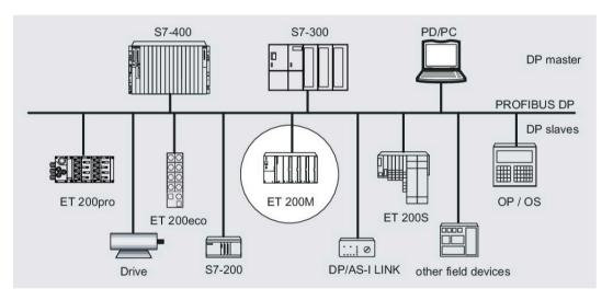
Figure 1-1 Typical structure of a PROFIBUS DP network
