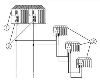
Figure 8-20 Redundancy with 2 x IM 153-2 in an H system
