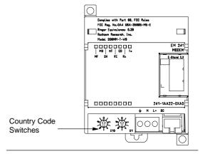
Figure 10-1 EM 241 Modem Module
