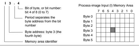
Figure 4-4 Byte.Bit Addressing
