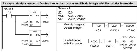
Note: VD100 contains: VW100 and VW102, and VD200 contains: VW200 and VW202.
