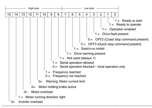
Figure 11-4 Status Bits for Standard Status Word for MicroMaster 4 and Main Feedback
