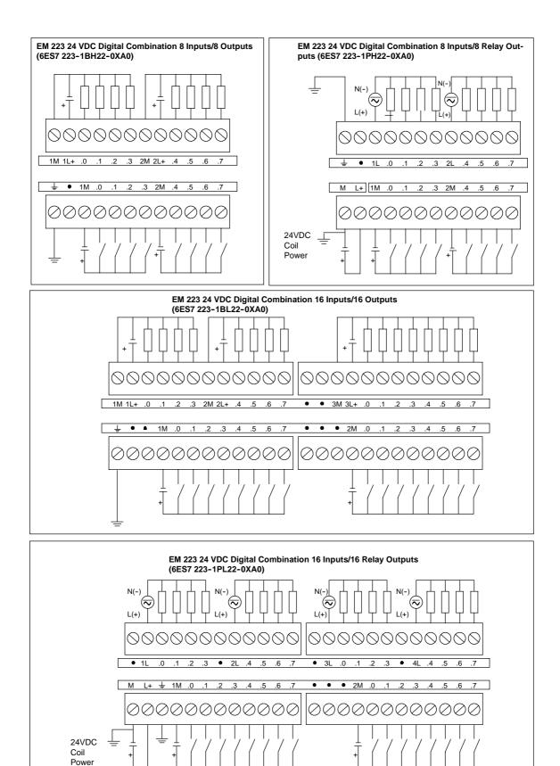
Figure A-11 Wiring Diagrams for EM 223 Expansion Modules
