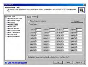
Figure 4-21 Analog Output Table
