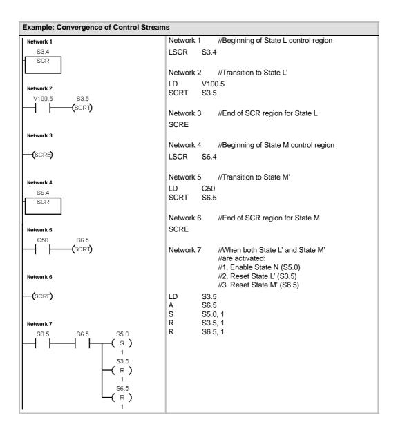
In other situations, a control stream might be directed into one of several possible control streams, depending upon which transition condition comes true first. Such a situation is depicted in Figure 6-34, which shows an equivalent SCR program.
