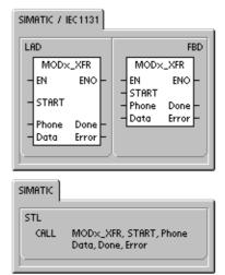
Done is a bit that comes on when the Modem module completes the data transfer.
