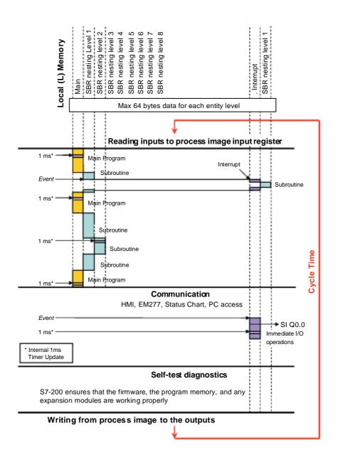
Figure 4-3 Typical Scan Flow
