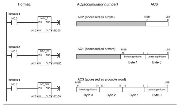
Figure 4-8 Accessing the Accumulators
