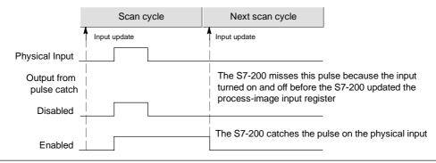
Figure 4-26 Operation of the S7-200 with the Pulse Catch Feature Enabled and Disabled
