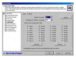
Figure 4-24 Analog Input Filter
