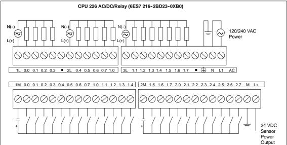
Figure A-6 CPU 226 Wiring Diagrams
