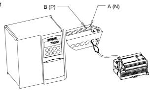
Figure 11-6 Connecting to the MM420 Terminal Block
