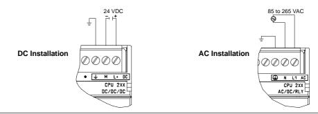
Figure 2-1 Connecting Power to the S7-200 CPU
