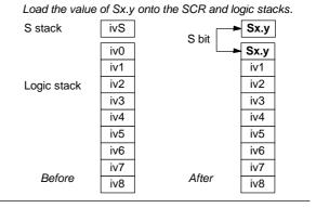
Figure 6-31 Effect of LSCR on the Logic Stack
