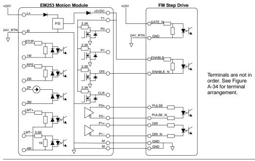
Figure A-36 Connecting an EM 253 Position Module to a SIMATIC FM Step Drive
