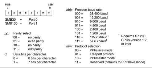
Figure 6-8 SM Control Byte for Freeport Mode (SMB30 or SMB130)
