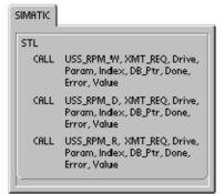
Param is the parameter number. Index is the index value of the parameter that is to be read. Value is the parameter value returned. The address of a 16-byte buffer must be supplied to the DB\_Ptr input. This buffer is used by the USS\_RPM\_x instruction to store the results of the command issued to the MicroMaster drive.
