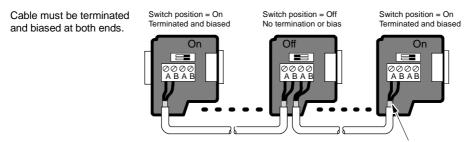
Bare shielding: approximately 12 mm (1/2 in.) must contact the metal guides of all locations.
