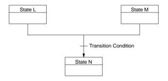
Figure 6-33 Convergence of a Control Stream
