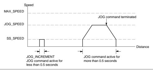
Figure 9-13 Representation of a JOG Operation
