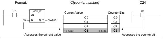
Figure 4-7 Accessing the Counter Bit or the Current Value of a Counter
