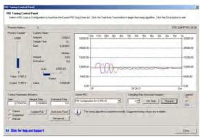
Figure 15-1 Auto-Tuning Sequence on a Direct Acting Loop
