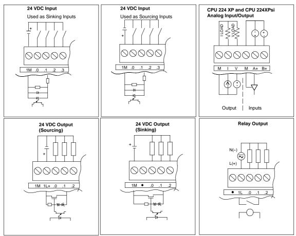
Figure A-2 CPU Inputs and Outputs
