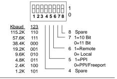
Figure 7-29 Settings for the RS-232/PPI Multi-Master Cable
