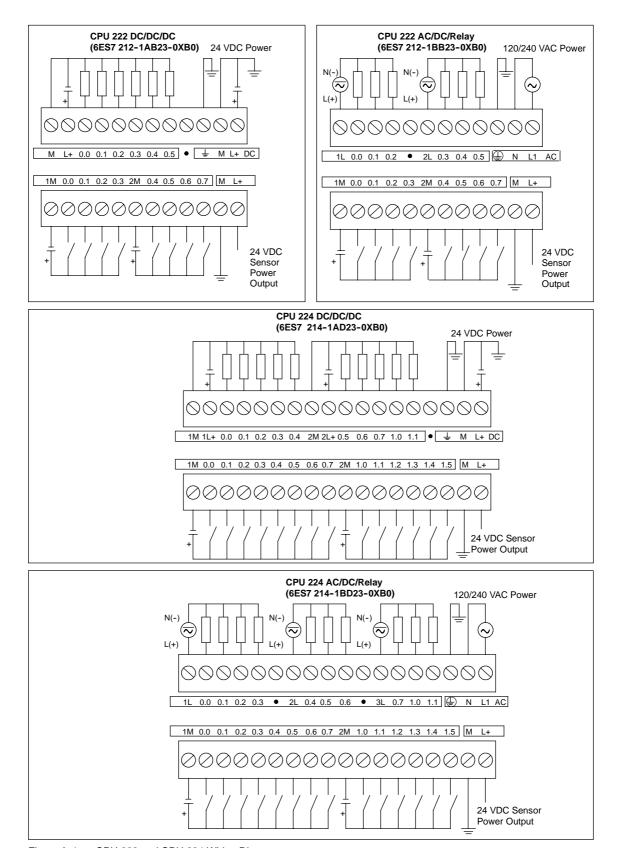
Figure A-4 CPU 222 and CPU 224 Wiring Diagrams
