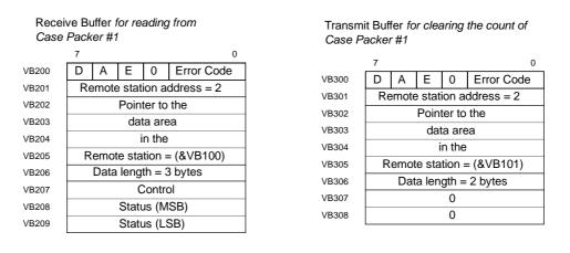
Figure 6-7 Sample TBL Data for the Network Read/Write Example
