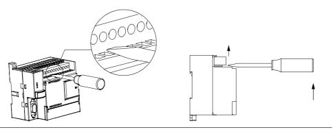
Figure 3-2 Removing the Connector
