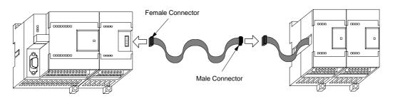
Figure A-43 Typical Installation of the I/O Expansion Cable
