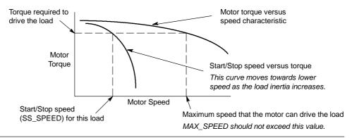
Figure 9-4 Typical Torque-Speed Curve for a Motor
