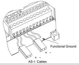
Figure A-42 Connecting the AS-Interface Module
