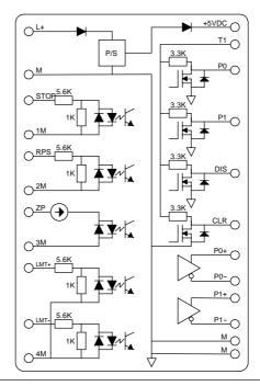
Figure A-35 Internal Schematic for the Inputs and Outputs of the EM 253 Position Module
