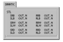
If the shift count is 0, a rotate operation is not performed. If the rotate operation is performed, the value of the last bit rotated is copied to the overflow bit (SM1.1).
