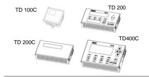
Figure 1-3 Text Display Units
