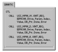
The address of a 16-byte buffer must be supplied to the DB\_Ptr input. This buffer is used by the USS\_WPM\_x instruction to store the results of the command issued to the MicroMaster drive.
