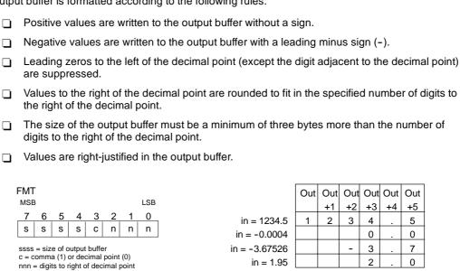
Figure 6-17 FMT Operand for the Real to ASCII (RTA) Instruction
