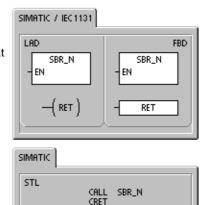
A subroutine call cannot be placed in any subroutine called from an interrupt routine. Recursion (a subroutine that calls itself) is not prohibited, but you should use caution when using recursion with subroutines.
