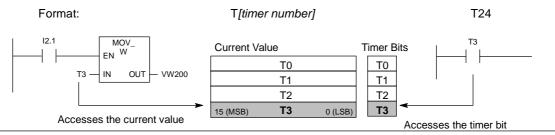
Figure 4-6 Accessing the Timer Bit or the Current Value of a Timer
