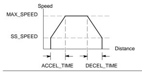
Figure 9-5 Acceleration and Deceleration Times
