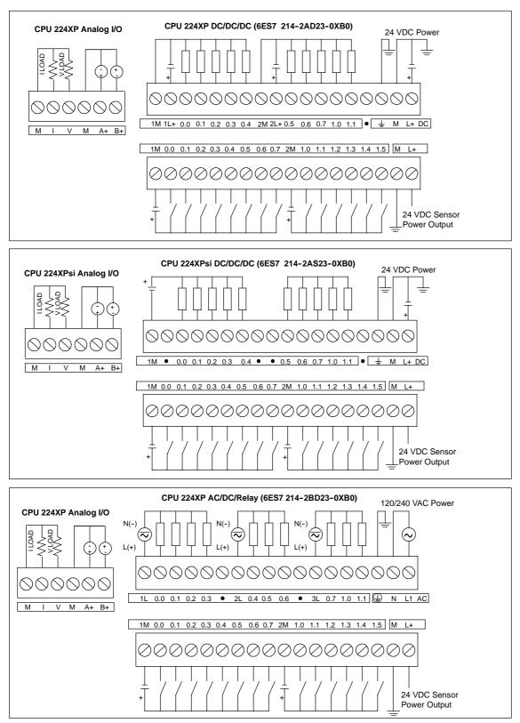
Figure A-5 CPU 224XP Wiring Diagrams
