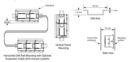
Figure 3-1 Mounting Methods, Orientation, and Clearance
