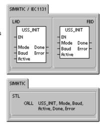
Baud sets the baud rate at 1200, 2400, 4800, 9600, 19200, 38400, 57600 or 115200. Baud rates 57600 and 115200 are supported by S7-200 CPUs version 1.2 or later.
