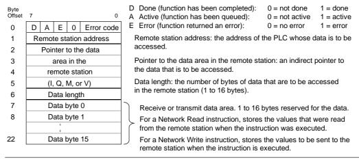
Figure 6-5 TBL Parameter for the Network Read and Network Write Instructions
