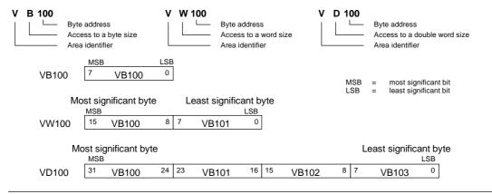
Figure 4-5 Comparing Byte, Word, and Double-Word Access to the Same Address
