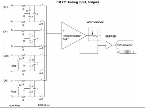
Figure A-18 Input Block Diagram for the EM231 Analog Input, 8 Inputs
