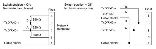
Figure 7-22 Bias and Termination of the Network Cable
