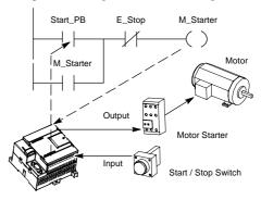
Figure 4-1 Controlling Inputs and Outputs
