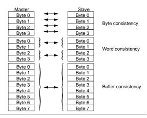
Figure A-29 Byte, Word, and Buffer Data Consistency
