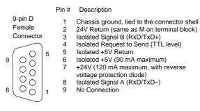
Note: Isolated means 500V of isolation from digital logic and 24V input power.
