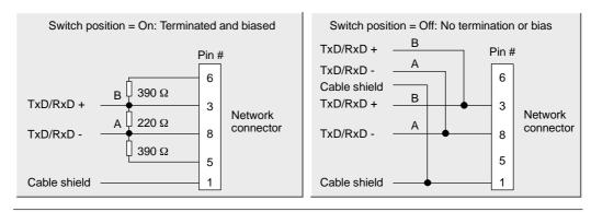
Figure 11-5 Bias and Termination of the Network Cable
