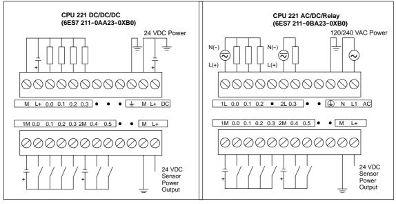
Figure A-3 CPU 221 Wiring Diagrams
