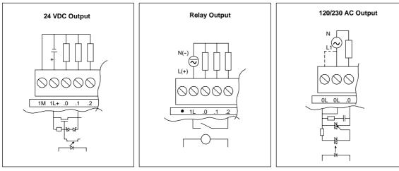
Figure A-8 S7-200 Digital Expansion Modules Outputs
