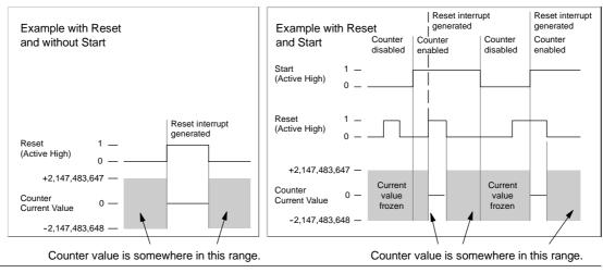
Figure 6-27 Operation Examples Using Reset with and without Start
