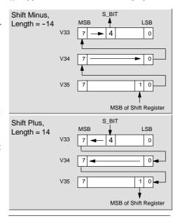
Figure 6-35 Shift Register Entry and Exit
