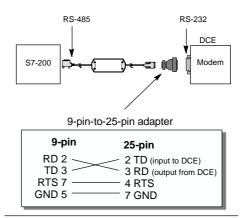
Figure 7-30 Pin Assignments for Adapters
