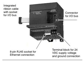
Figure A-40 Connecting the (CP 243-1) Ethernet Module
