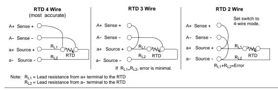
Figure A-25 Wiring the RTD to the Sensor by 4, 3, and 2 Wire
