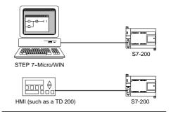
In both sample networks, the S7-200 CPU is a slave Figure 7-10 Single-Master PPI Network that responds to requests from the master.
