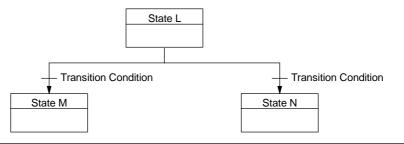
Figure 6-34 Divergence of a Control Stream, Depending on the Transition Condition
