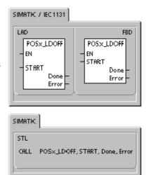
Turning on the START parameter sends a LDOFF command to the Position module. For each scan when the START parameter is on and the Position module is not currently busy, the instruction sends a LDOFF command to the Position module. To ensure that only one command is sent, use an edge detection element to pulse the START parameter on.
