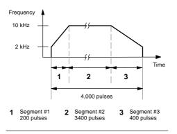
Figure 6-30 Frequency/Time Diagram
