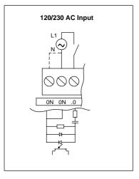
Figure A-7 S7-200 Digital Expansion Modules Inputs
