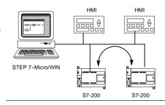
Figure 7-14 HMI Devices and Peer-to-Peer
