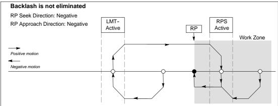
Figure 9-25 Placement of the Work Zone with and without the Elimination of Backlash
