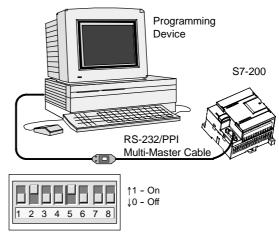
Figure 2-2 Connecting the RS-232/PPI Multi-Master Cable
