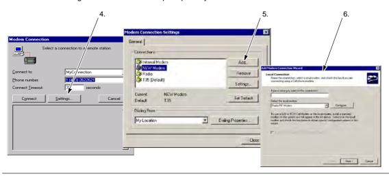
Figure 7-24 Adding a Modem Connection
