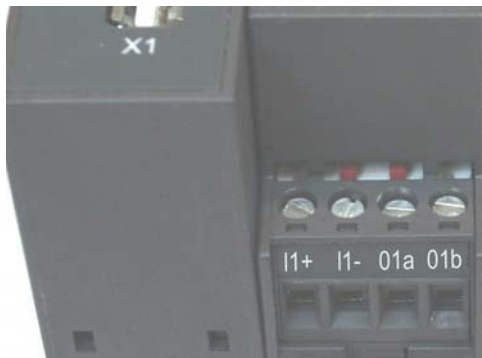
Figure 3-1 Connectors for in port and out port on the underside of the device
