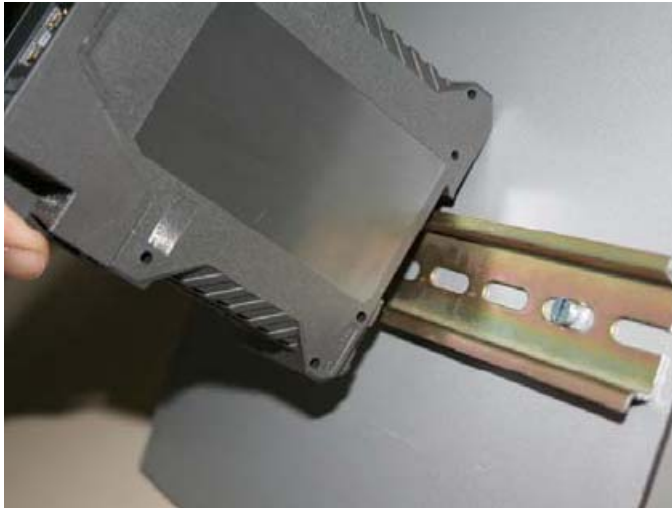
Figure 3-6 Installation on a DIN rail
