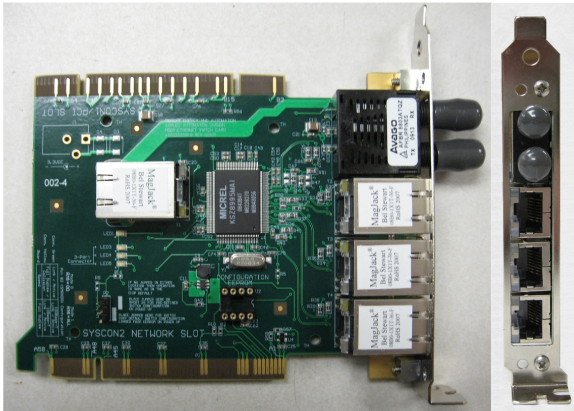
Figure 8: Ethernet Switch Board with Fiber (ESBF)
