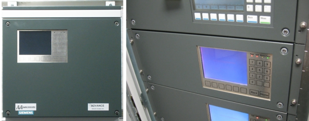
Figure 12: Network Access Unit Wall Mounted (Left) and Rack Mounted (Right)
