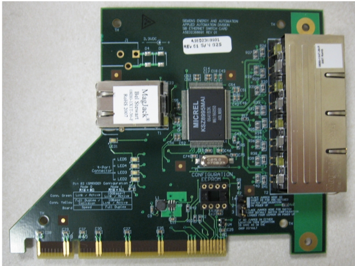
Figure 7: Ethernet Switch Board (ESB)
