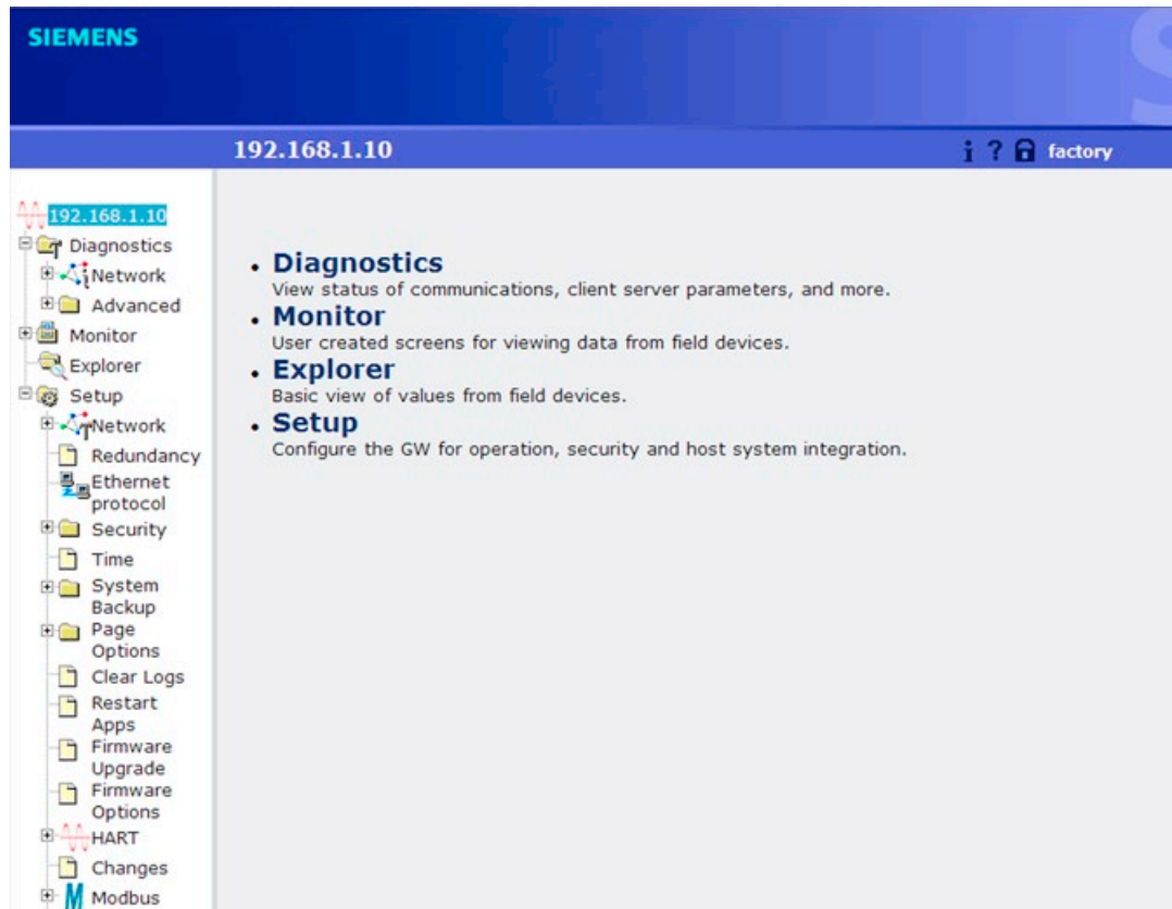
Figure 4-1 Start page of the Web-based configuration tool of the Link
