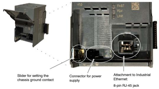
Figure 3-1 Connectors with Front Panel Opened
