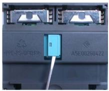
Figure 3-2 Fitting the C-PLUG and Removing It from the CP with a Screwdriver
