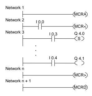
MCR functionality is activated by the MCRA rung. The rungs between the MCR< and the MCR> (outputs Q4.0, Q4.1) are executed as follows:
