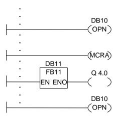
The Ladder rungs shown above are program sections from a function block written by a user. In this FB, DB10 is opened and MCR functionality is activated. If the unconditional call of FB11 is executed, the following occurs:
