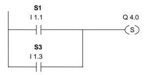
Network 2: Pressing either stop switch or opening the normally closed contact at the end of the belt turns the motor off.
