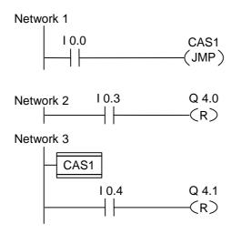
If 10.0 = "1", the jump to label CAS1 is executed. Because of the jump, the instruction to reset output Q4.0 is not executed even if there is a logic "1" at 10.3.
