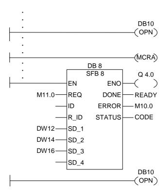
The Ladder rungs shown above are program sections from a function block written by a user. In this FB, DB10 is opened and MCR functionality is activated. If the unconditional call of SFB8 is executed, the following occurs:
