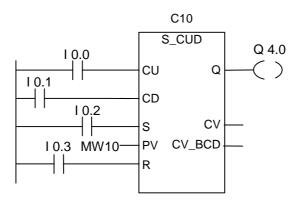
If I0.2 changes from "0" to "1", the counter is preset with the value of MW10. If the signal state of I0.0 changes from "0" to "1", the value of counter C10 will be incremented by one - except when the value of C10 is equal than "999". If I0.1 changes from "0" to "1", C10 is decremented by one - except when the value of C10 is equal to "0". Q4.0 is "1" if C10 is not equal to zero.
