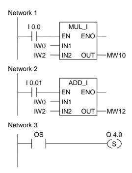
The MUL\_I box is activated by signal state "1" at I0.0. The ADD\_I box is activated by logic "1" at I0.1. If the result of one of the math functions was outside the permissible range for an integer, the OS bit in the status word is set to "1". Q4.0 is set if the scan of OS is logic "1".
