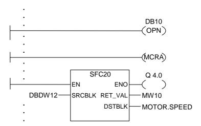
The Ladder rungs shown above are program sections from a function block written by a user. In this FB, DB10 is opened and MCR functionality is activated. If the unconditional call of SFC20 is executed, the following occurs:
