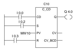
If I0.2 changes from "0" to "1", the counter is preset with the value of MW10. If the signal state of I0.0 changes from "0" to "1", the value of counter C10 will be decremented by one - unless the value of C10 is equal to "0". Q4.0 is "1" if C10 is not equal to zero.
