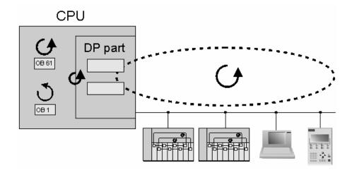
In this case, the situation corresponds to the example given above with the difference that all cycles (up to the OB 1 cycle) are of equal length and synchronously cycled. The clock pulse generator is comprised of the DP master constant bus cycle time clock that is sent as the global control frame to the DP slaves. A synchronous cycle interrupt OB 61 (or OB 61 to OB 64) ensures that it is synchronized with the user program.
