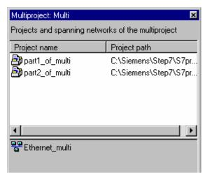
The upper section of the window displays the projects of the multiproject. The lower section displays all cross-project subnets of the multiproject under their master subnet name.
