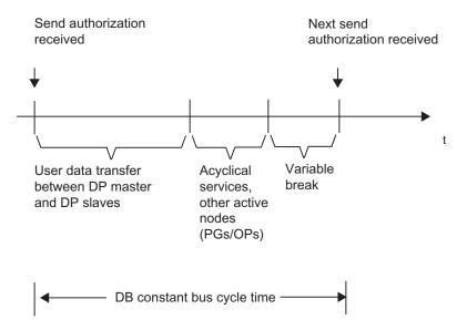
The "variable pause" shown in the figure is always minimal if communication jobs, for example, for other active nodes are still pending. The master (also known as the constant-bus-cycle-time master) controls the communication parts so that the same duration for a bus cycle is always achieved.
