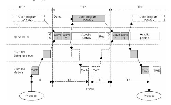
In the previous example, the DP master handles the cyclic master-slave data exchange with slaves 1 and 2. After this comes the processing of the acyclic portions for interrupts, bus acceptances or diagnostic services. The DP master then retains it for a reserve time until the configured constant DP bus cycle time has expired in order to compensate for possible network disturbances and retrieve possible message frame repeats. At this point, a new DP cycle starts with the global frame (GC).
