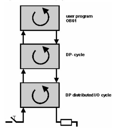
With constant bus cycle time and cycle synchronization, all cycles concerned have the same cycle time and length. This keeps the process reaction times of equal length and, because there are no cycle jumps, they are also shorter. This means that the previously described case in which information transmission can occur in the first or second cycle, depending on the position of individual cycles, now no longer applies.
