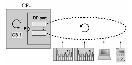
In the previous example, the behavior is depicted without constant bus cycle time and cycle synchronization by using a model structure with a DP master, two DP slaves, a programming device (PG) and an OP. This configuration yields the following subcycles, with their own cyclic and acyclic portions:
