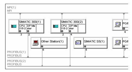
You can now assign your PG one of the "PG/PC" symbols (to identify the device you intend to use for accessing stations online). Assignment updates the interfaces in the programming device (PG or PC) to match the configured settings. If you change your configured settings (e.g. by modifying the transmission rate or another network property), the interface in your PG or PC will be updated automatically.
