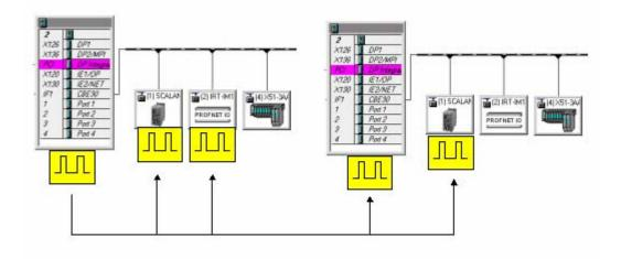
3. Now configure the topology; that is, specify how the ports for the individual devices are interconnected.
