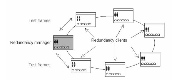
If no test frames arrive within a time interval, the manager lets TCP/IP frames through again. In this way, a communications path for TCP/IP frames, which had been previously interrupted for the reason cited above, is created again. If the ring opens, the redundancy manager generates a redundancy interrupt.
