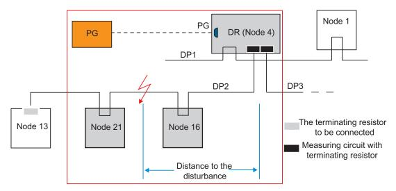
If STEP 7 does not localize the error in segment "DP2" or if, for example, this segment contains more than 32 partners and the Diagnostic Repeater cannot operate correctly anymore, you are shown the following image:
