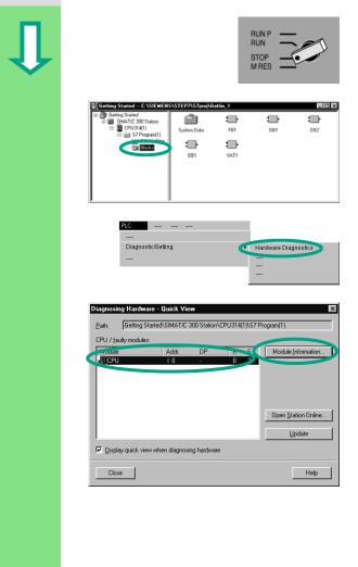
First turn the operating mode switch on the CPU to STOP.
