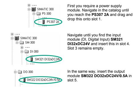
In order to change the parameters (for example, address) of a module within a project, double-click the module. However, you should only change the parameters if you are sure you know what effects the changes will have on your programmable controller.
