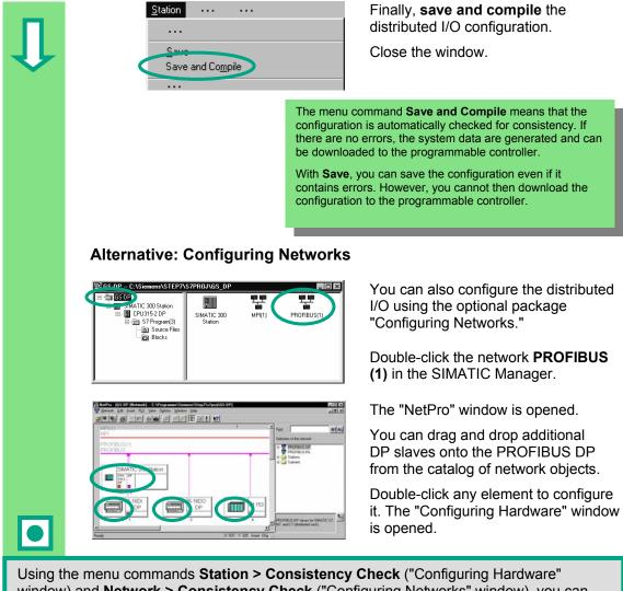
Using the menu commands **Station > Consistency Check** ("Configuring Hardware" window) and **Network > Consistency Check** ("Configuring Networks" window), you can check the configuration for errors before saving. Any errors are displayed and STEP 7 will suggest possible solutions.
