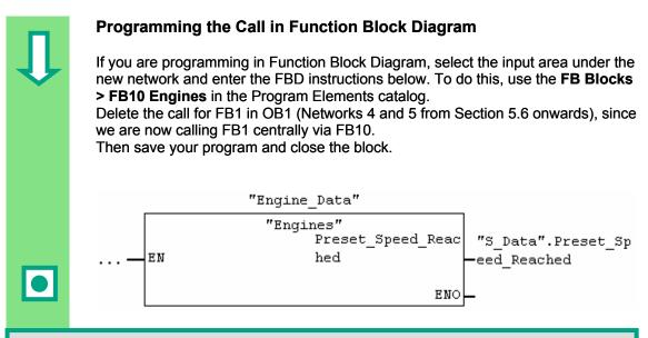
If you require additional engine control programs for your automation task; for example, for gas engines, hydrogen engines, etc., you can program these as multiple instances in the same way and call them from FB10.
