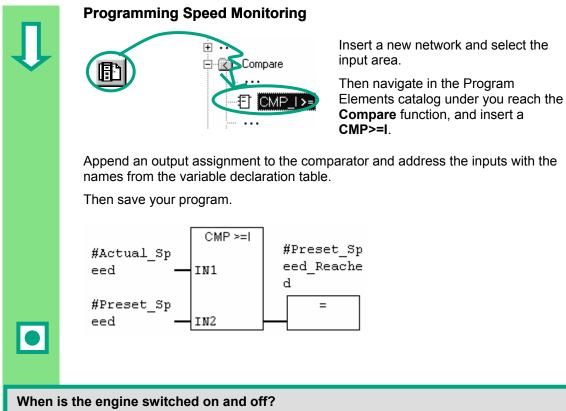
When the variable #Switch\_On has signal state "1" <u>and</u> the variable "Automatic\_Mode" has signal state "0," the engine is switched on. This function is not enabled until "Automatic Mode" is negated (normally closed contact).
