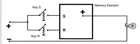
If key S is pressed, the bulb lights up and remains lit until key R is pressed.
