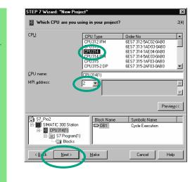
For the "Getting Started" sample project, select CPU 314. The example has been created in such a way that you can actually select the CPU you have been supplied with at any time.
