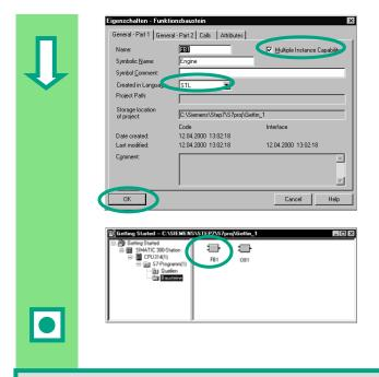
In the "Properties – Function Block" dialog box, select the language in which you want to create the block, activate the check box "Multiple instance FB," and confirm the remaining settings with OK.
