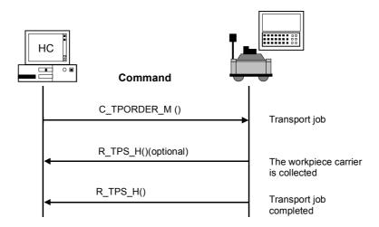
Fig. 8-1 Transport dialog, normal situation, no errors
