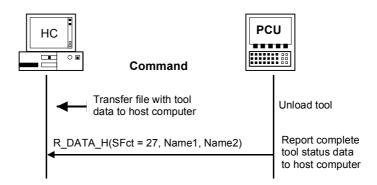
Fig. 5-16 Unload tool, initiated by the SINUMERIK
