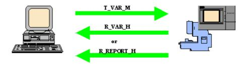
The VisualBasic application requests the value of an R parameter with the RPC: **T\_VAR\_M()**.
