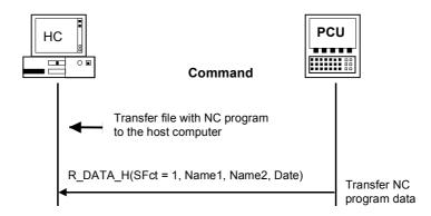
Fig. 5-7 Transfer NC program, initiated by the SINUMERIK
