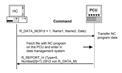
Fig. 5-6 Transfer NC program, initiated by host computer
