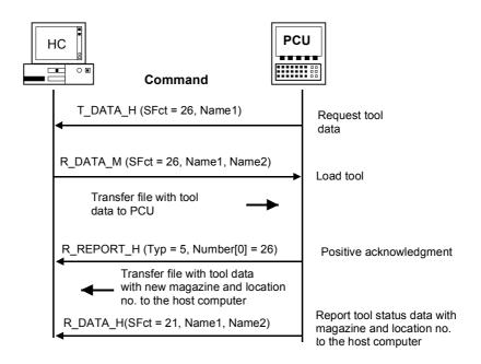
Fig. 5-15 Load tool, initiated by the SINUMERIK
