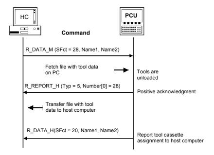
Fig. 5-19 Unload tool pallet/cassette
