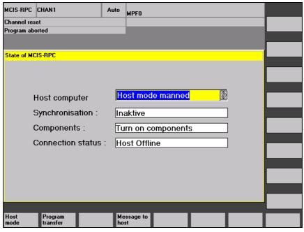
Fig. 3-1 The screen allows you to change the host computer mode
