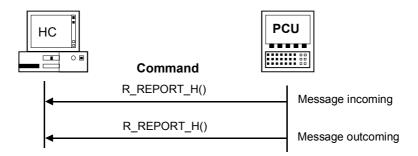
Fig. 5-2 Procedure for alarms/operator interruptions/operational messages
