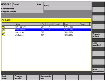
Fig. 3-2 Transferring NC programs/files
