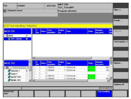
Fig. 3-10 Entry screen for tool handling/selection
