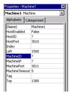
When you change the attribute: **MachinelD**, the display of the OCX in the form also changes. Sending of the RPC **T\_MACHINE\_M** is triggered by clicking on the "DoRPC" button. The RPC SINUMERIK application responds with the RPC **R\_MACHINE\_H**. The response to this in the example application is a message box.
