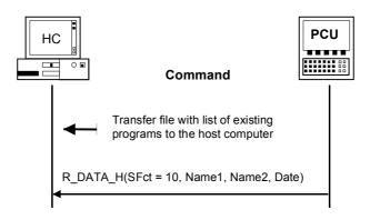
Fig. 5-12 Transfer NC program list to the host computer
