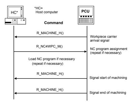
Fig. 5-1 Production dialog, normal execution, no errors
