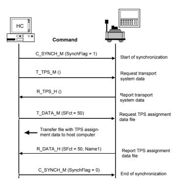
Fig. 8-2 TPS synchronization, initiated by host computer
