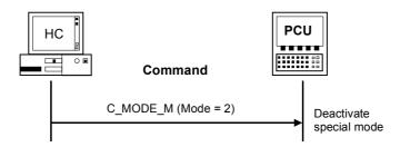
Fig. 5-22 Deactivate special mode, initiated by the host computer
