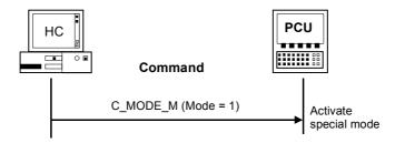
Fig. 5-21 Activate special mode, initiated by the host computer
