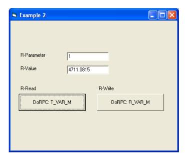
To activate the variable service of RPC SINUMERIK, at least one variable set must be defined in the file c:\add\_on\scvarset.ini on the controller. Changes in this file only become effective after the next cold restart of the controller. If this is not the case, RPC SINUMERIK responds with the RPC: R\_REPRT\_H() and the error: -800.
