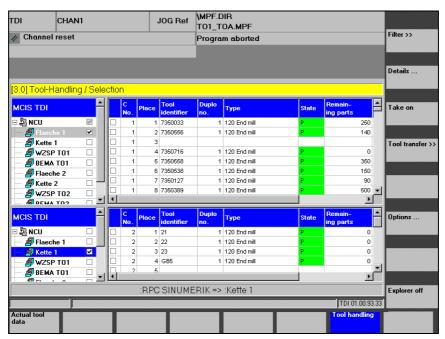
Fig. 3-9 Tool handling with status line
