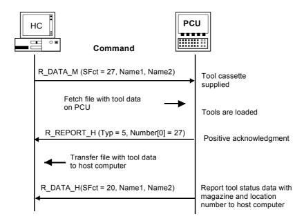
Fig. 5-18 Load tool pallet/cassette
