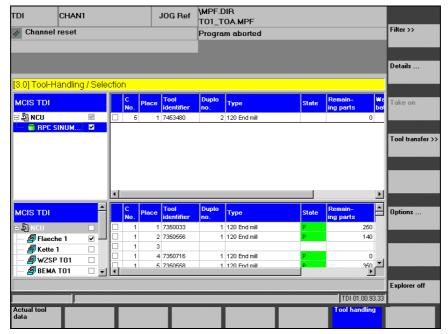
Fig. 3-13 Tool handling/filters: Request completed
