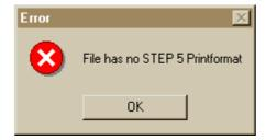
This error message is displayed if the selected file is not in valid STEP 5 print format or if it has not been created with the printer parameter file S5FILEDR.INI.
