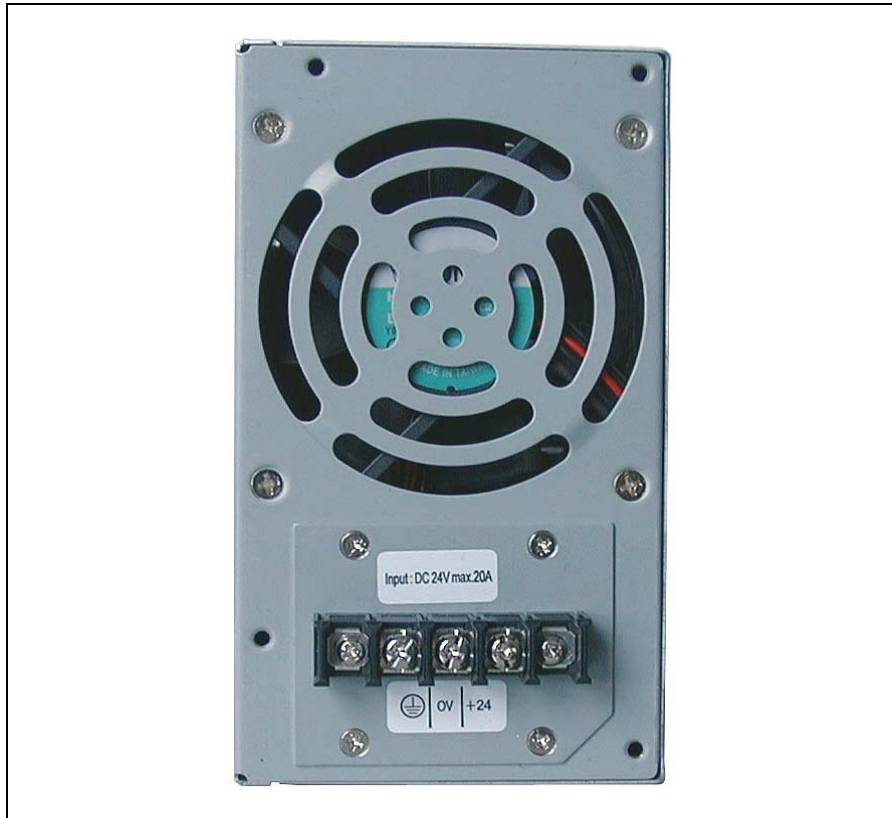
Figure 1-5 24 V power supply
