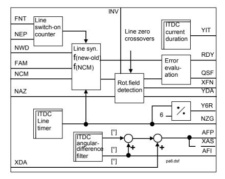
The ITDC generates, as function of internal counter statuses, the interrupt to start the FB-PA6 via the local extension bus (LE). This is realized in synchronism with the firing pulses.
