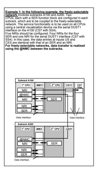
• It transfers data blocks from a serial interface (corresponding to the data entry at input CTS) to an additional serial interface (corresponding to the data entry at input ISA).
