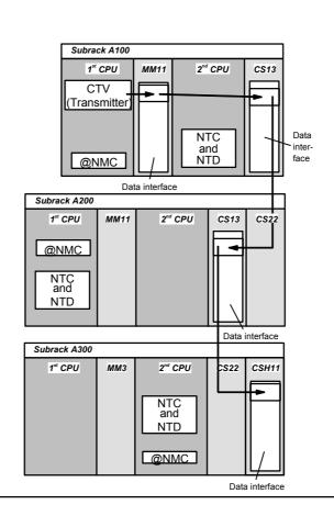
If a data transfer route ends or starts on a CSH11 or CS7 (which submodule is irrelevant), then the following restriction exists regarding the data transfer modi (e.g. handshake):
