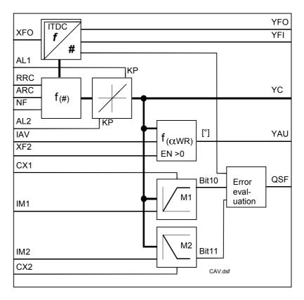
The current actual value sensing in the converter is either bipolar or unipolar, e.g. as for the Sitor set. For a signed current actual value, the actual value is checked to see whether it violates limits CX1 and CX2. YC > CX1  $\Rightarrow$  QSF \ bit10 = 1 overcurrent, torque direction 1
