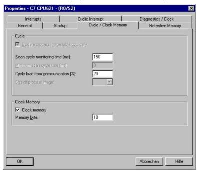
Activate the *Clock Memory* checkbox and enter 10 for the number of the memory byte. Each bit of the clock memory byte is assigned a period time/frequency:
