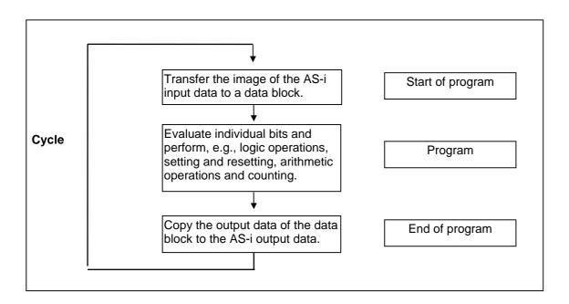
Because the bits of the AS-i line can only be accessed in word mode or doubleword mode, it is necessary to set up a memory data block. In the data block the AS-i data can be accessed in bit mode.
