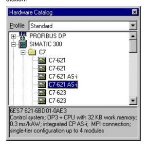
Double-click on *C7-621 AS-i* to insert the device into slot 2 in the Hardware Configuration window. Here you will see information on the set MPI address of the C7-CPU (default setting for the MPI address is 2) and an address map.
