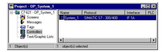
Open the Controller System\_1 by double-clicking.
