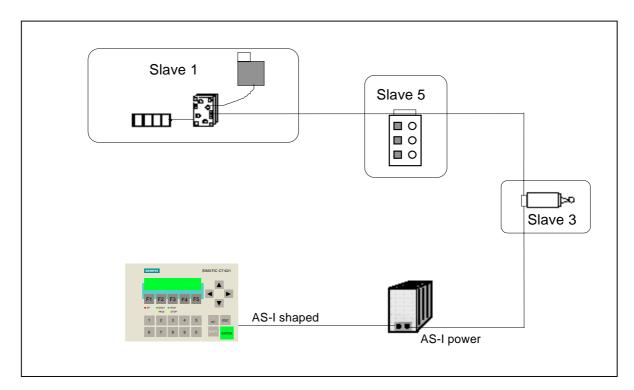
Set up your AS-i network according to the diagram above. Connect your slave 1 to your yellow AS-i shaped cable. If you have problems connecting the slaves to the AS-i cable, please read the setup instructions supplied with the AS-i components.
