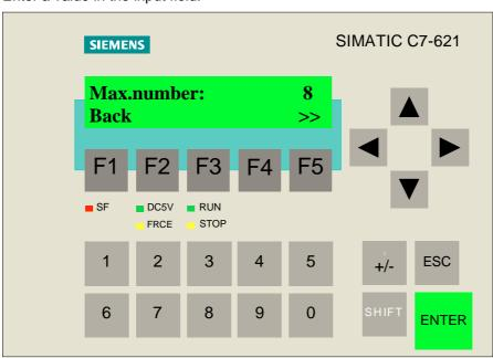
Activate the softkey to reach the second screen entry. Now check the functionality of your inductive proximity switch including the count function.
