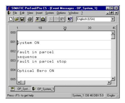
In the status line (not shown in the figure), you will see the relevant address which connects the message to the PLC. In your example, for message no. 001 the address is System ON: DB 46 DBX 5.0.
