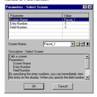
Close the dialog boxes *Parameters - Select Screen and Softkey F5* by clicking the *OK* button. A function is now assigned to the softkey.
