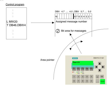
The above figure shows the connection between the PLC and the OP when a message appears. The process is described in detail below.
