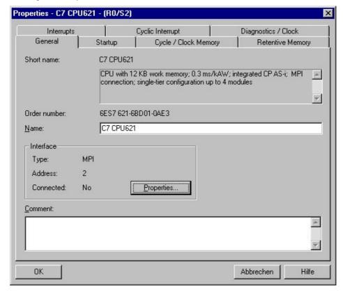
Open the *Properties - MPI Nodes* window by clicking the button *Properties ...*, and select the *Subnet: MPI(1)*. Accept the settings with *OK*, save and compile the hardware configuration, and load it into the C7 CPU again.
