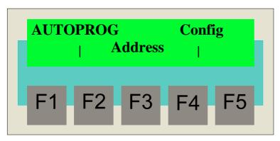
For setting addresses, the mode set for the device must be the configuring mode. When the C7 is shipped, this mode is preset by default.
