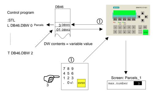
The values of the input are stored in the data interface (DB46).
