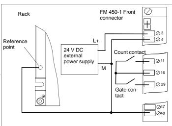
**Test:** Turn on the power supply module and the external 24 V DC power supply. The red EXTF LED on the FM 452 is lights up briefly and goes off again. The INTF LED remains lit since you have not yet entered the FM 452 in the hardware configuration.
