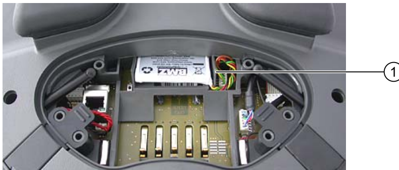
① Cable routing
