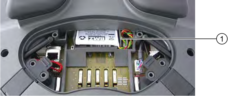
① Cable routing
