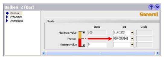
5. In the same way, assign the tags to the remaining 6 bars. Make sure that each element of the PERCENT array variable is incremented by the count of 1.
