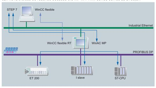
Figure 4-4 Routing from Ethernet to PROFIBUS DP with WinAC MP
