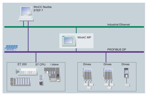
Figure 2-1 Embedded automation with WinAC MP 2008
