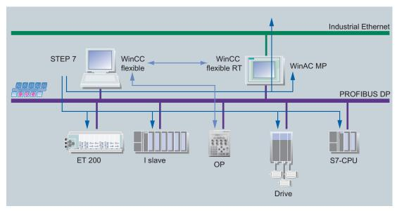
Figure 4-5 Routing with WinAC MP over PROFIBUS
