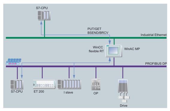
Figure 4-7 CPU-CPU communication over WinAC MP
