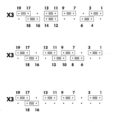
With jumpers 12-14 and 4-6 the two-wireline R has the control signal, the break status will be regonized (default). Pin 4 (R(A)) of the front connector is connected to +5 V via resistor. Pin 11 (R(B)) of the front connector is connected to ground via resistor.
