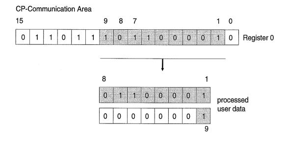
In the example above two bytes with the values 61H and 01H are transmitted by the CP to the link partner in the form of a response.
