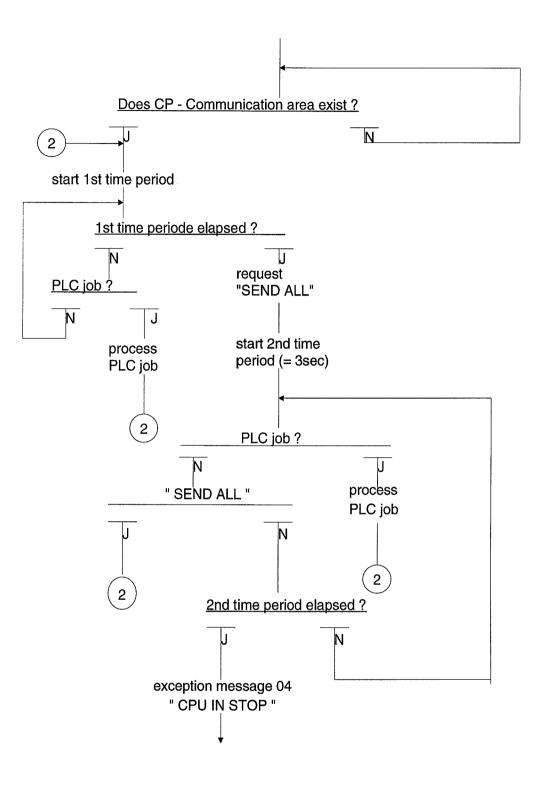
The following points describe how the "SEND" and/or "FETCH" jobs activated in the S5 program may influence the cycle test initiated by the CP. In this instance the time of triggering (= first or second time period) is irrelevant!
