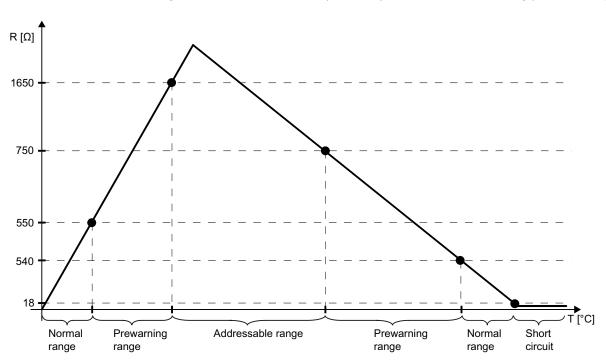
The diagram below shows the temperature pattern and the switching points belonging to it.
