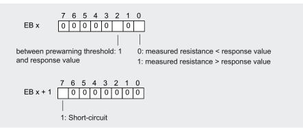
Assignment in the process input image (PII) in the case of SIMATIC S5
