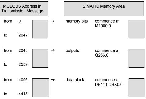
The Modbus coil addresses from 0 to 2047 access the SIMATIC memory bits commencing at memory bit M 1000.0; i.e. length of area = 2048 bits = 256 bytes, which means last memory bit = M 1255.7.
