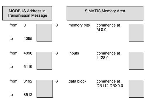
The Modbus addresses from 0 to 4095 access the SIMATIC memory bits commencing at memory bit M 0.0; i.e. length of area = 4096 bits = 512 bytes, which means last memory bit = M 511.7.
