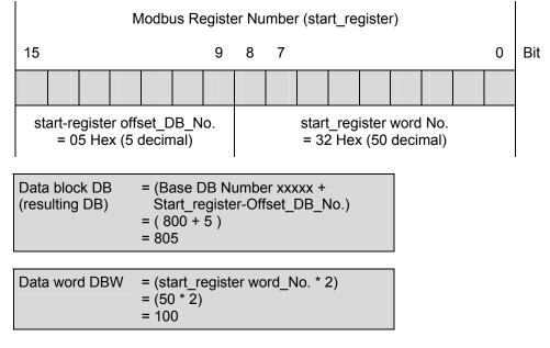
Write access is made to DB 805, data words DBW 100 to DBW 104.
