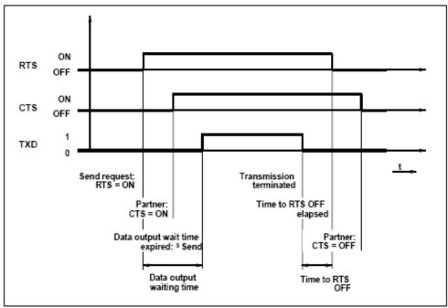
Figure 7-1 Time Diagram for Automatic Use of the RS 232C Secondary Signals
