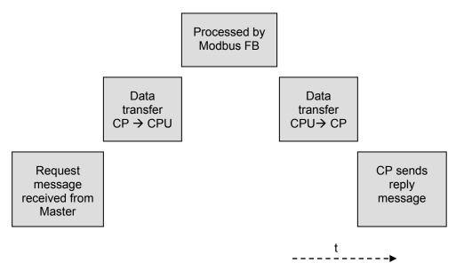
The reaction times depend on the cycle time of the CPU program (Modbus FB) and the CPU type (data transfer CPU<-->CP).
