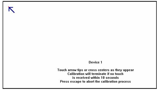
Figure 1-11 Touch screen calibration
