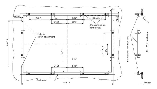
Figure 1-4 Dimensioned drawing mounting cut-out
