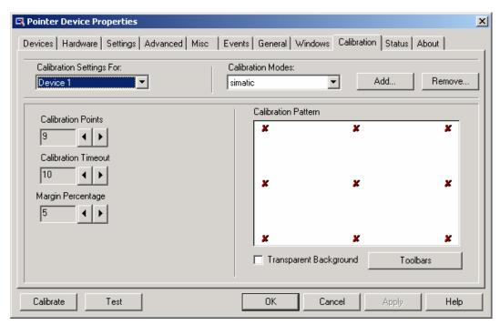
Figure 1-13 Touch defaults, "Calibration" tab
