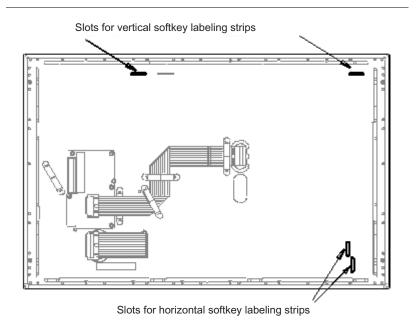
Figure 1-2 Device rear with connections and slots for the labeling strips
