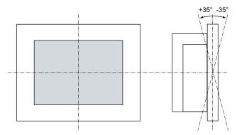
Figure 1-3 Permitted mounting positions
