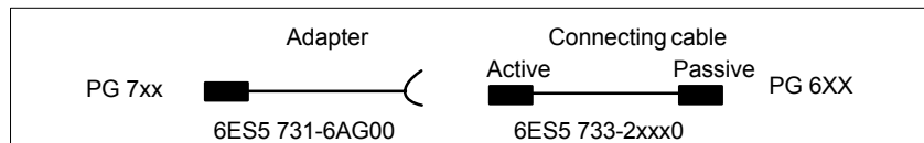
Figure 3-10 Direction of Connection: Adapter - Connecting Cable
