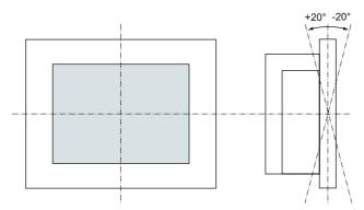
Figure 1-1 Permitted mounting positions
