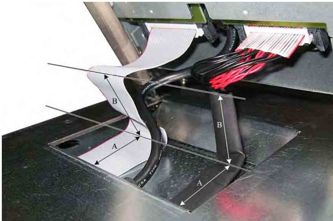
Figure 12-3 Separate the control unit from the computer unit, example regarding folding cables
