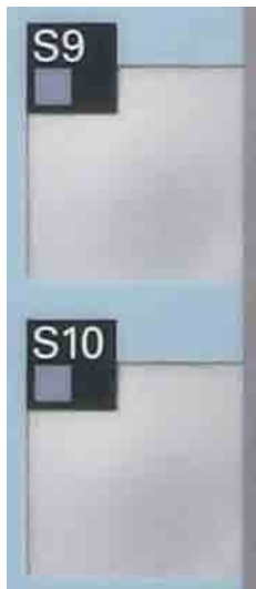
Figure 10-3 Softkeys with LEDs, taking the 15" control unit as an example
