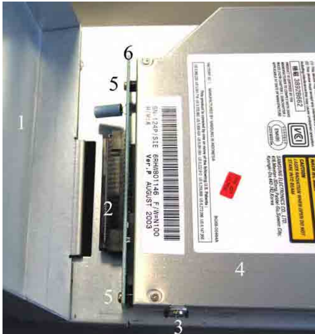
Figure 12-7 Drive removed, housing flipped up
