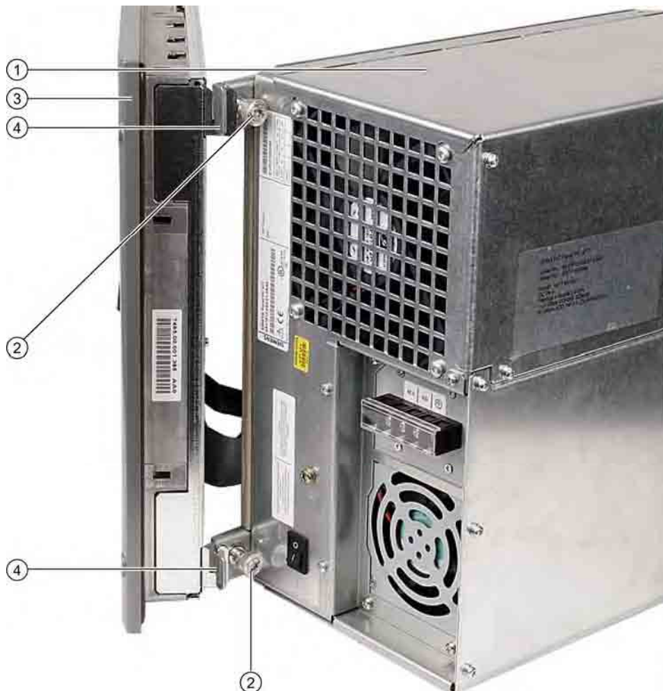
Figure 12-1 Separating the control unit from the computer unit
