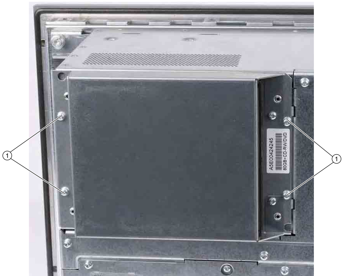
Figure 12-4 Installing and removing the optical drive
