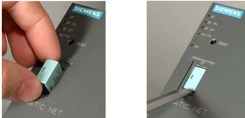
Figure 3-2 Fitting a C-PLUG in the IWLAN/PB Link PN IO and Removing a C-PLUG from the IWLAN/PB Link PN IO using a Screwdriver
