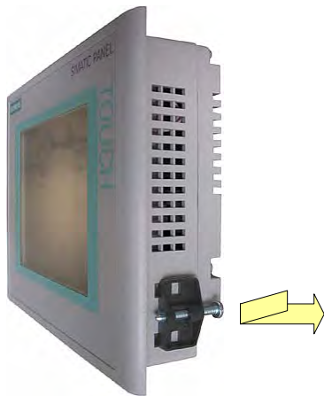
Figure 4-11 Installing the mounting clamp on the HMI device
