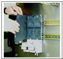
Shift the control unit ICU24(F) in parallel to the guide rails into the terminal module until the upper and lower locking spring engages.
