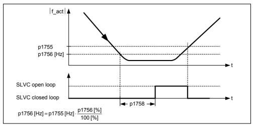
Fig. 7-6 Changeover condition for SLVC
