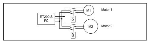
Fig. 6-6 Changing-over the drive data set to activate the drive parameter for motor 2
