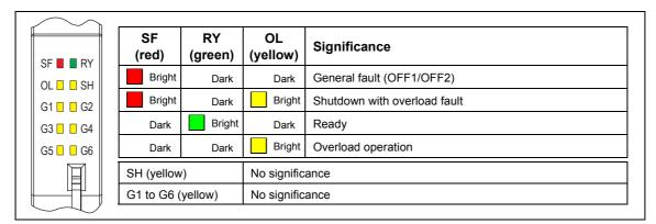
Fig. 2-19 LED state display on the front panel of the ICU24
