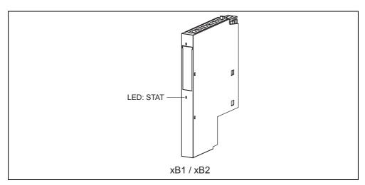
Fig. 2-23 Brake control module xB1 / xB2
