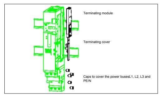
Fig. 3-7 Inserting the terminating cover with caps
