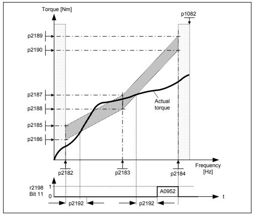
Fig. 8-5 Load torque monitoring (p2181 = 1)
