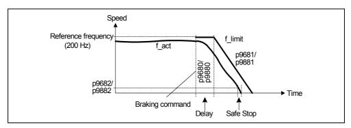
Fig. 6-34 "Safe braking ramp" function
