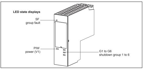
Fig. 2-12 Power/expansion module PM-D F X1
