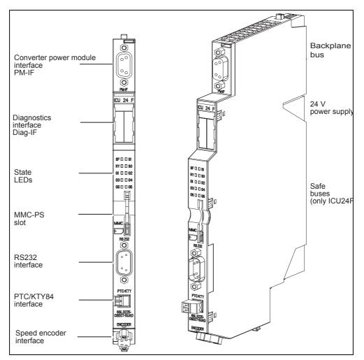
Fig. 2-18 Control unit ICU24(F) with its components
