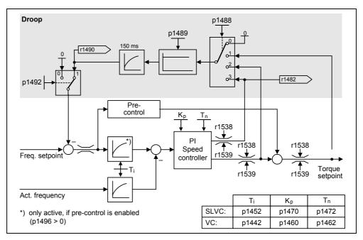
Fig. 7-11 Speed controller with droop
