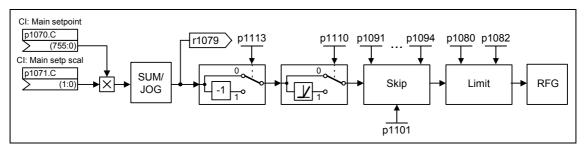
Fig. 6-18 Modifying the frequency setpoint
