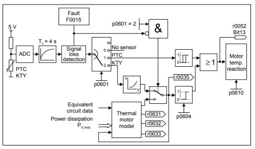
Fig. 8-1 Thermal motor protection
