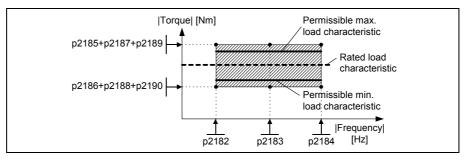
Fig. 8-3 Load torque monitoring with min. / max. permissible load characteristic
