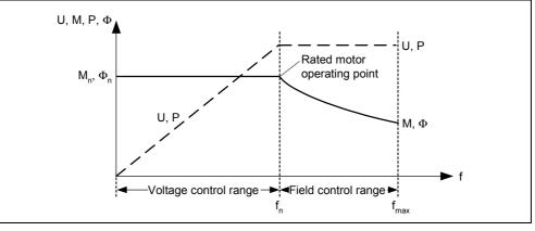
Fig. 7-1 Operating ranges and characteristics of induction motor when fed from a frequency converter
