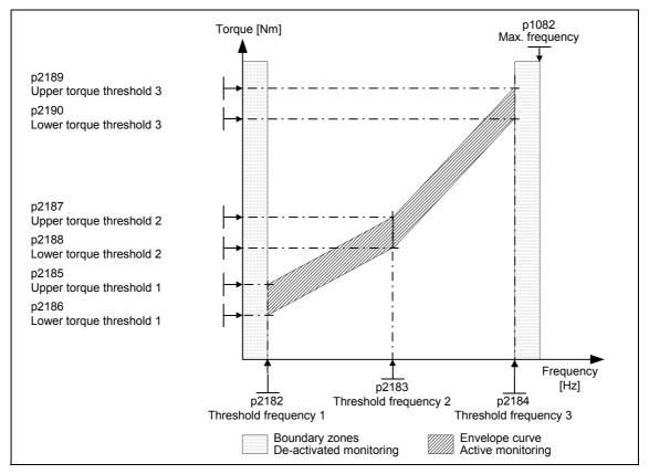
Fig. 8-6 Frequency/torque tolerance bandwidth
