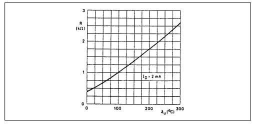
Fig. 8-3 KTY84 characteristic for 1LG / 1LA motors
