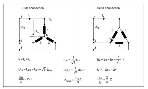
Fig. 6-14 Conversion, star / delta circuit configuration
