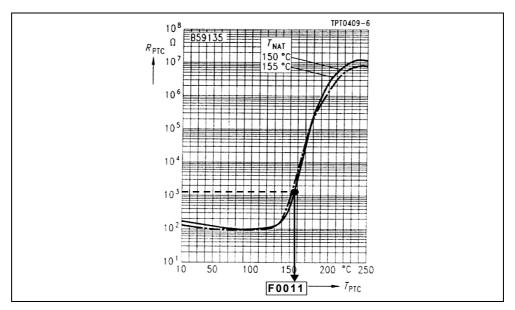
Fig. 8-2 PTC characteristic for 1LG / 1LA motors
