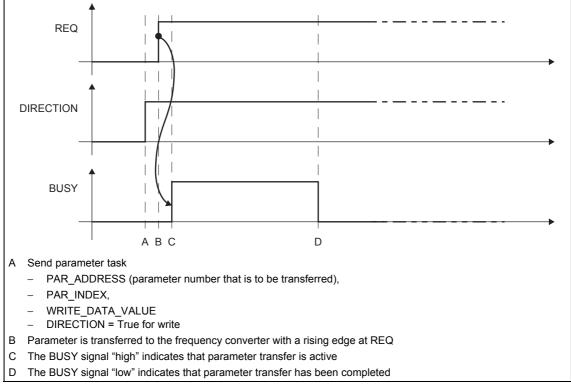
Fig. 5-4 Parameter transfer to the frequency converter
