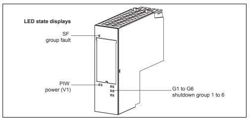
Fig. 2-15 Power/expansion module PM-D F PROFIsafe
