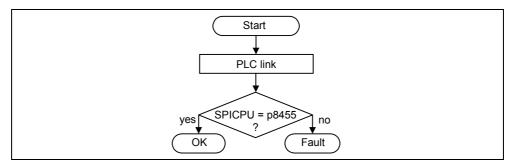
Fig. 6-31 Checking the slot ID
