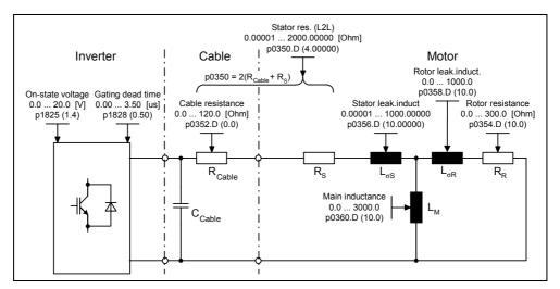
Fig. 6-15 Equivalent circuit diagram
