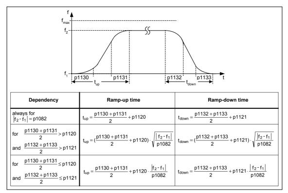
Fig. 6-20 Ramp-function generator with rounding-off
