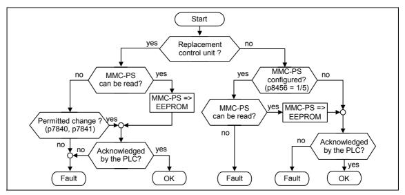
Fig. 6-37 Conditions for start of the converter
