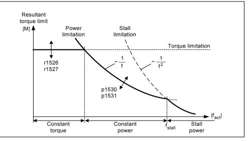
Fig. 7-13 Torque limits
