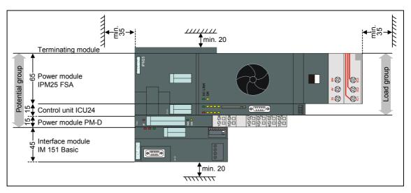
The following example shows the layout and parts list for the minimum configuration of an ET 200S station with a frequency converter.
