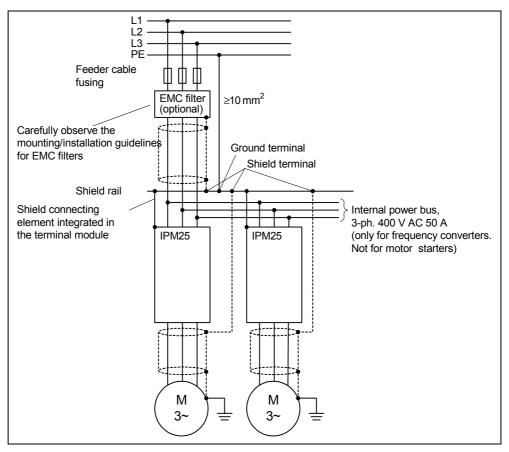
Fig. 9-1 ET 200S FC frequency converter with EMC filter
