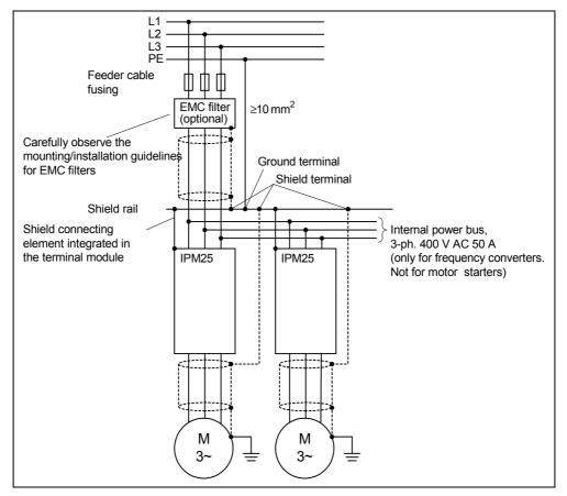
Fig. 2-24 ET 200S FC frequency converter with EMC filter
