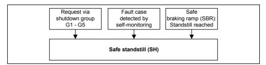
Fig. 6-32 Initiating the "safe standstill"
