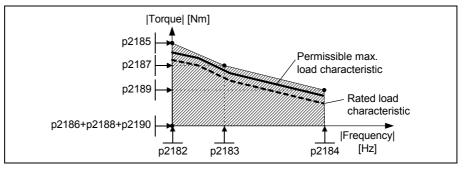
Fig. 8-2 Load torque monitoring with max. permissible load characteristic
