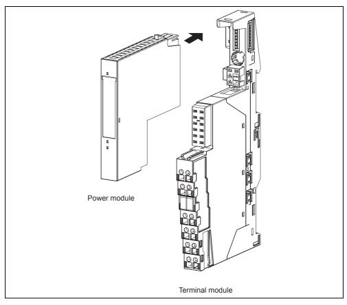
Fig. 3-4 Inserting a power module
