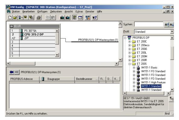
Fig. 5-1 Linking-in IM 151 in HW Config
