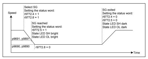
Fig. 6-36 State signals of the "safely-reduced speed" function
