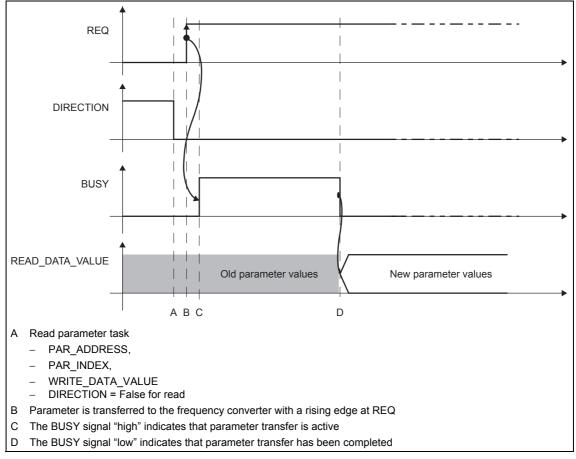
Fig. 5-5 Parameter transfer from the frequency converter
