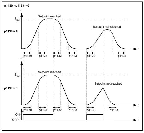
Fig. 6-21 Rounding-off after an OFF1 command
