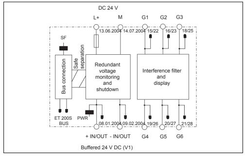
Fig. 2-14 Block circuit diagram, PM-D F X1
