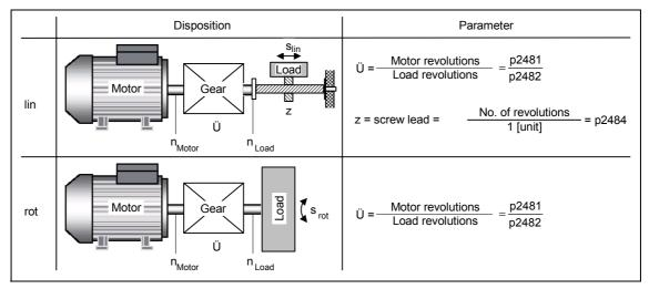
Fig. 6-24 Rotary or linear axis
