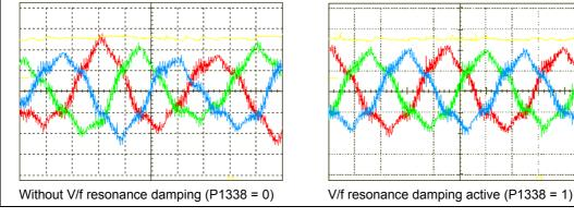
Fig. 7-4 Effect of V/f resonance damping
