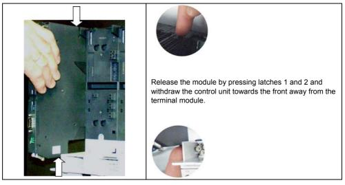
Fig. 3-6 Removing an ICU24(F)
