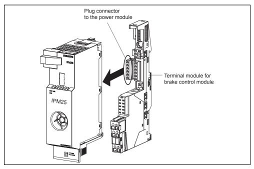
Fig. 4-3 Interface, brake control module – converter power module
