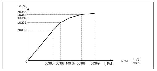
Fig. 6-16 Magnetizing characteristic
