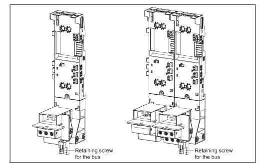
Fig. 2-6 TM-IPM65 and TM-IPM130 terminal modules
