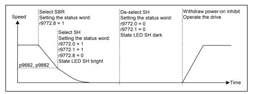
Fig. 6-35 State signals of the "safe braking ramp" function
