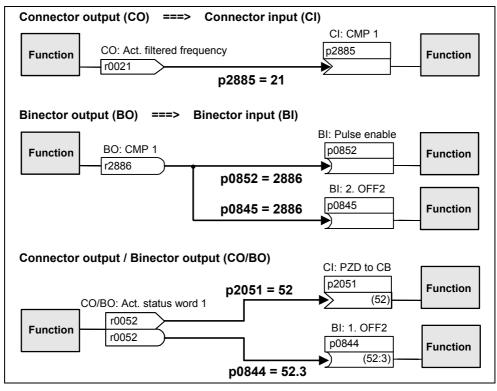
Fig. 6-5 BICO connections (examples)
