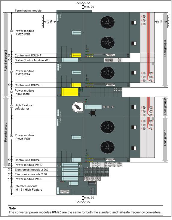
Fig. 1-4 Example for the layout of an ET 200S station
