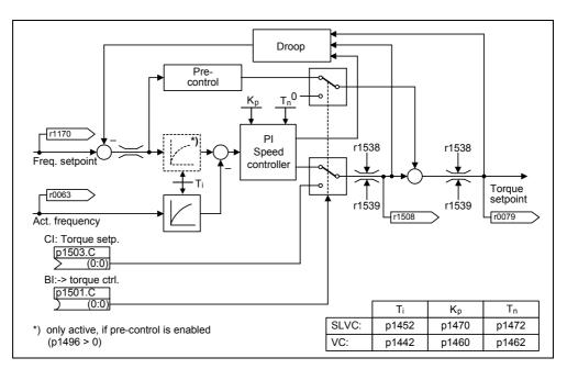
Fig. 7-12 Closed-loop speed/torque control
