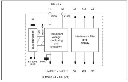
Fig. 2-17 Block circuit diagram PM-D F PROFIsafe
