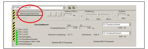
Fig. 6-11 Fetching the control priority
