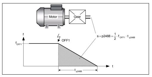
Fig. 6-23 Positioning down ramp
