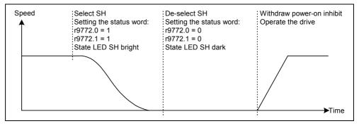
Fig. 6-33 State signals of the "safe standstill" function
