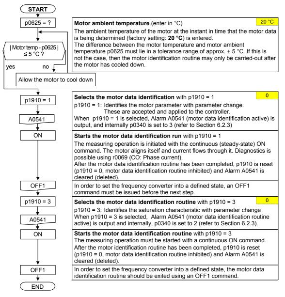
If problems occur during the identification routine, e.g. if the current controller oscillates (the frequency converter noise fluctuates), the rating plate data must be again checked and an approximately correct magnetizing current p0320 entered. The motor data identification routine should then be re-started after calling p0340 = 1 (refer to Section 6.2.3) (also refer to http://support.automation.siemens.com/WW/view/en/20279537)..
