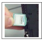
The label should point to the right so that the chamfered edge of the MMC-PS faces downwards.
