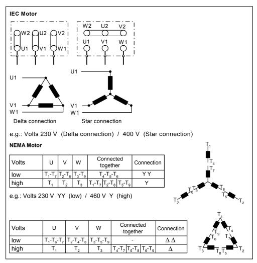
Fig. 6-13 Motor terminal box
