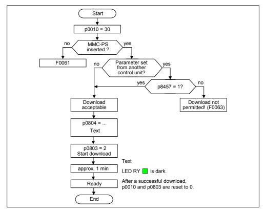
Fig. 6-39 Flow diagram to download a parameter set
