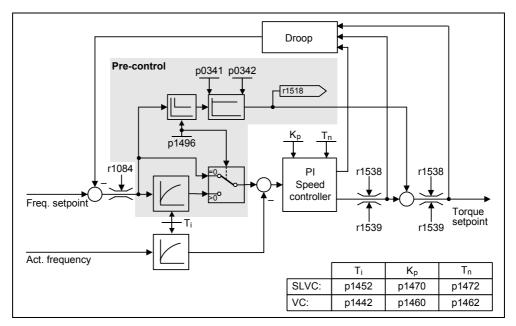
Fig. 7-10 Closed-loop speed controller with pre-control
