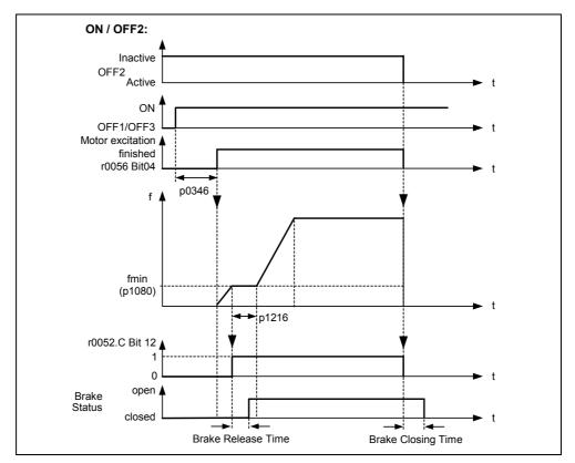
Fig. 6-27 Motor holding brake after OFF2
