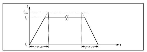
Fig. 6-19 Ramp-function generator without rounding-off
