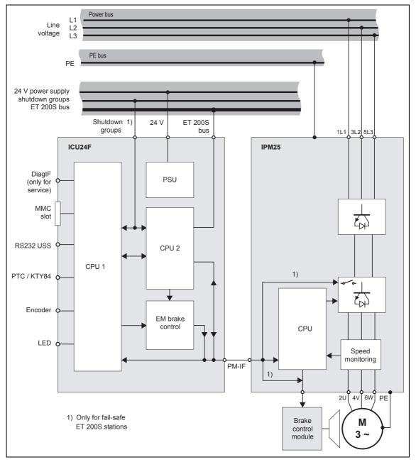
Fig. 1-2 Block diagram, fail-safe ET 200S FC
