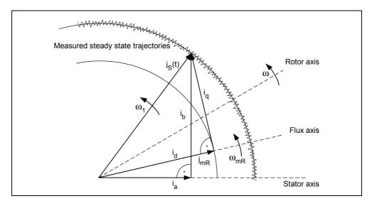
Fig. 7-5 Current Vector diagram in the steady-state condition
