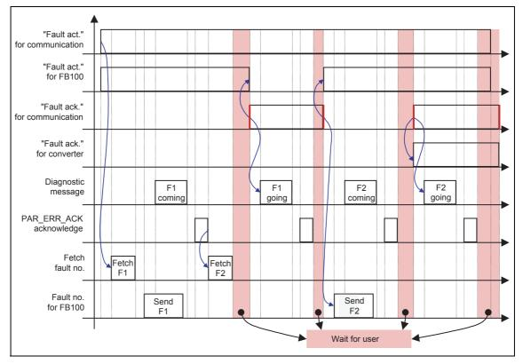
The following diagram shows how drive faults are handled.
