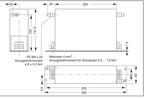
Fig. A-4 Dimension drawing EMC filter (25 A)
