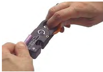
2. Measure the length to be stripped by holding the cable against the template. Mark the position using the index finger of your left hand.
