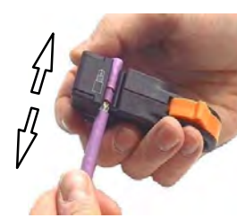
6. Keeping the tool closed, remove it from the end of the cable. If the cut is poor, change the blade cassette.
