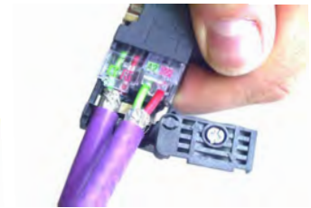
6. If you use the connector within a segment, fit the outgoing cable into the contact cover labeled A2, B2.
