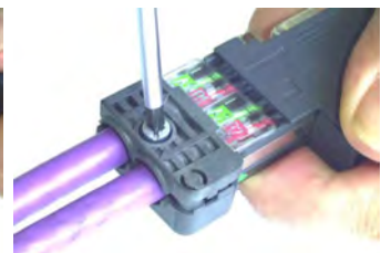
9. Tighten the screw of the strain relief clamp.
