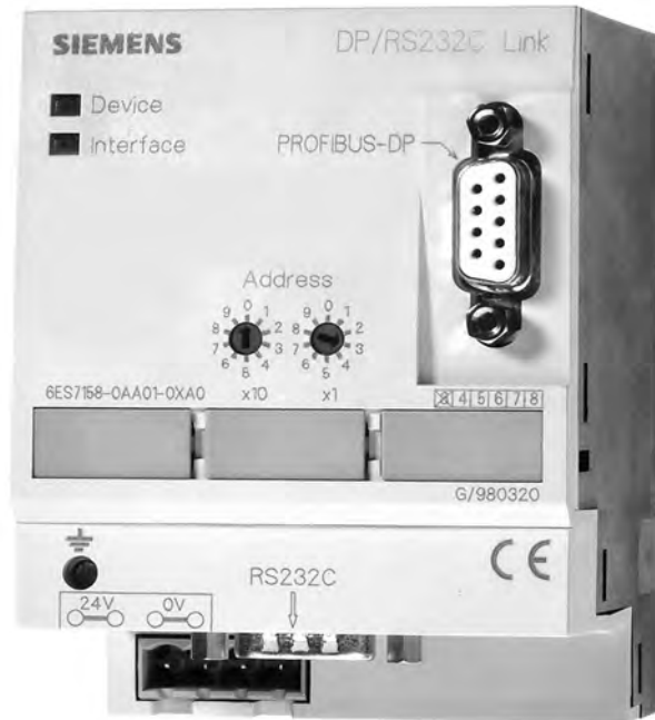
Figure 2-18 DP/RS-232C Link for PROFIBUS-DP
