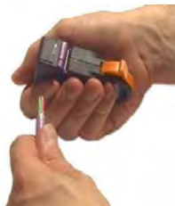
7. Remnants remain in the tool. After opening the tool, the remnants of the cable can be removed.
