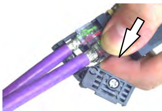
7. Press down the contact cover firmly.
