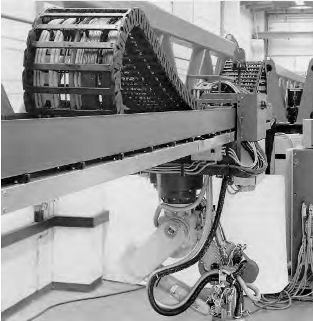
Figure 7-7 Example of Using the Glass Fiber-Optic Trailing Cable in a Drag Chain
