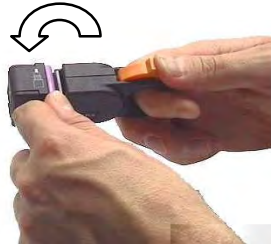
5. Turn the tool four times in the direction of the arrow for PVC insulation (eight times for PUR or PE insulation).
