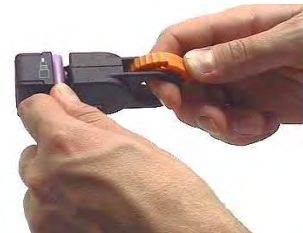
3. Insert the measured end of the cable into the tool as far as allowed by the index finger of the left hand.
