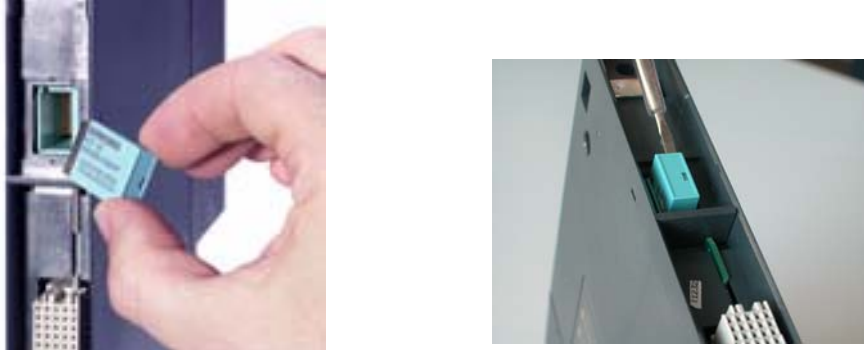
Figure 3-1 Fitting the C-PLUG in the CP and Removing It from the CP with a Screwdriver
