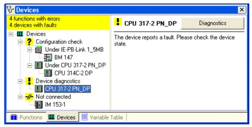
Figure 3-17 Diagnostic window, Devices tab
