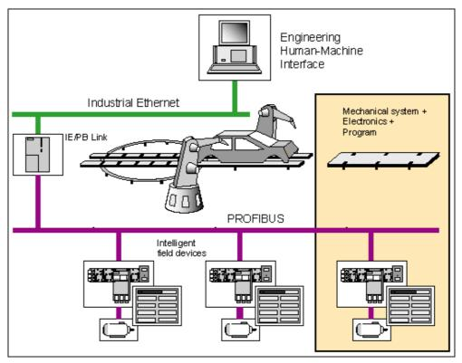
Figure 1-2 New: A modular concept with distributed intelligence
