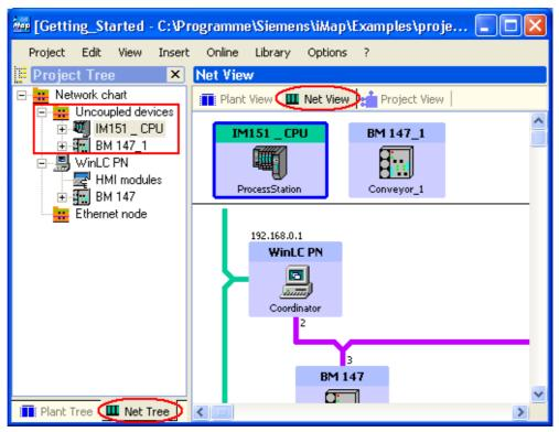
Figure 4-6 Uncoupled PROFIBUS devices
