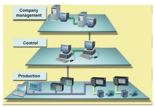
Figure 1-11 Access to process data
