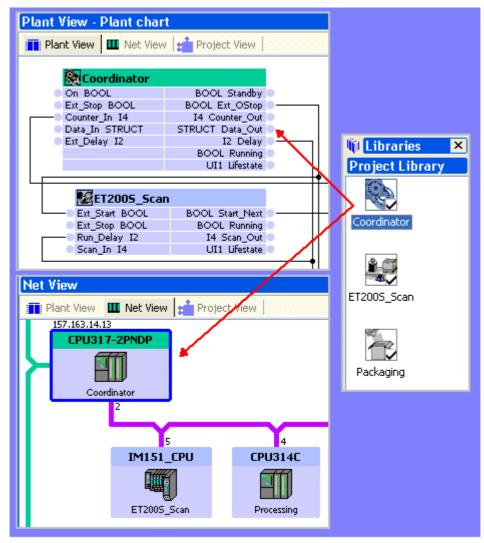
Figure 4-3 Inserting a PROFInet component into a SIMATIC iMap project
