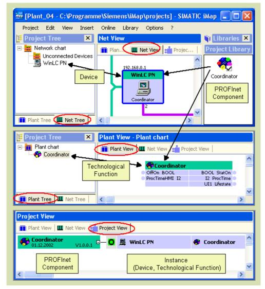
Figure 3-3 PROFInet components and their instances
