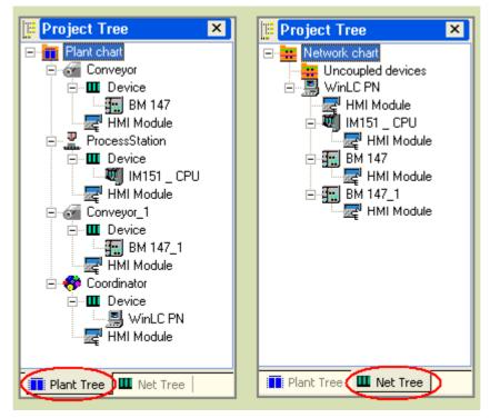
Figure 3-2 Project tree, example of an object hierarchy
