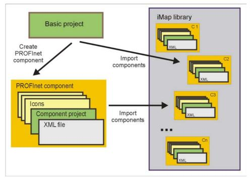
Figure 4-17 Project structure for PROFInet components
