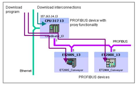
Figure 5-3 Downloading to PROFIBUS devices
