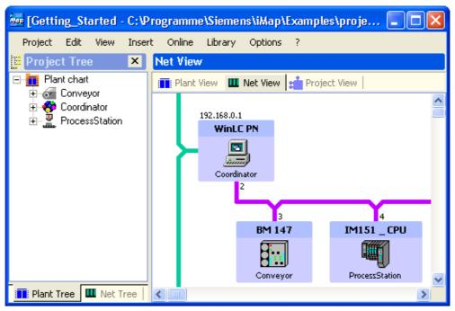
Figure 4-5 Coupled PROFIBUS devices
