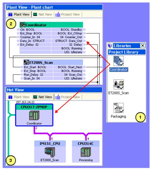
Figure 1-5 Representation of a PROFInet component in SIMATIC iMap
