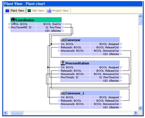
Figure 4-8 Display Interconnection Lines
