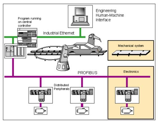
Figure 1-1 The old automation concept with a modular plant structure
