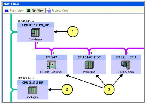
Figure 1-9 Example: Representation of the devices in the SIMATIC iMap net view
