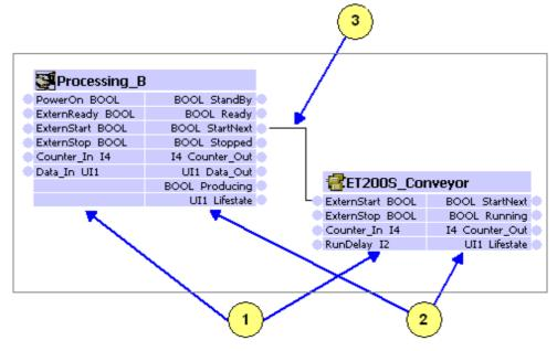
Figure 1-7 Interconnected technological functions
