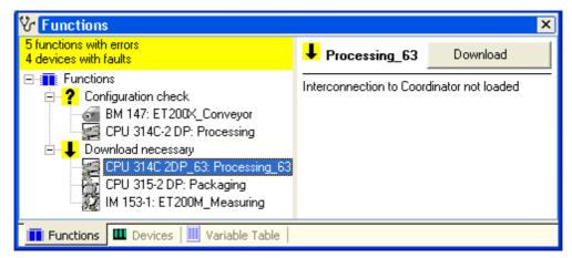
Figure 3-16 Diagnostic window, Functions tab
