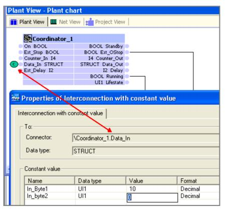
Figure 4-11 Interconnecting with constant values for a connector of the data type STRUCT
