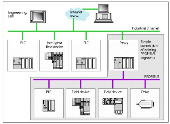
Figure 1-3 Supported network types: Industrial Ethernet and PROFIBUS
