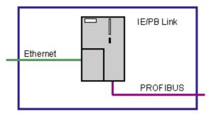
Figure 6-2 Bus ports of the IE/PB Link
