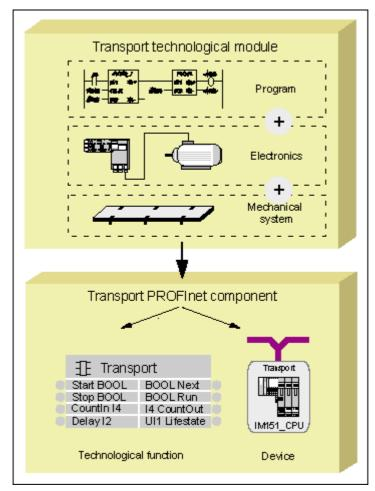
Figure 1-4 Creating a PROFInet component from a technological submodule
