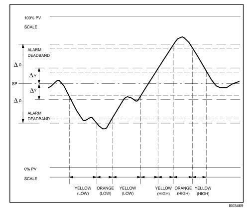
Figure 8-3 Example of Alarm Deadband For Analog Alarms
