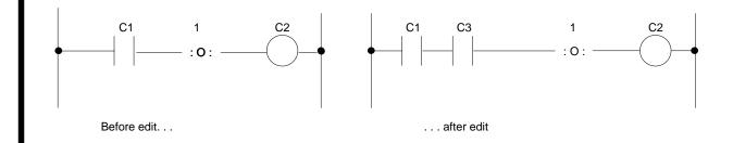
In this edit, the intent is to add a dependency on C3 for the C2 output. Due to the edit, however, the C2 output may be unexpectedly driven for one scan. This will occur, for example, if C1 is on during the edit process and both C1 and C3 are on when the controller enters the run mode following the edit.
