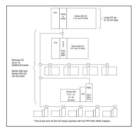
Figure 1-1 Components for the TI545/TI555 System
