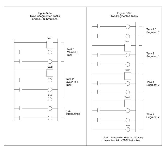
Figure 5-9 Examples of Cyclic RLL Design
