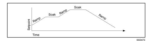
Figure 9-3 Example Ramp/Soak Cycle
