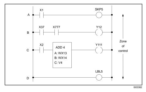
The operation of the SKP and LBL instructions is illustrated in Figure 6-82. In this example, SKP5 is located on rung A. When the SKP has power flow, the ladder logic within its zone of control, (rungs B and C) does not execute.
