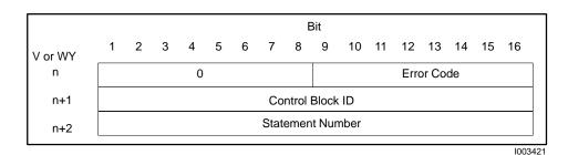
Figure 7-3 Word Specification for SF Program Errors
