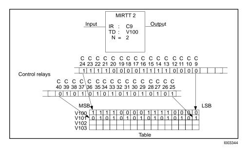
Figure 6-46 Example of MIRTT Operation
