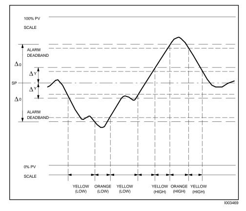
Figure 9-6 Example of Alarm Deadband For Loops
