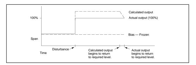
Figure 9-7 Loop Response to the Freeze Bias Option
