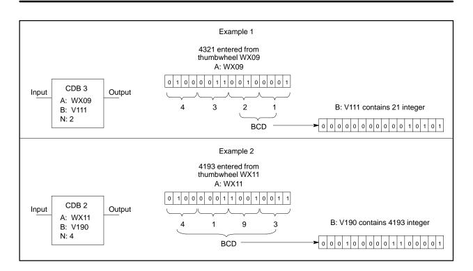
Figure 6-10 Examples of CDB Operation
