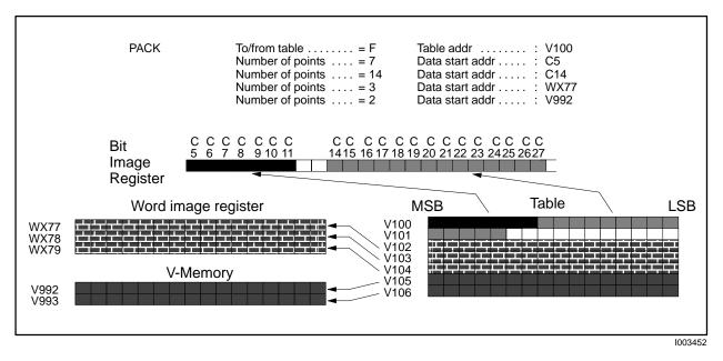
Figure 7-34 Example of PACKing Bits and Words From a Table
