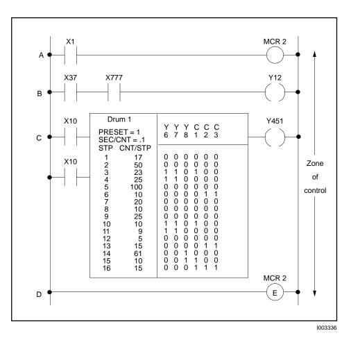
Figure 6-40 Example of the MCR Zone of Control
