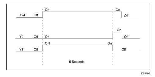
Figure E-9 Timing Diagram for TMR Application Example #2
