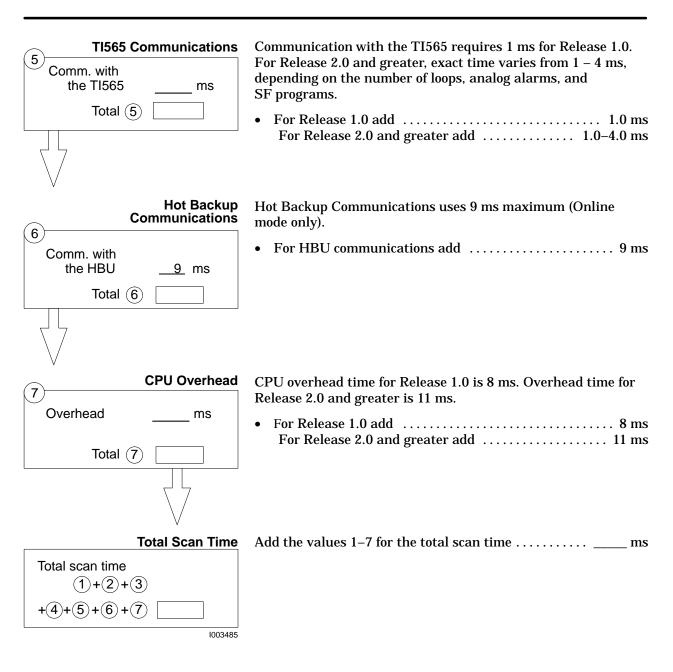
Fixing scan time to a value longer than needed only allows more processing time for the main CPU communication ports. Other functions consume only the amount of time required to execute. If the scan time is fixed at less than is required to execute all tasks, the controller uses the amount of time required to perform all tasks in the timeline and sets the "scan overrun" flag. Nothing is left out of a scan due to a fixed scan time.
