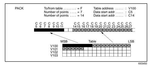
Figure 7-32 Example of PACKing Multiple Blocks of Bits From a Table
