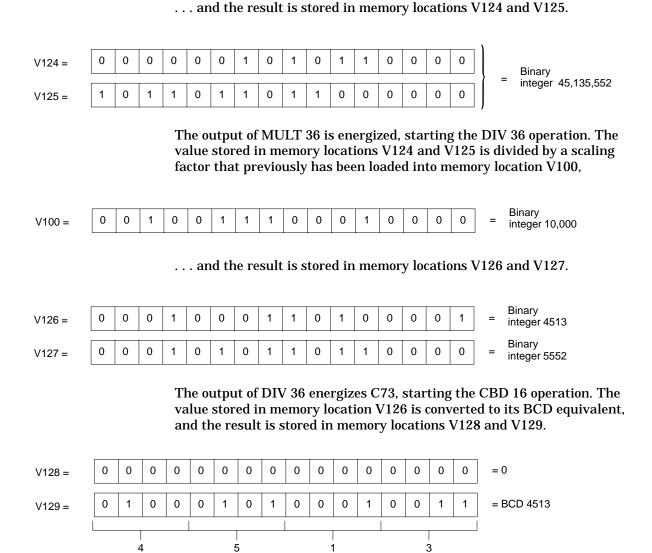
The output of CBD 16 energizes, starting the MOVW 81 operation. The value stored in memory location V129 is moved to the output IR WY65. IR WY65 outputs the BCD number to a Word Output Module located in Slot 1 of Base 1. WY65 is the first output of this module. A reading of 4.513 volts is displayed on a digital panel meter where the decimal point is fixed internally to the panel meter.
