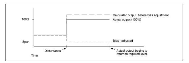
Figure 9-8 Loop Response to the Adjust Bias Option
