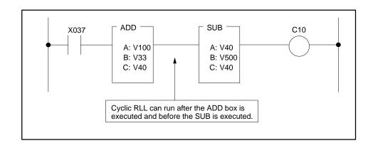
Figure 5-10 Example of Cyclic RLL Execution Interrupt
