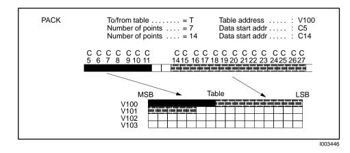
Figure 7-28 Example of PACKing Multiple Blocks of Bits Into Table
