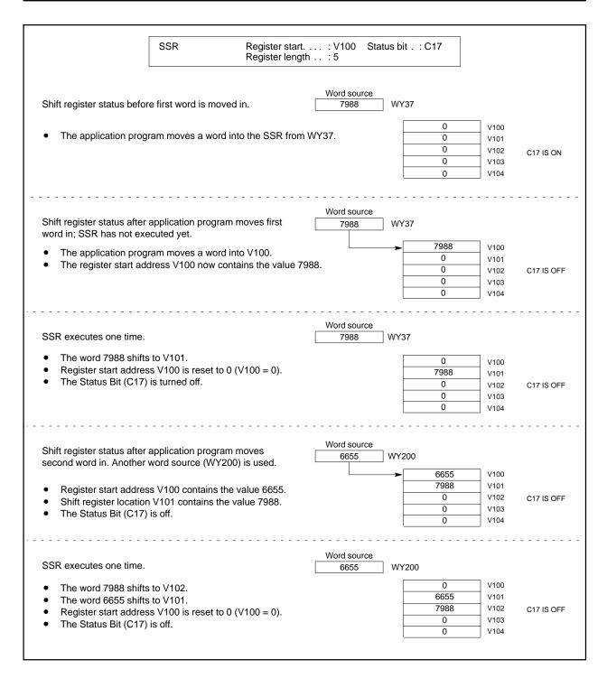
Figure 7-53 Example of SSR Operation
