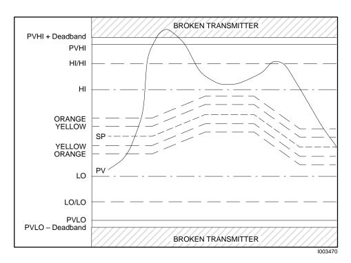
Figure 9-10 shows the process variable in broken transmitter alarm.
