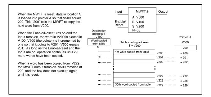
Figure 6-58 The MWFT Operation
