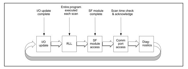
Figure 1-16 Scan Sequence for the TI520C/TI530C/TI530T Controllers
