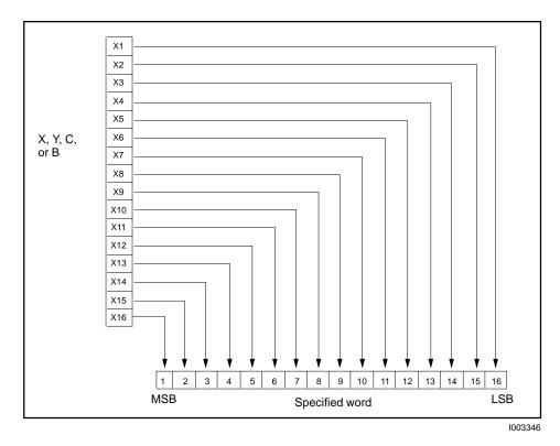
Figure 6-48 Example of MIRW Operation
