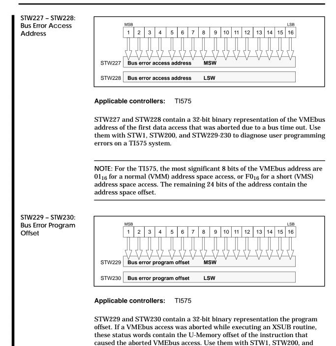
STW227-228 to diagnose user programming errors on a TI575 system.
