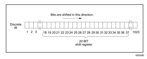
Figure E-3 20-Bit Shift Register in Discrete Image Register
