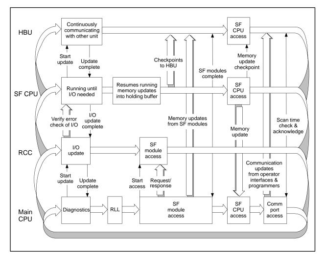
Figure 1-7 Scan Sequence for the TI565 CPU
