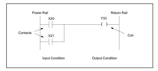
Figure 5-1 Single Rung of a Relay Ladder Logic Program
