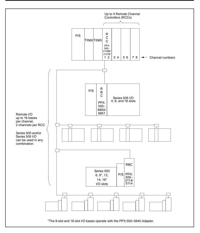
Figure 1-5 Components for the TI560/TI565 System
