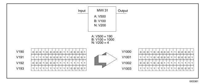
Figure 6-60 The MWI Operation
