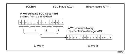
Figure 7-6 Example of BCDBIN Operation
