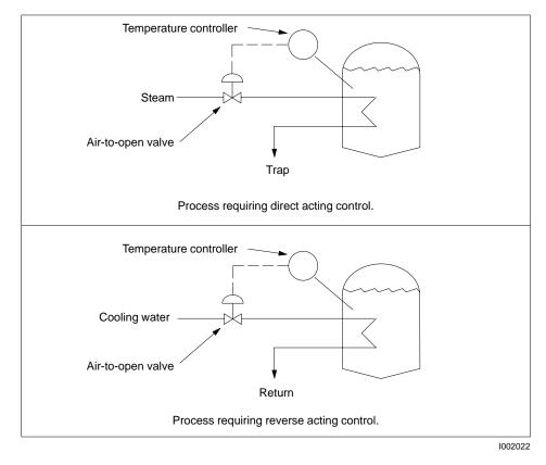
Figure 9-9 Examples of Direct- and Reverse-Acting Control
