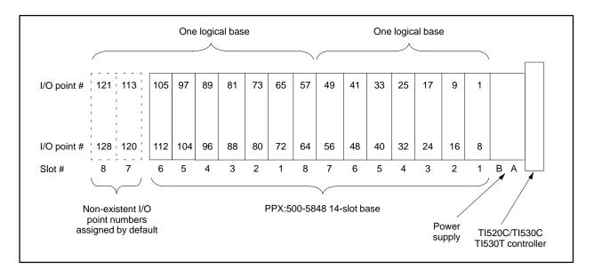
Figure 1-15 Default I/O Point Numbers for 14-Slot Base
