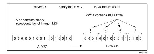
Figure 7-8 Example of BINBCD Operation
