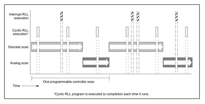
Figure 1-4 Timing Relationship of the TI545/TI555 Controller Scan Operations
