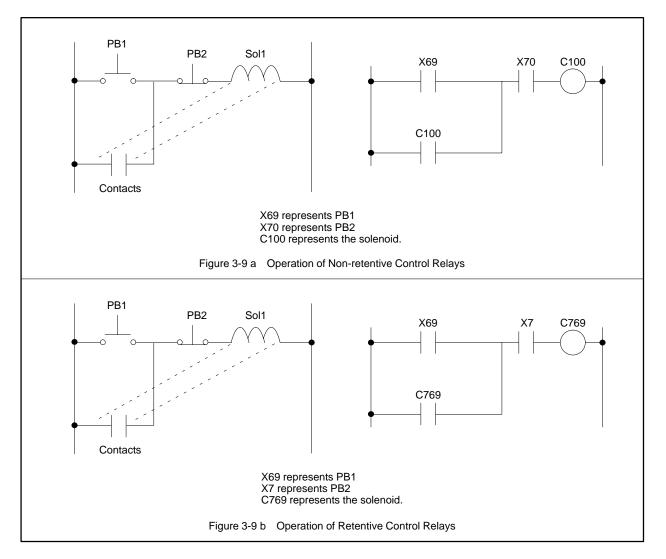
Figure 3-9 Control Relay Operation
