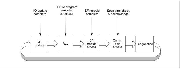
Figure 1-11 Scan Sequence for the TI525/TI535 Controllers
