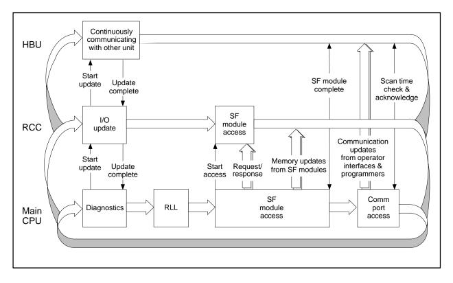
Figure 1-6 Scan Sequence for the TI560 Controller
