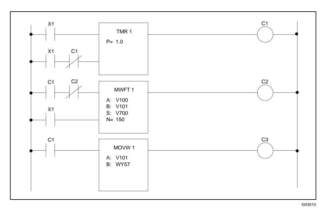
Figure E-20 RLL for MWFT Application Example
