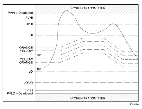
Figure 8-4 Example of Broken Transmitter Alarm
