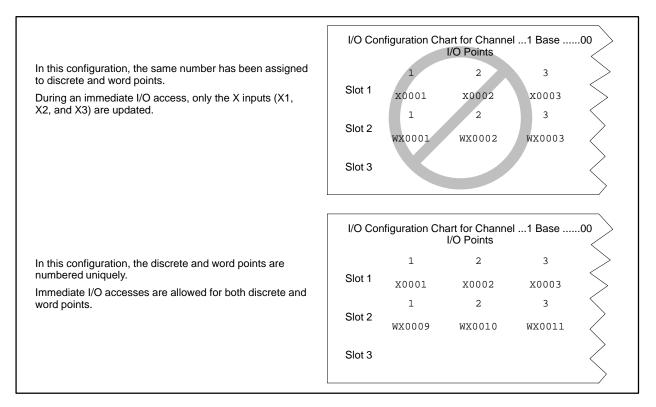
Figure 3-7 Immediate I/O Configuration Chart
