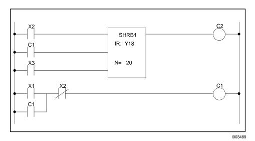
Figure E-2 RLL for SHRB Application Example
