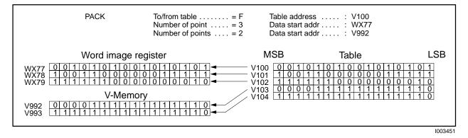
Figure 7-33 Example of PACKing Words From a Table
