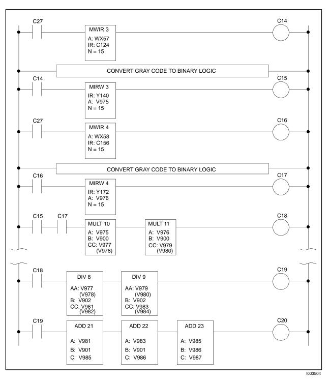
Figure E-16 RLL for MIRW Application Example
