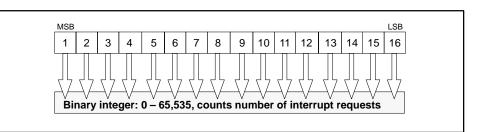
STW221 is a 16-bit integer (0 - 65,535) that is incremented each time an interrupt request is received from any interrupting module installed in the local base.
