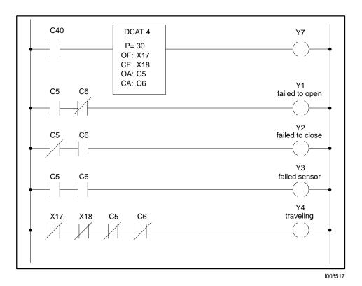
Figure E-27 RLL for DCAT Application Example
