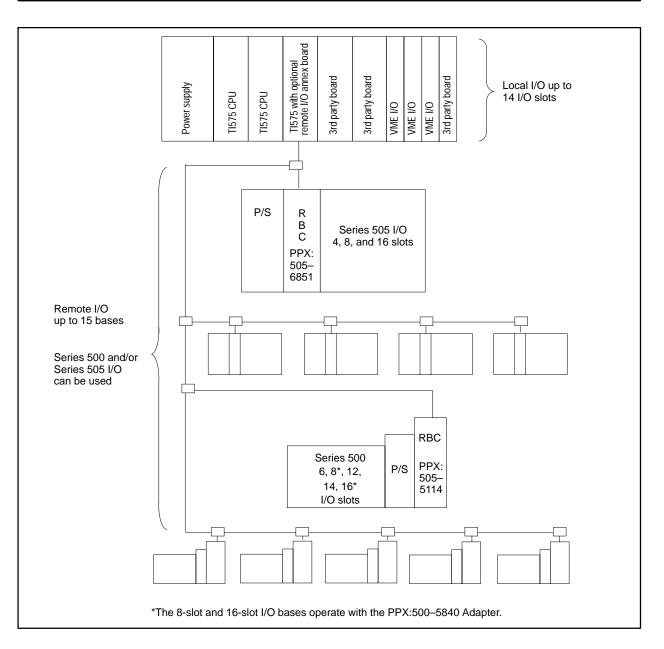
Figure 1-8 Components for the TI575 System
