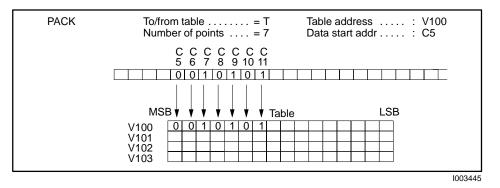
Figure 7-27 Example of PACKing Bits Into Table
