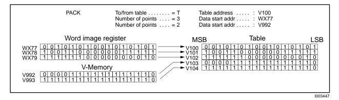
Figure 7-29 Example of PACKing Words Into Table
