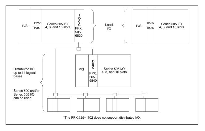
Figure 1-9 Components for the TI525 and TI535 Systems
