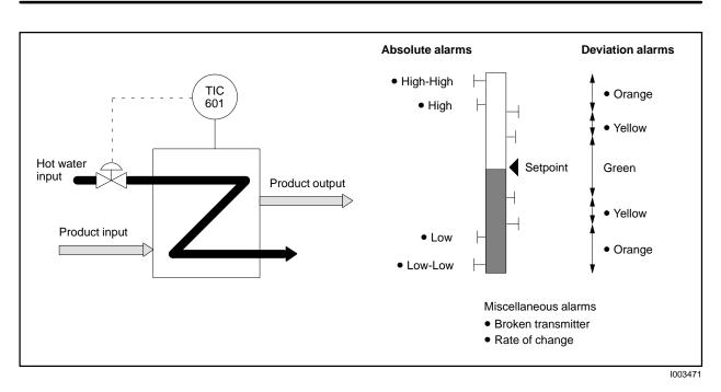
Figure 9-1 Example of Loop Control
