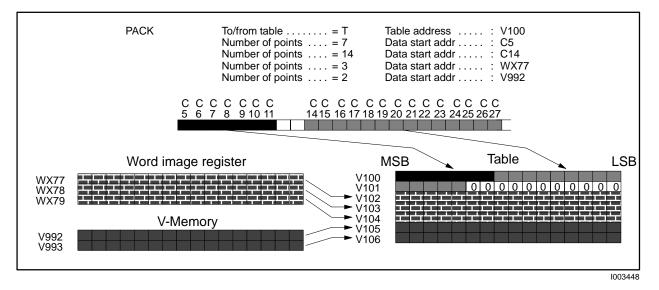
Figure 7-30 Example of PACKing Bits and Words Into Table
