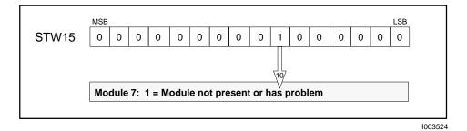
Figure G-2 Example of Status Word Reporting a Module Failure
