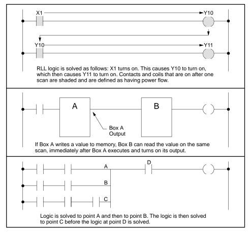
Figure 5-7 How Relay Ladder Logic is Solved
