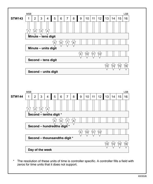
Figure G-3 illustrates how the clock information is displayed, using BCD, for a TI545 controller on the date: Monday, 5 October, 1992 at 6:39:51.767 P.M. Note that the 24-hour (military) format is used, and Sunday is assumed to be day 1.
