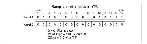
Figure 7-41 Short Form Address Example
