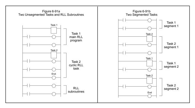
Figure 6-91 Examples of TASK Design
