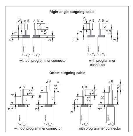
Figure 5-9 Length of stripped ends for connection to bus connector (6ES7 972-0B.20 ...)
