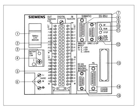
Figure 4-1 Front view of the S5-95U with DP master interface
