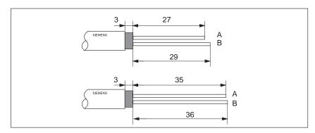
Figure 5-12 Length of stripped ends for connection to bus connector (6ES7 972-0BA30 ...)
