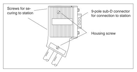
Figure 5-11 Appearance of the bus connector with order number 6ES7 972-0BA30 ...
