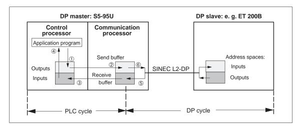
Figure 4-2 Principle of data exchange between S5-95U and DP slave
