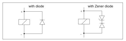
Figure 5-2 Circuits with DC-actuated coils
