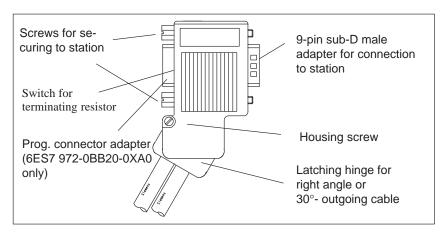
Figure 5-8 Bus connector with order number 6ES7 972-0B.20 ...
