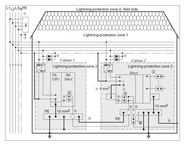
Figure E-2 Example showing lightning protection for the ET 200 distributed I/O system
