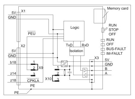
Figure 3-2 Block diagram of the IM 308-C
