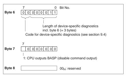
Figure 3-4 Structure of device-specific diagnostics of the IM 308-C as DP slave
