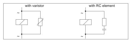
Figure 5-3 Circuits with AC-actuated coils
