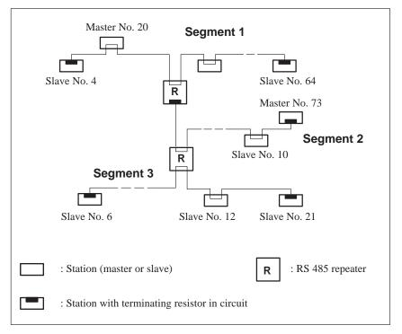
Figure 1-2 Linking bus segments with RS 485 repeaters
