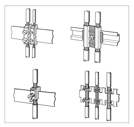
Figure 5-1 Securing shielded cables with cable clamps and cable ties (schematic diagram)
