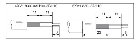
Figure 5-6 Length of stripped ends for connection to bus connector (6ES5 ...)
