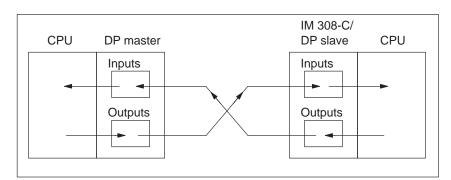
Figure 3-3 Method of operation, IM 308-C as DP slave
