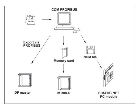
Figure 1-5 Purpose of the COM PROFIBUS parameterization software
