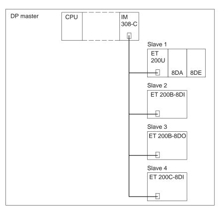
Figure C-7 Example of a bus configuration
