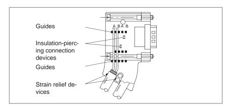
Figure 5-13 Connecting bus cable to bus connector (6ES7 972-0BA30 ...)
