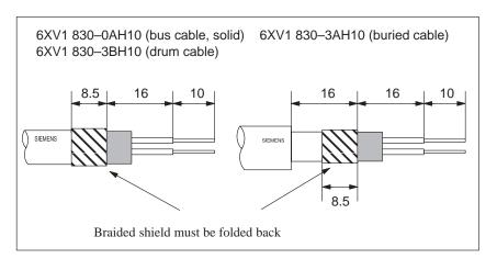
Figure 6-9 Length of stripped ends for connection to RS 485 repeater
