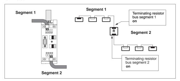
Figure 6-3 Two bus segments connected to the RS 485 repeater (1)
