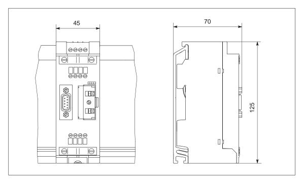
Figure F-6 RS 485 repeater on busbar for S7-300
