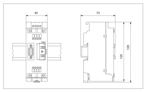
Figure F-5 RS 485 repeater on standard-section busbar
