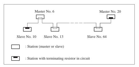
Figure 1-1 Structure of a bus segment
