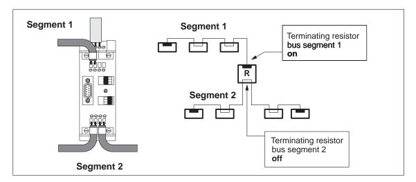
Figure 6-4 Two bus segments connected to the RS 485 repeater (2)
