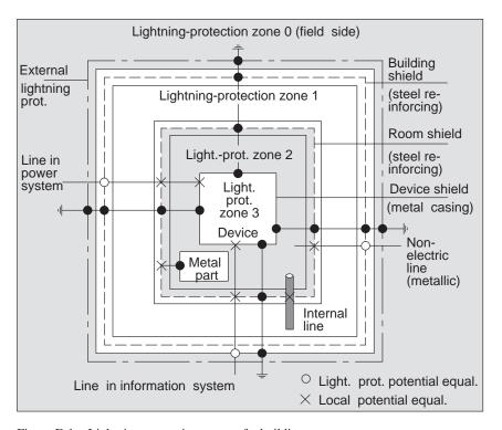
Figure E-1 Lightning-protection zones of a building
