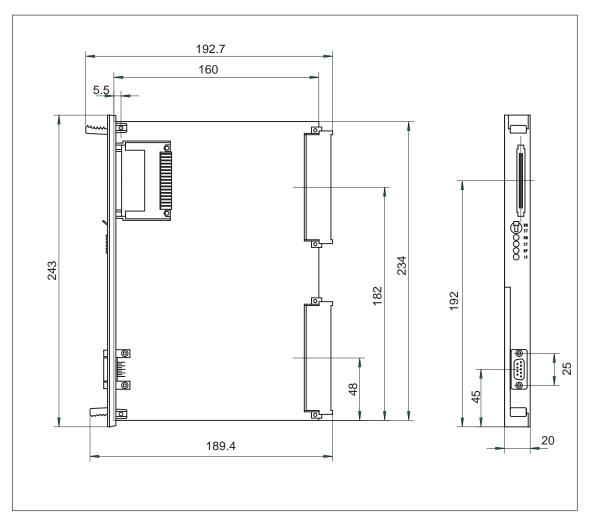
Figure F-1 Dimensional drawing of the IM 308-C master interface
