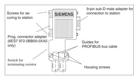
Figure 5-5 Bus connector with order number 6ES7 972-0B.10 ...
