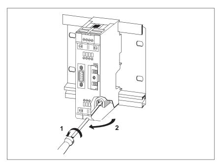
Figure 6-7 Removing the RS 485 repeater from the busbar for S7-300
