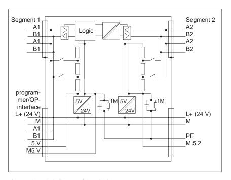
Figure 6-1 Block diagram of the RS 485 repeater
