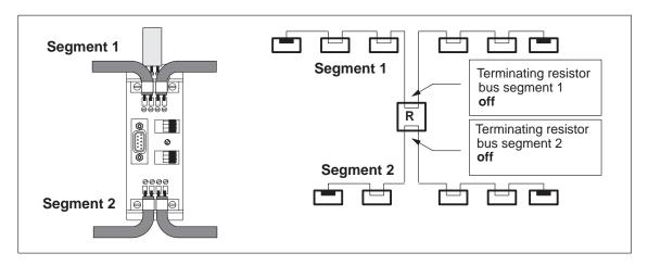
Figure 6-5 Two bus segments connected to the RS 485 repeater (3)
