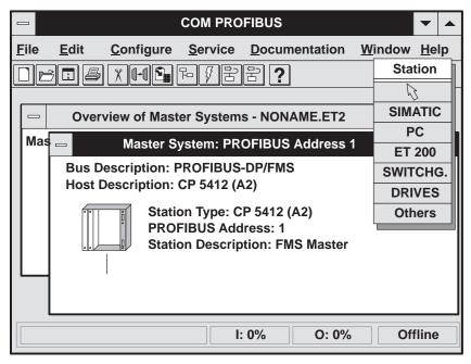
Figure 7-13 Example showing how the FMS master system is displayed on screen
