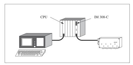
Figure 9-2 Using the FB IM308C to assign a PROFIBUS address to a DP slave
