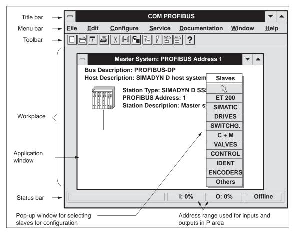
Figure 7-1 Screen elements of COM PROFIBUS
