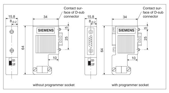
Figure F-2 IP 20 bus connector (6ES7 972-0B.10-0XA0)
