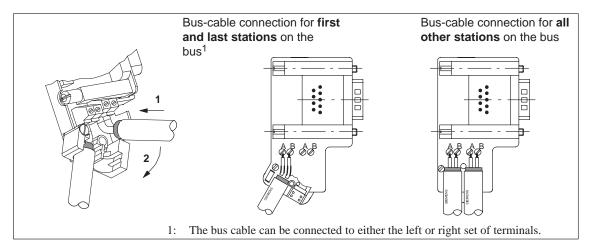
Figure 5-10 Connecting bus cable to bus connector (6ES7 972-0B.20 ...)
