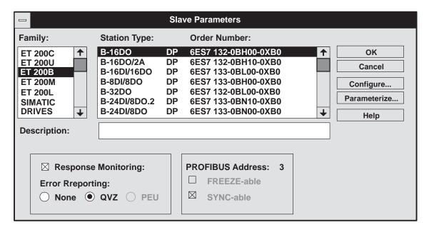
Figure 7-9 Example of the "Slave Parameters ET 200B" dialog box
