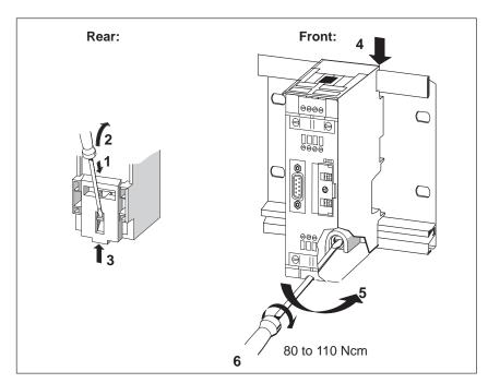
Figure 6-6 Mounting the RS 485 repeater on the busbar for S7-300
