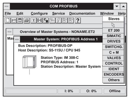
Figure 7-5 Example showing how the master system is displayed on screen
