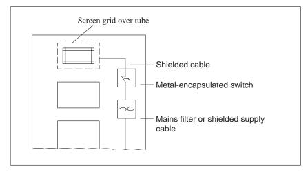
Figure 5-4 Measures for suppressing interference from fluorescent tubes in cabinets
