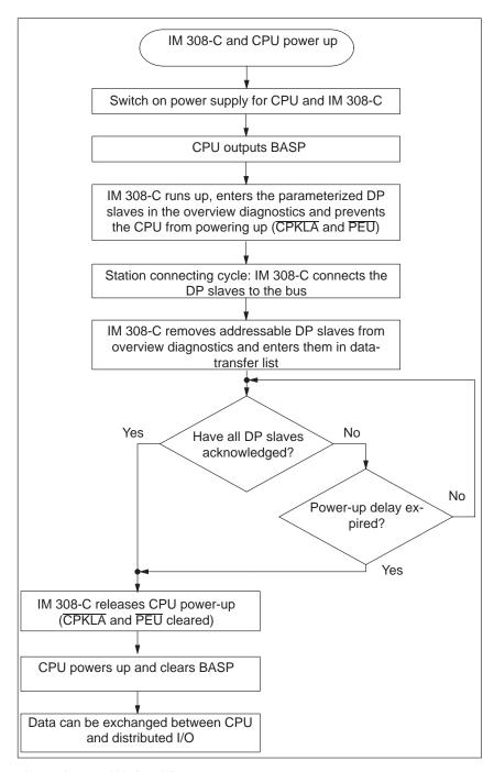
Figure 12-1 IM 308-C and CPU power-up
