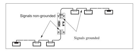
Figure 6-8 ET 200 bus segments operating as non-grounded segments
