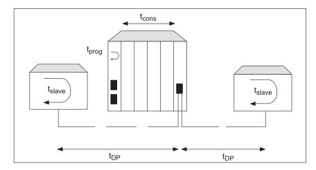
Figure C-1 Reaction times in the ET 200 distributed I/O system
