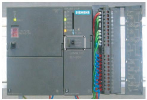
Figure 5-5 Successful wiring, CPU in position STOP
