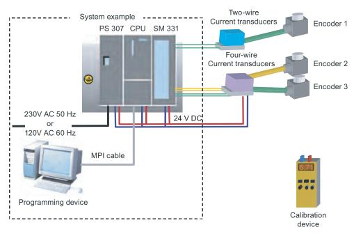
Figure 3-1 Sample station components
