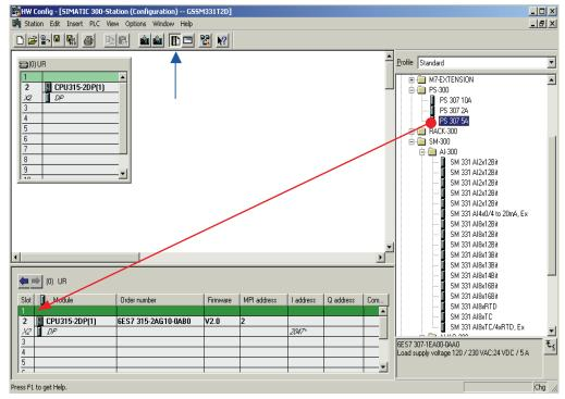
Figure 6-8 Hardware configuration: Basic configuration
