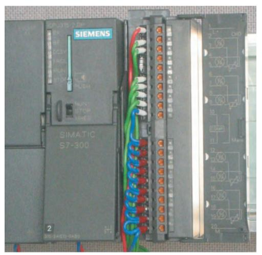
Figure 5-4 SM331 Front connector wiring
