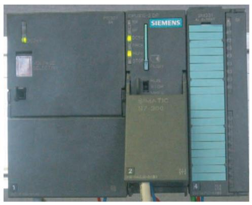
Figure 6-13 CPU in error free state
