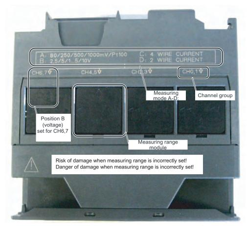
Figure 4-2 4 measuring range modules with default setting B (Voltage)
