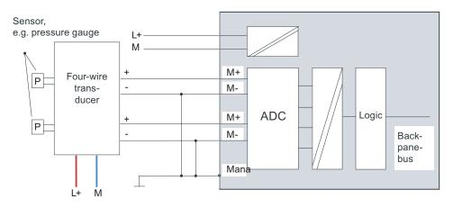
Figure 5-3 Wiring: 4-Wire current transducer
