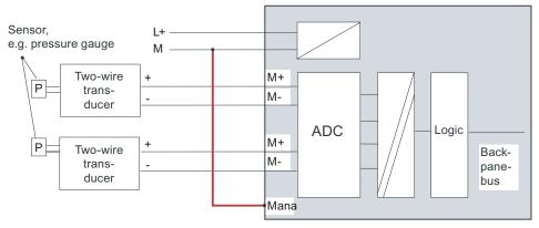
Figure 5-2 Wiring: 2-Wire current transducer
