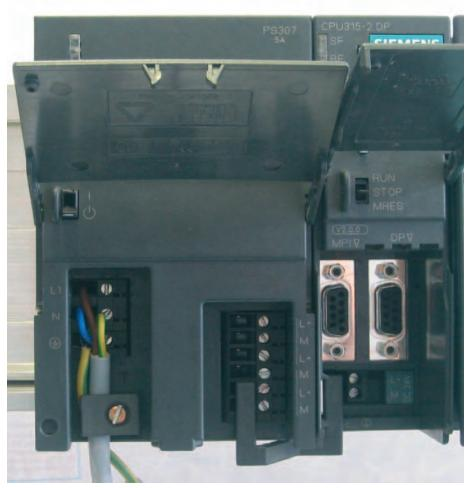
Figure 5-1 Wiring the power supply module and the CPU
