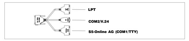
The I Cable enables the connection to S5 automation devices (COM1/TTY), to devices with a serial port (COM2/standard V.24) such as a modem or mouse and to devices with a parallel port (standard LPT) such as a printer or scanner. Please, use the I Cable on a level surface only (e.g. desk) to prevent contact problems. *Refer to Chapter 3.6 of the electronic manual.*
