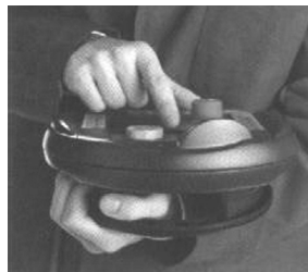
Figure 4-1 Lower arm support for right and left-handed users in Manual Mode
