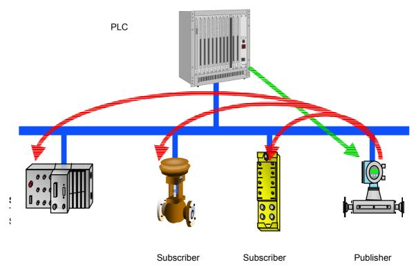
Figure 4.1: Principle of Data Exchange Broadcast
