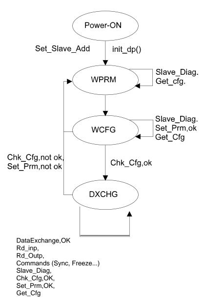
The sequence in principle of this state machine is helpful in understanding the firmware sequence. Details are found in the Standard.
