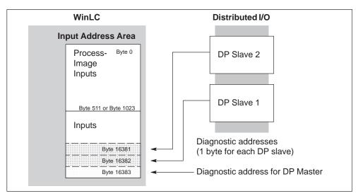
Figure 6-6 Diagnostic Addresses for the Distributed I/O
