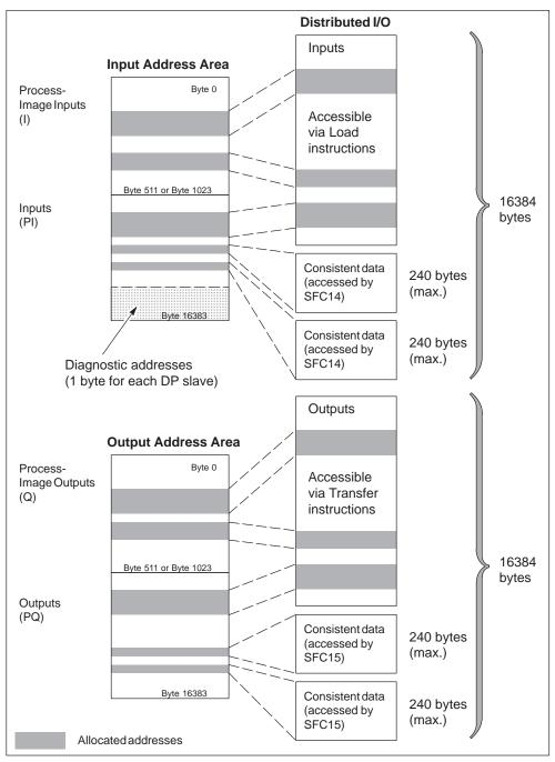
Figure 6-5 Accessing the Distributed I/O
