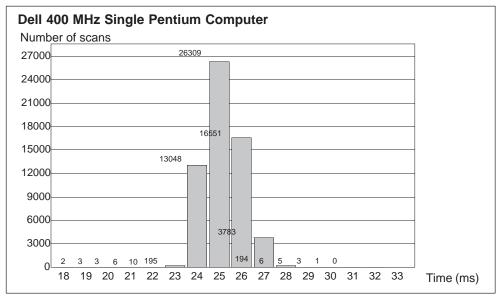
Figure B-1 Sample Jitter for the Dell 400 MHz Single Pentium Computer
