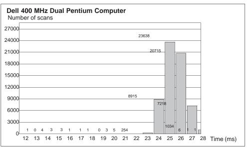
Figure B-3 Sample Jitter for the Dell 400 MHz Dual Pentium Computer
