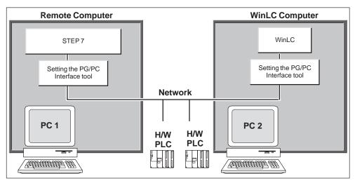
Figure 3-2 Connecting STEP 7 to WinLC over a network
