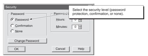
Figure 4-20 Setting the Security Level for WinLC
