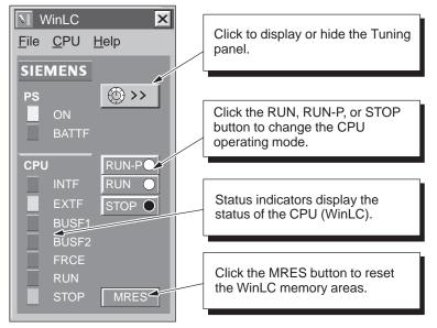
Figure 4-7 Using the CPU Panel of WinLC
