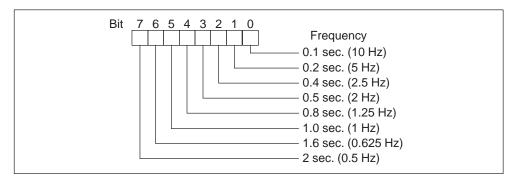
Figure 5-3 Clock Frequencies for the Memory Byte Configured as Clock Memory
