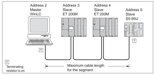
Figure 6-3 Maximum Cable Length for a Segment
