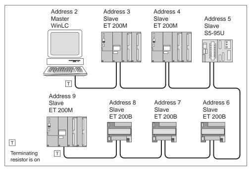
Figure 6-2 Typical Addresses for a PROFIBUS-DP Network
