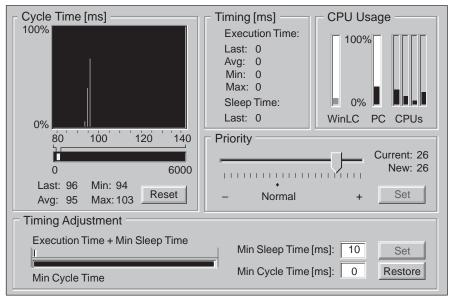
Figure 4-11 Tuning Panel for Adjusting the Operation of WinLC
