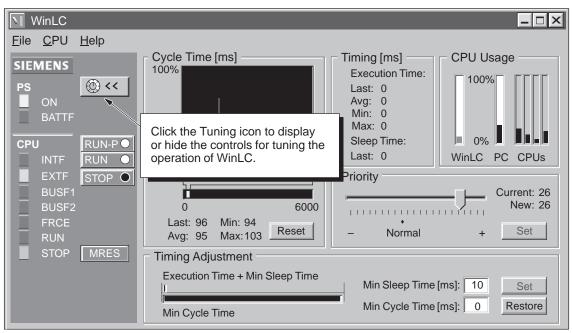
Figure 4-12 Displaying or Hiding the Tuning Panel of WinLC
