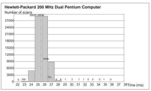
Figure B-2 Sample Jitter for the Hewlett–Packard 200 MHz Dual Pentium Computer
