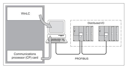
Figure 2-1 Installing the Components for WinLC
