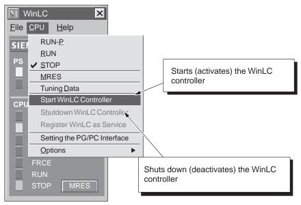
Figure 4-14 Shutting Down the WinLC Controller
