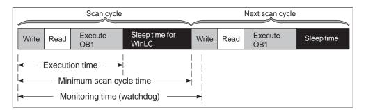
Figure 4-10 Elements of the WinLC Scan Cycle
