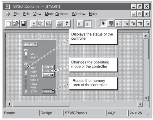
Figure C-1 Buttons and Indicators on the Panel Control
