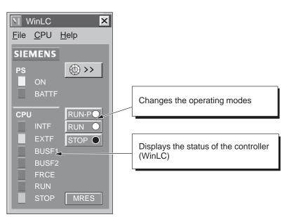
Figure 5-1 Mode Selector Buttons and Status Indicators of the CPU Panel
