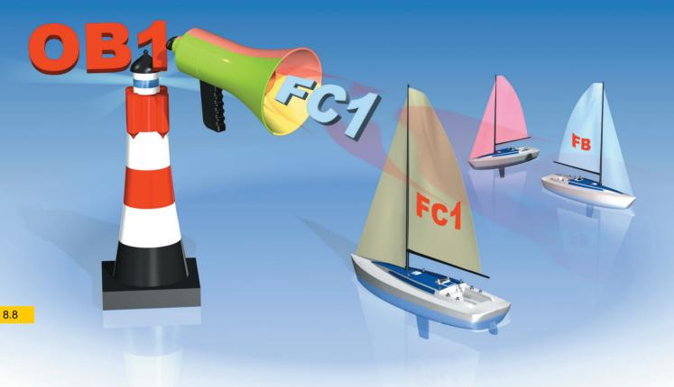
FC1 is called in OB1 in the same way as a function block. For function parameters OB1 provides corresponding address data for the petrol or Diesel engine.
