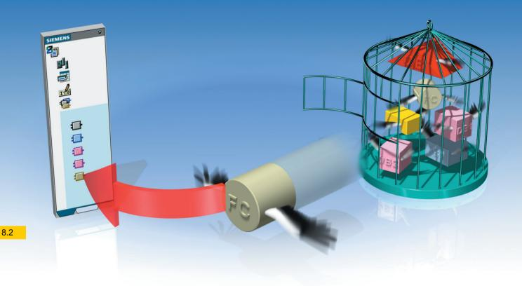
Functions are used if FC programming does not require of you to save intermediate results, mode settings or operating modes until the next block call. This is why they are also referred to as "Blocks without memory".
