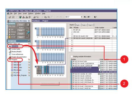
During hardware configuration you develop an image of the PLC station on your programming device. You can copy this configuration to other STEP 7 Lite projects and, if required, modify and download it to other existing stations. During the PLC startup routine, the CPU compares the default configuration created in STEP 7 Lite with the actual configuration of the system. This way any existing errors can then be detected and reported immediately.
