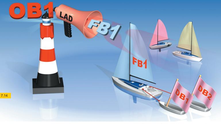
The entire function block program will be ineffective unless it is called in OB1. To control both engines, one DB is used per FB call.
