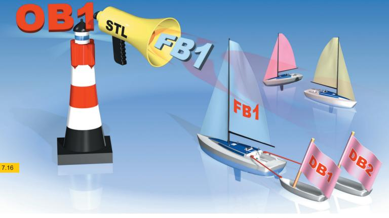
A function block program will be ineffective unless it is called in OB1. To control both engines, one DB is used per FB call.
