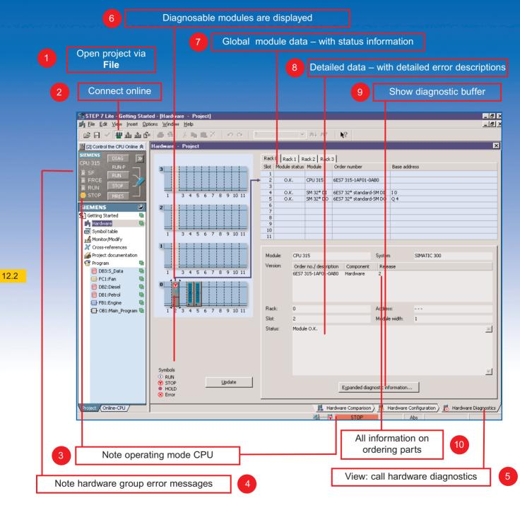
STEP 7 Lite offers extensive error diagnostics at a glance after a hardware error has occurred in the PLC station. The code number will indicate the diagnostics path. This view is only available in online mode.
