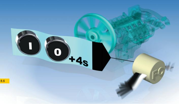
In our next example you are going to program a timer function. When the timer is switched, the timer function simutaneously switches on a fan which runs for 4 seconds after the engine has been switched off (off delay)
