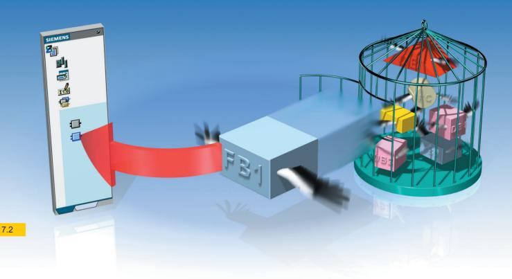
Function blocks are used in function programming if you have to save intermediate results or operating settings and operating modes until the next call. For this reason, they are also referred to as "Blocks with memory".
