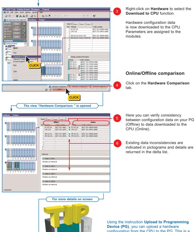
**Device (PG)**, you can upload a hardware configuration from the CPU to the PG. This is a typical service action if you want to access a switching cabinet with a PG in order to analyze an error.
