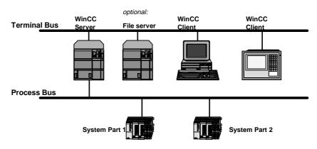
A **WinCC server** always has one physical connection to the PLCs (point-to-point or process network). In addition, the server has a network connection to the assigned WinCC clients.
