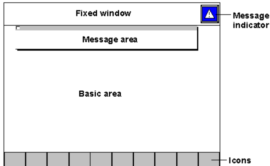
Example of partitioning the display on the SIMATIC Panel PC
