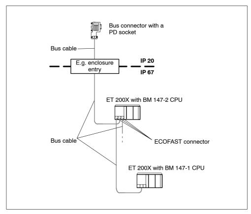
Figure 3-5 Connecting the DP network
