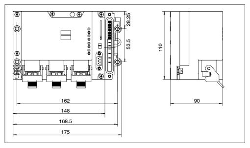
Figure 9-2 Dimensioned drawing of basic module BM 147 CPU (BM 147-2 CPU is shown)
