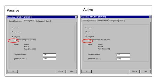
Figure 3-2 Setting the mode of the DP interface at the BM 147 CPU
