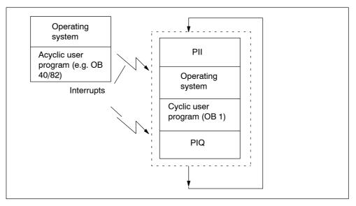
Figure 8-1 Component parts of the cycle time
