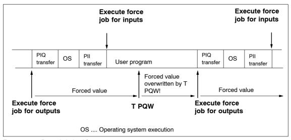
Figure 3-6 Principle behind forcing
