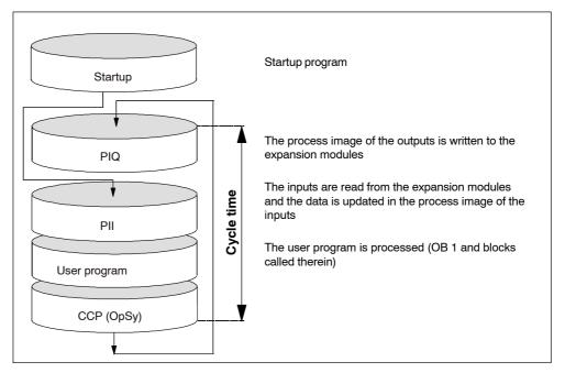
Figure 7-5 Processing steps within a cycle
