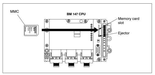
Figure 7-2 Position of the memory card slot for the MMC on the BM 147 CPU
