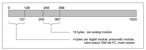
Figure 2-2 Structure of the default address area
