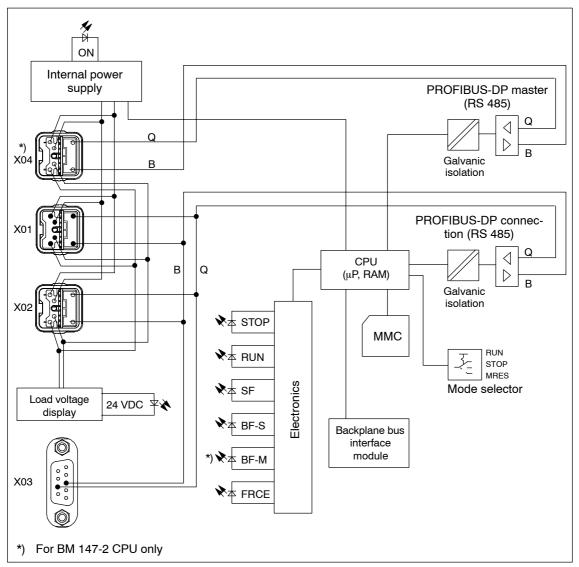
Figure 9-1 Block diagram BM 147 CPU
