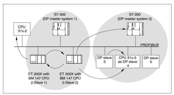
Figure 3-7 Direct communication with the BM 147 CPU
