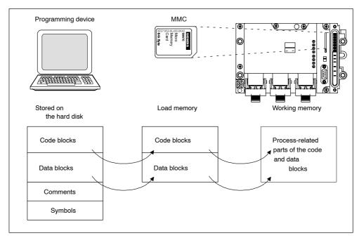
Figure 7-4 Load and working memory
