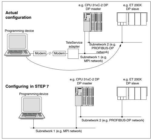
Figure 7-9 Routing – TeleService application example
