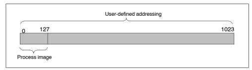
Figure 2-5 Structure of the address area for user-oriented addressing
