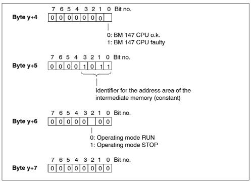
Figure 6-8 Byte y+4 to y+7 for the diagnostic interrupt (changed operating status of the intelligent slave)
