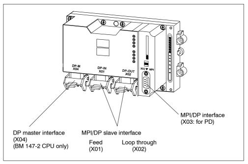
Figure 5-2 Interfaces on basic module BM 147 CPU
