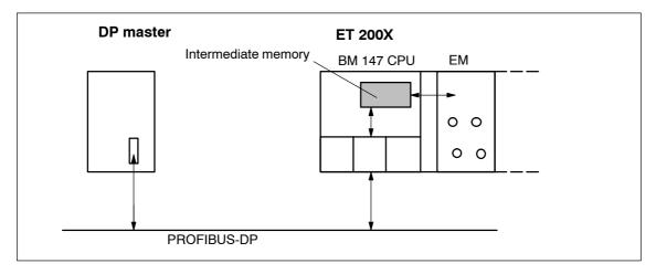
Figure 2-6 Intermediate memory in the BM 147 CPU
