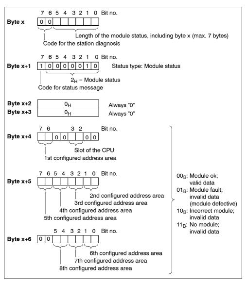
Figure 6-6 Structure of the module status
