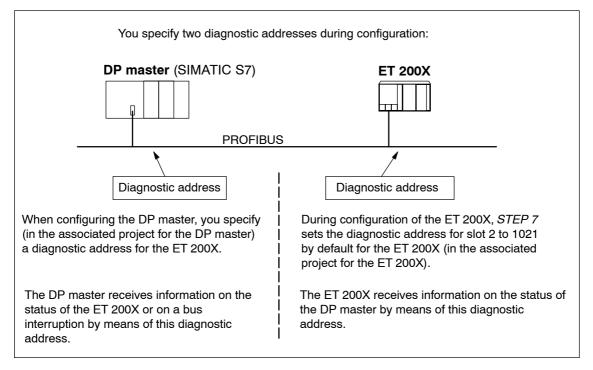
Figure 6-3 Diagnostic addresses for the DP master and ET 200X
