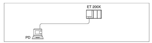
Figure 3-4 The PD directly accesses the ET 200X
