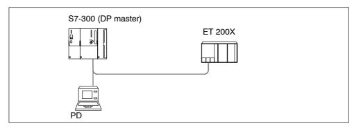
Figure 3-3 PD/OP accesses the ET 200X via the DP interface in the DP master
