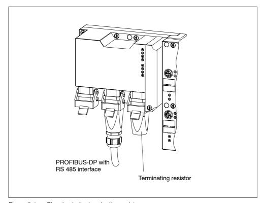
Figure 5-4 Plugging in the terminating resistor
