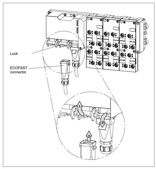
Figure 5-3 Plugging the connector into the BM 147 CPU
