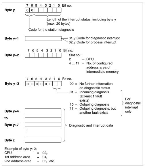
Figure 6-7 Structure of the interrupt status
