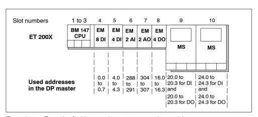
Figure 2-4 Example of address assignment to expansion modules
