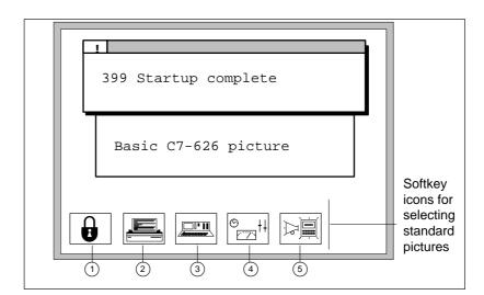
Figure 2-13 Basic C7 Picture (Example)
