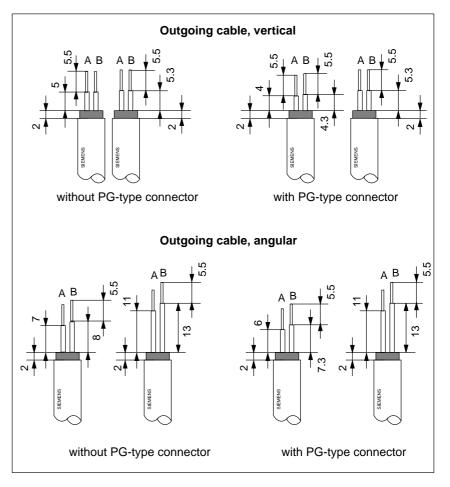
Figure 3-14 Length of Stripped Insulation for Connecting to the Bus Connector 6ES7 972-0B.20 ...
