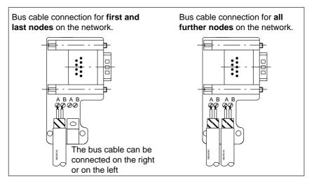
Figure 3-17 Connecting the Bus Cable to the Bus Connector (6ES7 972-0B.10-0XA0)
