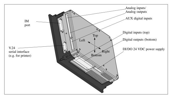
Figure 2-8 A View of the C7 with External I/O Interfaces
