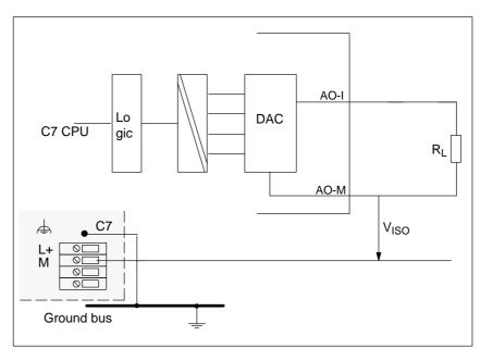
Figure 6-5 Connecting Loads to a Current Output of an Isolated Analog Output Module
