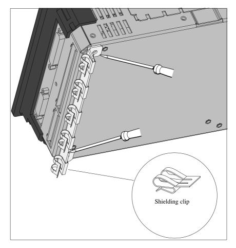
Figure 2-10 C7 with Grounding Bar and Shielding Clips
