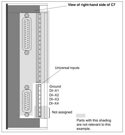
Figure 7-1 Pin Assignments of the Universal Inputs
