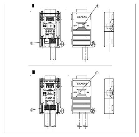
Figure 3-11 PROFIBUS Bus Connector
