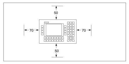
Figure 2-7 Gap Dimensions to be Observed when Installing the C7
