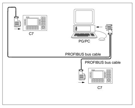
Figure 4-2 Connecting a Programming Device to Several C7s
