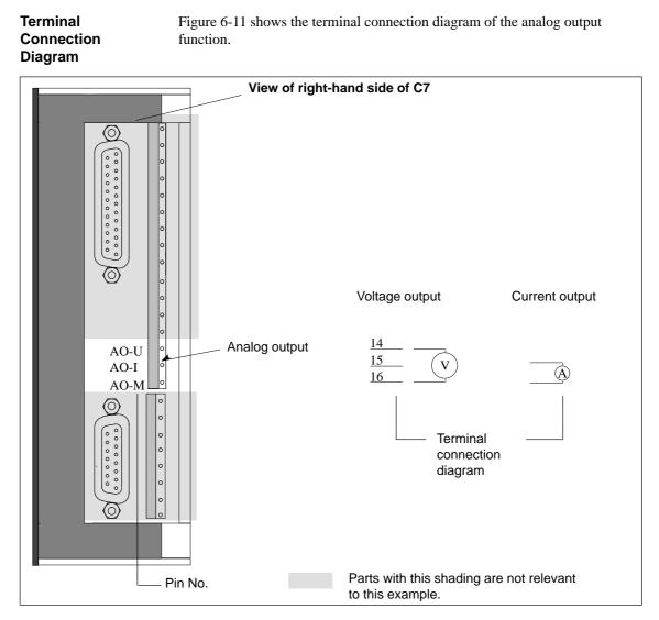
Figure 6-11 Terminal Connection Diagram of the Analog Output Function
