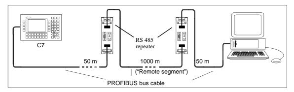
Figure 3-8 Maximum Cable Length Between Two RS 485 Repeaters
