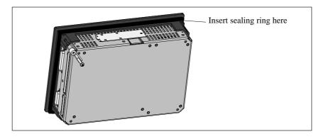
Figure 2-2 Inserting the Sealing Ring
