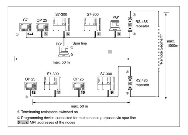
Figure 3-9 Cable Lengths in an MPI Network
