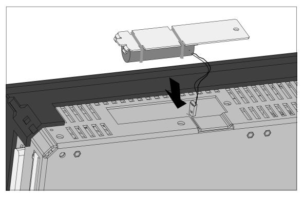
Figure 8-3 Inserting the Back-Up Battery
