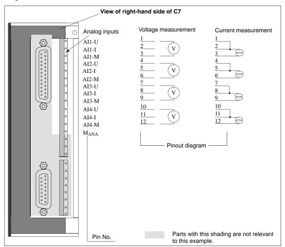
Terminal Connection Diagram Figure 6-7 shows the terminal connection diagram of the analog inputs.
