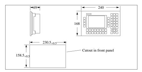
Figure 2-3 Dimensions for the C7
