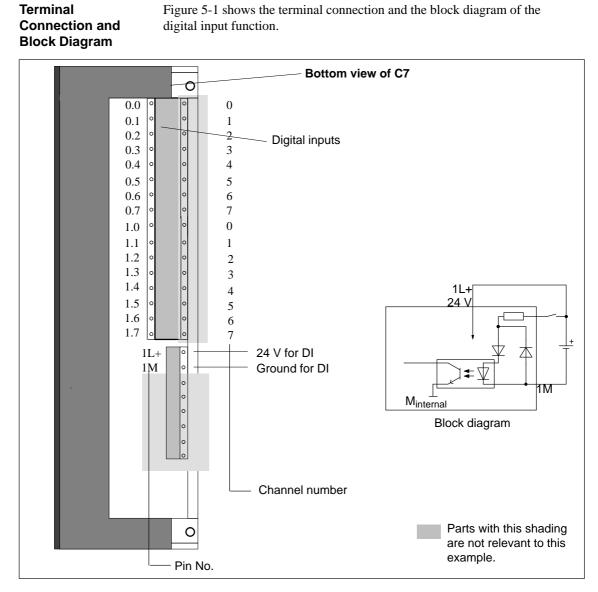
Figure 5-1 Terminal Connection and Block Diagram of the Digital Input Function
