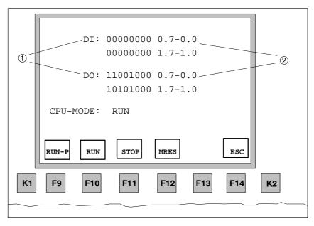
Figure 5-3 DI/DO Status Bits in a C7
