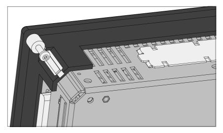
Figure 2-5 Fixing Bracket Engaged, with Screw
