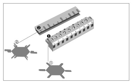
Figure 2-11 How to Key Connectors
