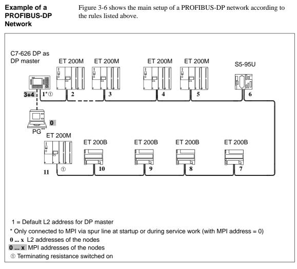
Figure 3-6 Example of a PROFIBUS-DP Network
