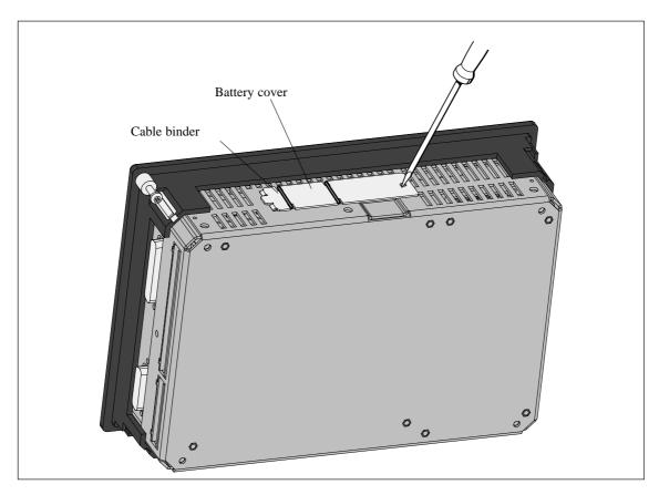
Figure 8-1 Battery Cover Before Opening
