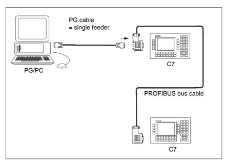
Figure 4-3 Connecting a Programming Device/PC to an MPI Network
