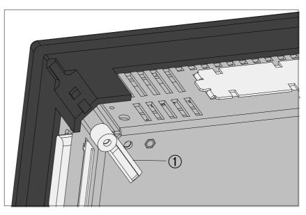
Figure 2-4 Fixing Bracket Before Engaging
