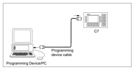
Figure 4-1 Connecting a Programming Device/PC to a C7
