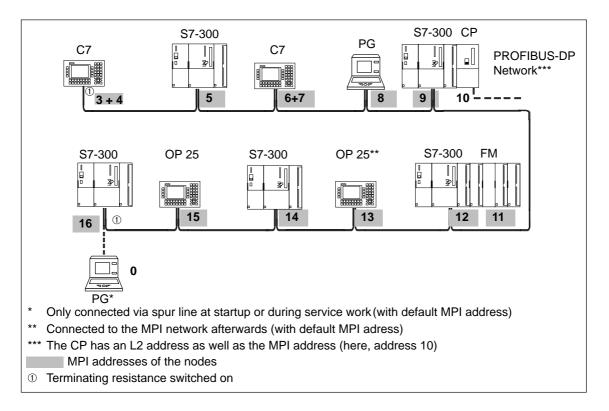
Figure 3-5 Example of an MPI Network
