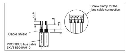
Figure 3-12 Connecting the PROFIBUS Bus Cable to the Screw-Type Terminal Block
