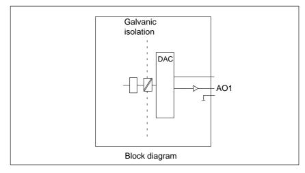
Figure 6-12 Block Diagram of the Analog Output Function
