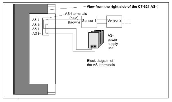
Figure 5-1 Connections and Block Diagram of the AS-i Terminals
