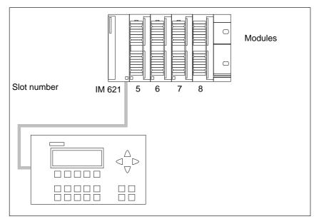
Figure 2-15 Maximum Configuration for a C7-621 AS-i
