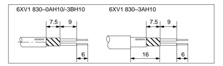
Figure 3-12 Preparing the LAN Cable for Connecting the Bus Connector 6ES7 972-0B.10-0XA0
