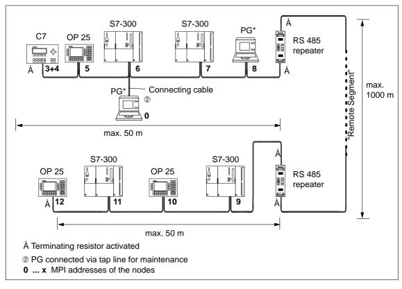
Figure 3-6 Cable Lengths in an MPI Network
