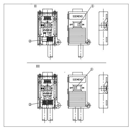
Figure 3-7 Appearance of the PROFIBUS Bus Connector
