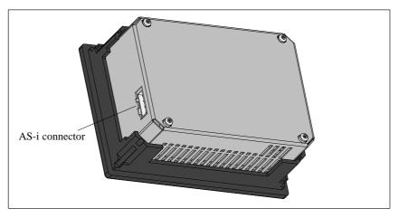
Figure 2-10 C7-621 AS-i with AS-i Connector
