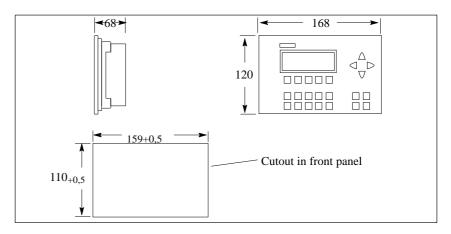
Figure 2-2 Dimension Drawings for the C7
