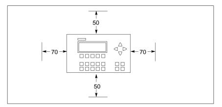
Figure 2-6 Minimum Clearances when Installing the C7
