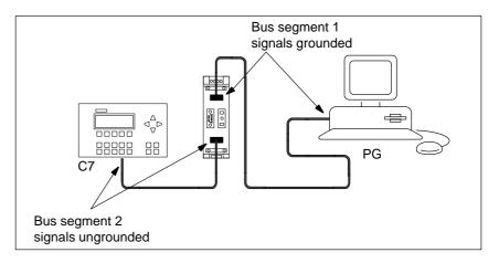
Figure 4-4 PG Connected to an Ungrounded S7-300
