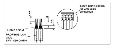
Figure 3-8 Connecting the PROFIBUS LAN Cable to the Screw Terminal Block
