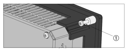
Figure 2-4 Securing Post Engaged, with Screw
