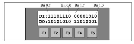
Figure 6-3 Example of a Status Display on a C7-621
