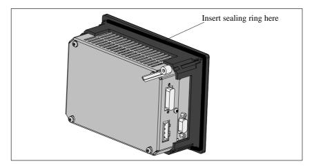
Figure 2-1 Inserting the Sealing Ring
