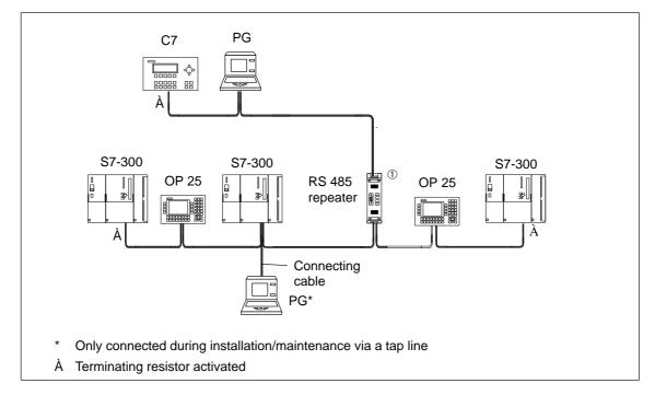
Figure 3-3 Activating Terminating Resistors in an MPI Network
