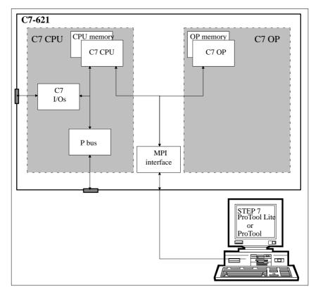
Figure 1-3 Components of the C7-621
