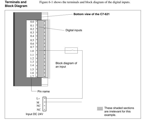
Figure 6-1 Terminals and Block Diagram of the Digital Inputs
