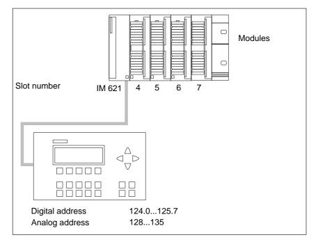
Figure 2-14 Maximum Configuration with a C7-621
