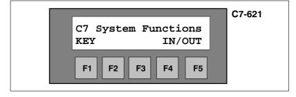
Figure 2-16 C7-621 System Functions Menu with Function Keys
