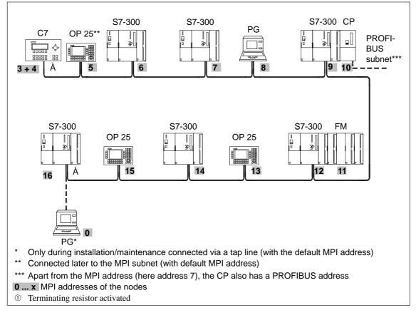
Figure 3-4 Example of an MPI Subnet
