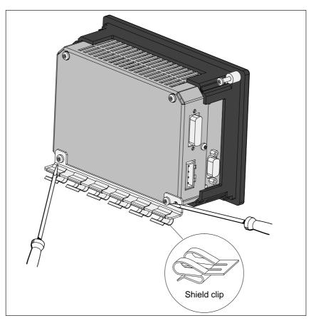
Figure 2-11 C7-621 with Grounding Bar and Shield Clips
