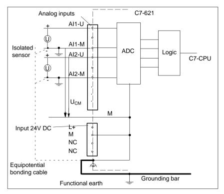
Figure 7-2 shows the connection of non-isolated sensors to a floating analog input module.
