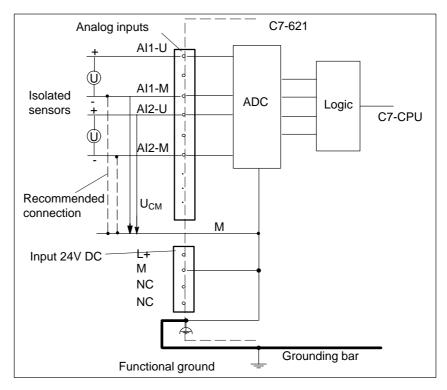
Figure 7-1 shows the connection of isolated sensors to a non-floating analog input.
