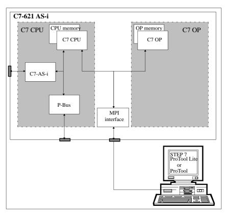
Figure 1-4 Components of the C7-621 AS-i
