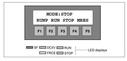
Figure 2-18 "C7 CPU Modes" Menu with Function Keys
