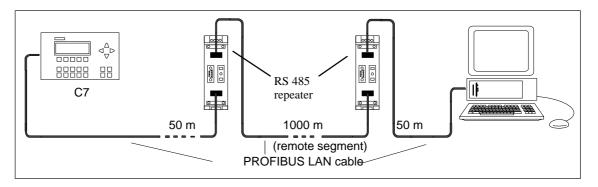
Figure 3-5 Maximum Cable Length Between Two RS 485 Repeaters
