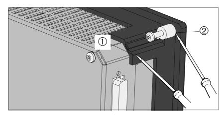
Figure 2-5 Removing the Securing Post
