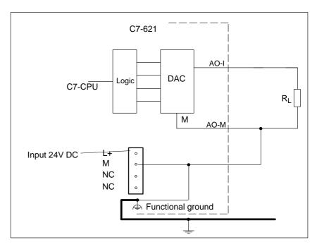
Figure 7-5 Connecting Loads to a Current Output of a Non-Floating Analog Output
