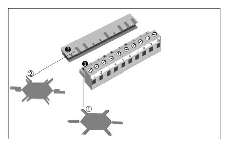
Figure 2-12 Preventing Insertion of the Wrong Connector
